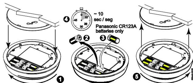
**CAUTION:** The batteries used in this device may present a fire or chemical burn hazard if mistreated. Do not recharge, disassemble, heat above 100°C (212°F) or dispose of in fire. Use only Panasonic CR123A Lithium batteries. Use of other batteries may present a risk of fire or explosion. Keep used batteries away from children. Dispose of used batteries properly.
