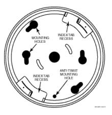
3. Secure the sensor to the mounting base by aligning the sensor's index tabs to the index tab recesses on the mounting base. While pushing in, turn the sensor clockwise until it locks. DO NOT touch the metal
