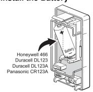
BATTERY CAUTION: Risk of fire, explosion, and burns. Do not recharge, disassemble, heat above 212 °F (100 °C), or incinerate. Dispose of used batteries properly. Keep away from children.
