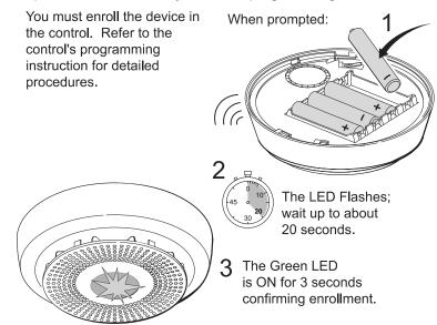
The device can also be manually enrolled. See the Controller's Programming Guide for details.
