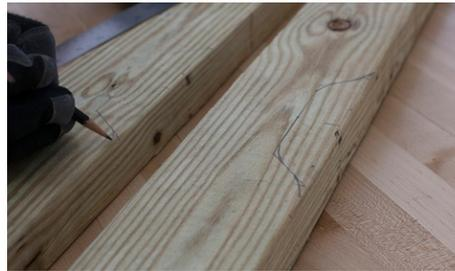
We'll begin with the handle cutout, found on one side of the board set. First, draw the 4" x 6" outline and ease a curve based on the diagram provided on Page 3.
