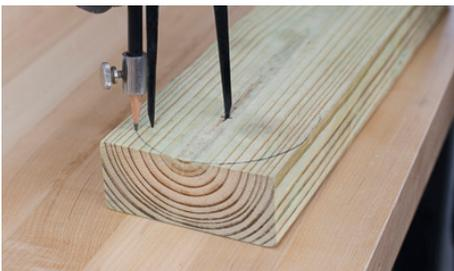
Using a compass, draw a semi-circle with a 1 3/4" radius.
