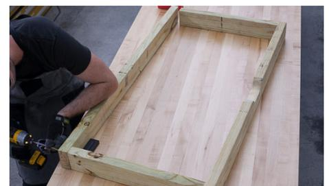
Use two 2 1/2" wood screws at each corner to attach the boards to each other.
