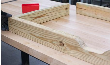
**Tip:** Direct-measure your board stock's width and use half of this number in place of the 1 3/4" for a more precise mid-point. 1 3/4" is based on a 3 1/2"-width 2x4.
