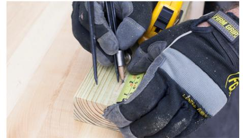
At the top of part (C), mark a point that is 1 3/4" from the top and 1 3/4" from the edges. This is the center of the circle.
