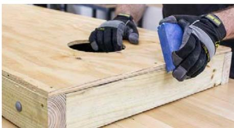
Ease any sharp edges with a medium-grit sanding block. Apply preferred finish to the wood.
