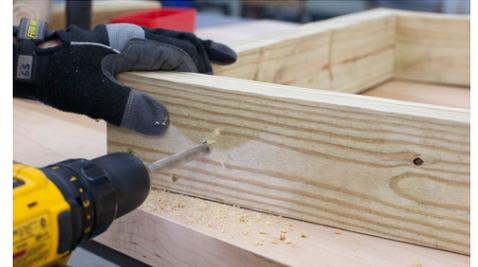
Using a 3/8" drill bit, make a hole at this point.
