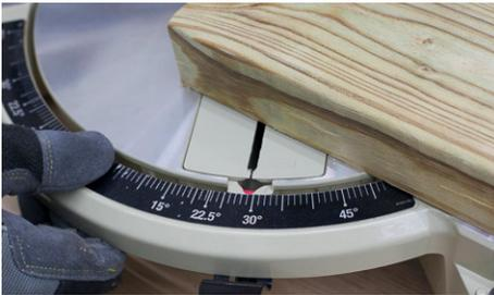
At the bottom of part (C), mark a line at a 29° angle from one of the corners. You can also use a compound miter saw to dial in to 29° if you have one.
