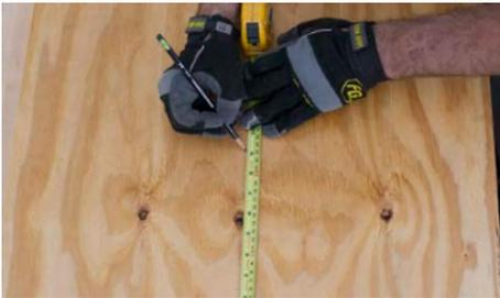
On part (E), mark a point that is 12" from the left and right edges and 9" from the top edge.
