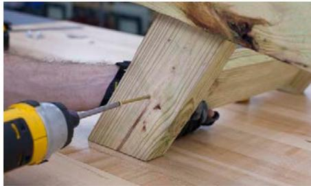
Use two 2 1/2" wood screws at each end to attach part (D) to parts (C).
