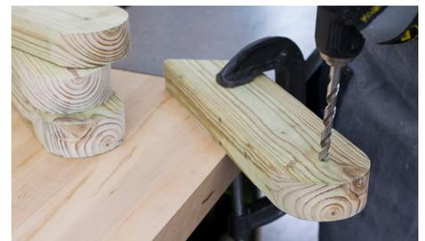
Using a 3/8" drill bit, make a hole at the center of the circle you marked.
