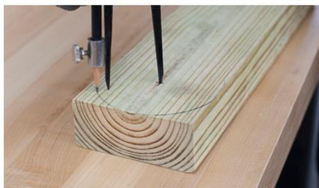
Using a compass, draw a semi-circle with a 1 3/4" radius.
