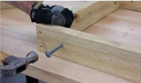
Connect part (C) to part (A) with a 3/8" carriage bolt. Use a hammer if needed.
