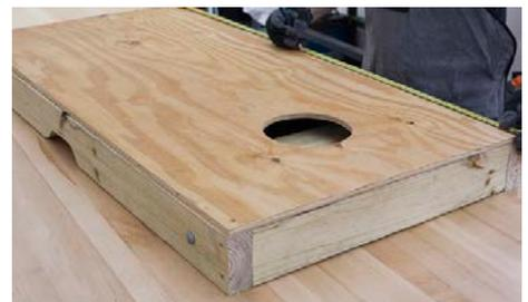
Attach at the four corners using 1 1/2" wood screws. Then use screws at 12-inch intervals along the perimeter of the board.
