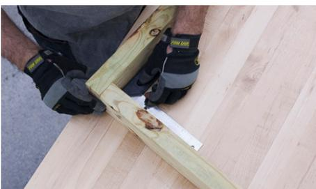
To make the frame, arrange parts (A) and (B) on a flat surface in a rectangle as shown. Keep the edges flush and the angles at 90 degrees (use a square to ensure right angles).
