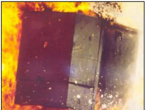
well before a circuit breaker or recloser can clear the circuit. Equipment not containing oil may still explode and evolve huge volumes of smoke and toxic gases. This may be spread through the ventilation systems of a major office complex.
