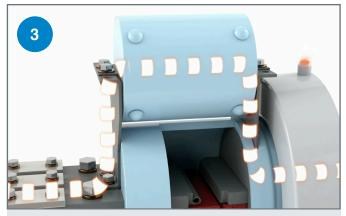
The resultant arc voltage across this gap causes a transfer of the short-circuit current to a small, parallel current-limiting fuse.
