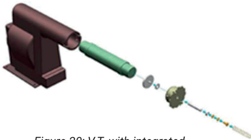
Figure 20: V.T. with integrated fuse-holder (exploded view)
