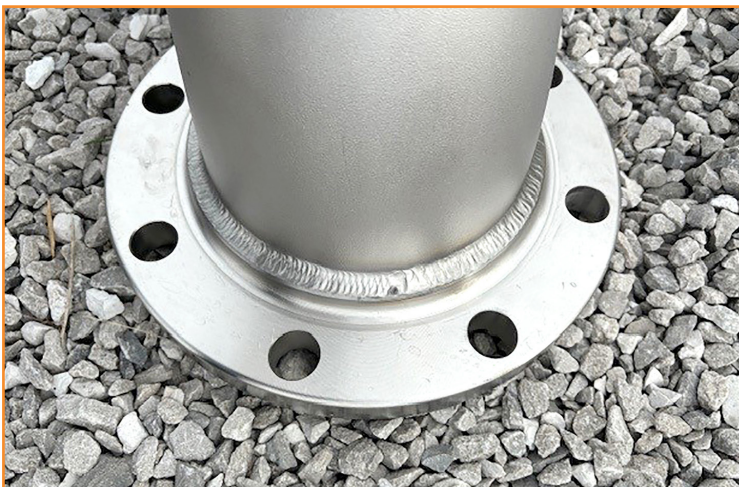
Tyler Jones has been busy with quality welding at the Miller plant during the off season. Pictured, a stainless steel exhaust pipe for a steam return tank.
