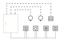
Switches communicate with systems (lighting, roll-down blinds, etc.) via the cabinet and can control any systems, without having to be directly connected.
