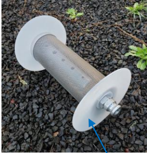
Installed Off-Bottom Props to keep the screen from touching the stream bed - optional
