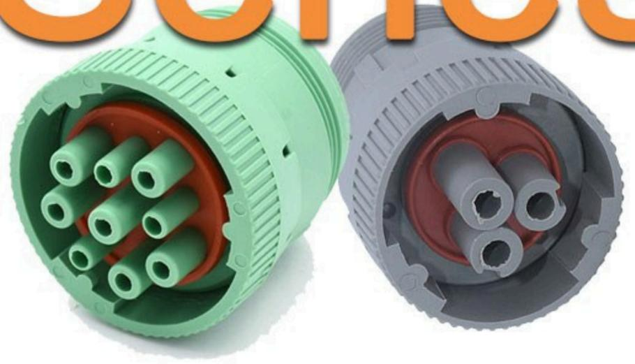
The HD10 series is an environmentally sealed, thermoplastic, and cylindrical connector series. With arrangements from 3 to 9 cavities, HD10 connectors accept size 4, 12, or 16 contacts and are available either in-line or flanged. HD10 connectors are heavily used for diagnostic applications and are available with or without a coupling ring.
