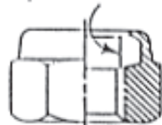
Green nylon insert identifies Greer-Smyrna as manufacturer of locknuts per ANSI/ASME.
