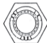
Grade markings per IFI Standard 100 (one or two small notches cut circumferentially into each of the six corners at about mid-height)
