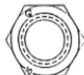
Conelok metric locknuts — Bearing surface
