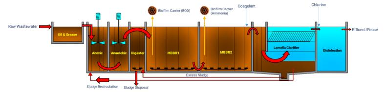
In a BioCar™ system, the wastewater passes through the reactor, and as it flows over the media, microorganisms attach themselves to the surfaces of these carriers, forming a biofilm. The biofilm acts as a substrate for the growth of bacteria, fungi, and other microorganisms that consume organic matter and nutrients in the wastewater.
