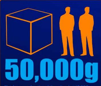
The force at the rim of the wheel at 10,200 rpm. A sugar cube would weigh more than two men
