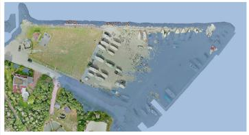
LiDAR derived models can project flooding such as storm surge events.
