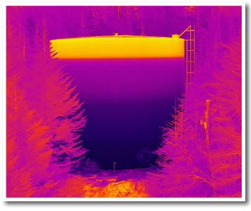
Utilizing state of the art infrared cameras RPM Aerial can capture subtle temperature changes which can be used to detect water levels, sediment levels and in ground water leak detection
