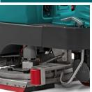
With a stainless-steel frame and components, the Chrome® version guarantees resistance to oxidation and rust caused by corrosive applications and aggressive detergents.
