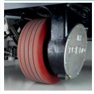
Powerful and reliable, the traction motor is vertically installed in the front part of the machine. The front wheel is driven via a gear box which is lubricated and sealed to protect it against impact, dirt, and humidity.
