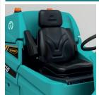
The operator's seat is equipped with weight sensors and a seat belt, it is also possible to cut off power in an emergency or during maintenance operations, guaranteeing maximum protection and safety to operators and mechanics.
