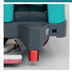
The robust frame realized in thick steel provides protection to both the operator and the internal parts of the machine. The optional overhead guard can be fitted to the E110-D for added safety.
