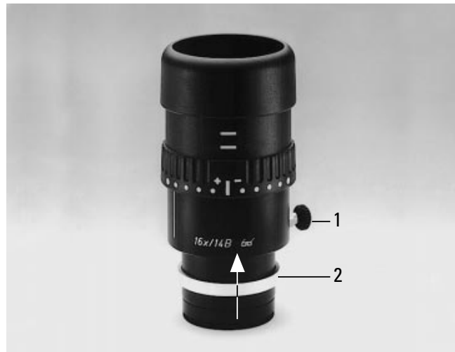
Fig. 93 Eyepiece 16x/14B 1 Clamp screw, 2 Spacer rings for Leica microscopes (must be pushed up as far as the stop)
