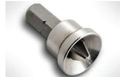
A "Phillips Dimple Bit" is a specialized screwdriver bit, particularly useful for drywall installation. Ensures precise screw depth when installing drywall, countersinking screws to the perfect depth to prevent overdriving and damage to the drywall.
