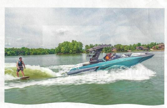
The author at the helm of the latest high-tech wakesurf boat model from Malibu, that actually allows the surfer to determine the wave's size. shape, and even the side of the boat it is created while riding it, via a wireless remote control on his wrist.
