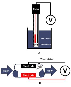
Figure 2: (A) Manual meter and probe, (B) M9 Analyzer conductivity cell
