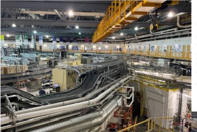
When a synchrotron accelerates electrons, they are "bent" around corners using magnets. When the particles go around the corners they release photons, or little bits of all kinds of light. We can then filter out the spectra, or kinds, of light we want such as Infrared (IR), Ultra-Violet (UV), and X-Ray light.
