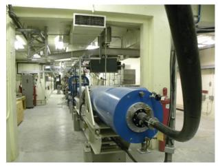
In the electron source, bursts of electrons are injected into an ultra-high vacuum stainless steel tube. These electrons will eventually create the synchrotron light that is used for research.
