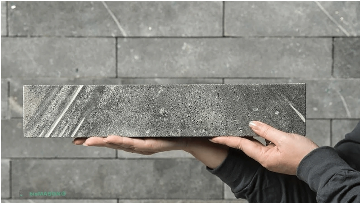
A Biocement block grown by bioMason.
