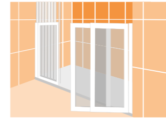
Option 3 One fixed half height 400mm panel with floor to ceiling pole and one sliding door hung from opposite wall
