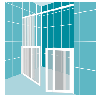
Option 4 Pair of sliding doors hung between walls meeting in middle
