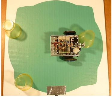
This video explores the use of the Ultrasonic portion of the Range Sensor to clear the Swimming Pool more quickly than the previous method we used.
