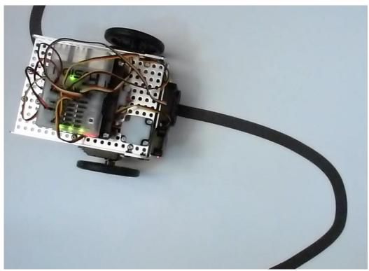
This is a "first look - proof of concept" video that shows Fusion can follow the edge of a line. Please note the slot "A0" to "A1" correction in the video. When Fusion is shown following the edge of a line, it is using the corrected program.
