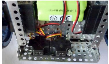
In this "proof of concept" video, we take a first look at Fusion following a line using one Optical Distance Sensor on each side of a line. In our experience, this is an option preferred by many students to the one-sensor edge-following option. The Fusion Basic Kit includes one Optical Distance sensor, but others can be <u>obtained here</u>.
