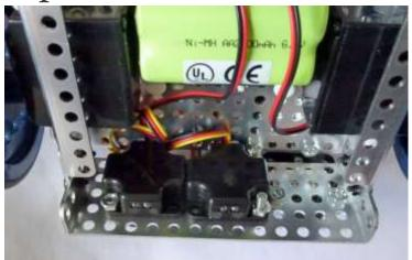
In this "proof of concept" video, we take a first look at Fusion following a line using one Optical Distance Sensor on each side of a line. In our experience, this is an option preferred by many students to the one-sensor edge-following option. The Fusion Basic Kit includes one Optical Distance sensor, but others can be obtained here.
