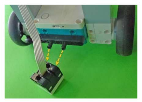
Finally, we can plug the cable from the Color Sensor into slot C on our TAZ1 Robot.
