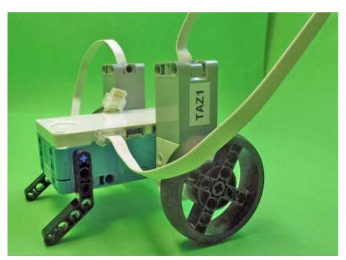
Compare the cable plug and the slot in the computer brick. The plug only goes in one way - DO NOT try to force it in upside down. When you have the plug the right way around, carefully put the plug in to the slot.
