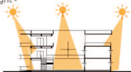
Double Height space for efficient daylight.
