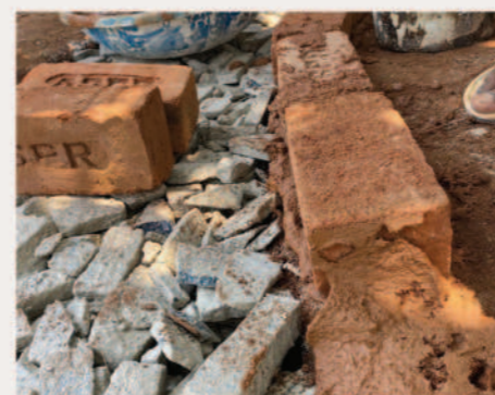
Granite waste mixed with waste limestone
