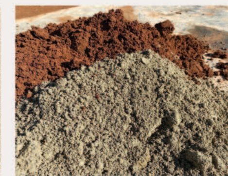
Surkhi mixed with Lime mortar
