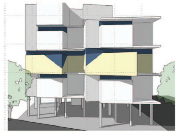
Play with strip window & openings in cantilever slab portion - Kitchen area strip light window & chajja level corner fixed window possibility at kitchen with slab protection above. Glass railing to emphasis on mass, possibility of color/cladding at dynamic floor level.
