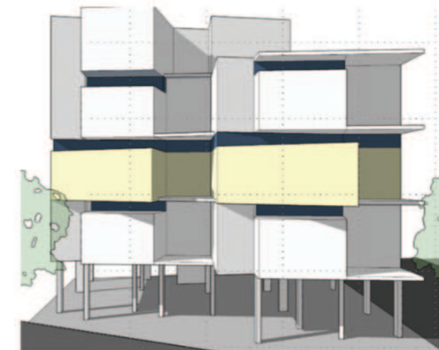
Play with strip window & openings in cantilever slab portion - Kitchen area strip light window & chajja level corner fixed window possibility at kitchen with slab protection above. Glass railing to emphasis on mass, possibility of color/cladding at dynamic floor level.
