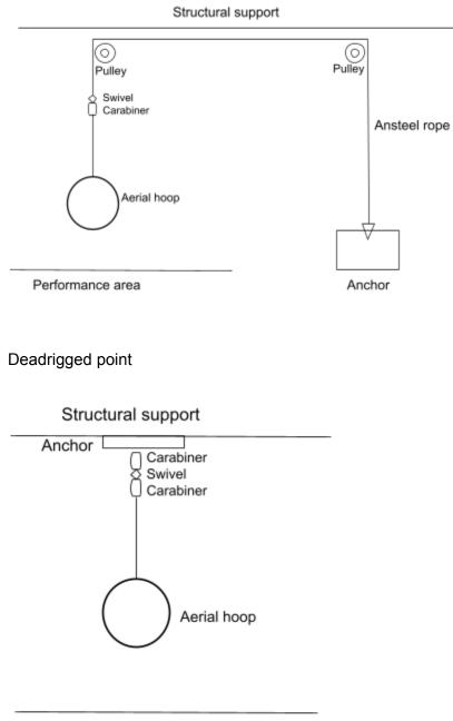
Rigging with pulley system and anchor without mechanical advantage system
