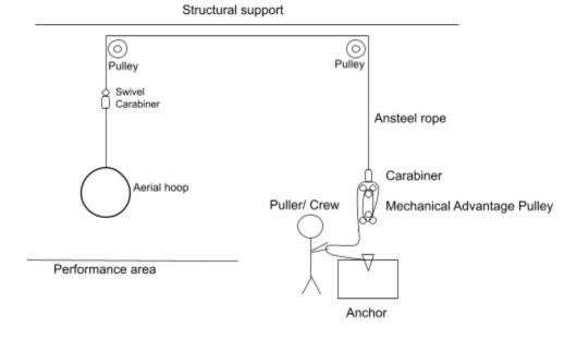
Rigging with pulley system with mechanical advantage system
