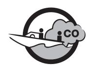
The boat's motor(s) and other equipment such as generators and appliances produce carbon monoxide, a colorless, odorless gas that can cause death quickly. Keep everyone away from the boat's exhaust at all times and keep the boat well ventilated.
