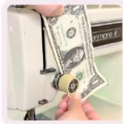
Clean discs using approved material
