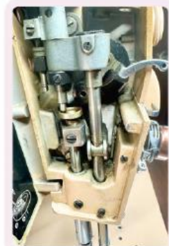
Clean lint & thread from needle bar area
