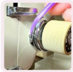
Check spring on external tension system
