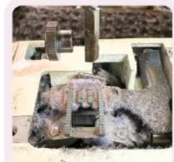
Example of compacted feed dogs.
