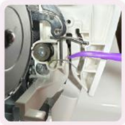
Check spring on internal tension system
