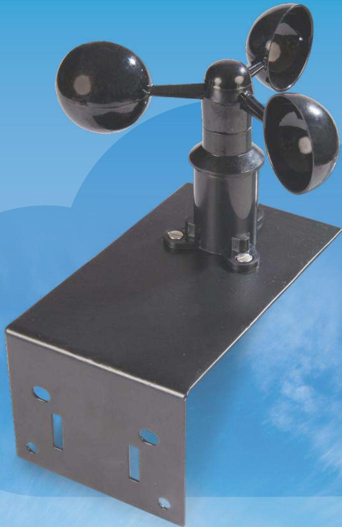
A sensitive instrument for measuring wind speeds. Rugged design and build to withstand strong winds.
