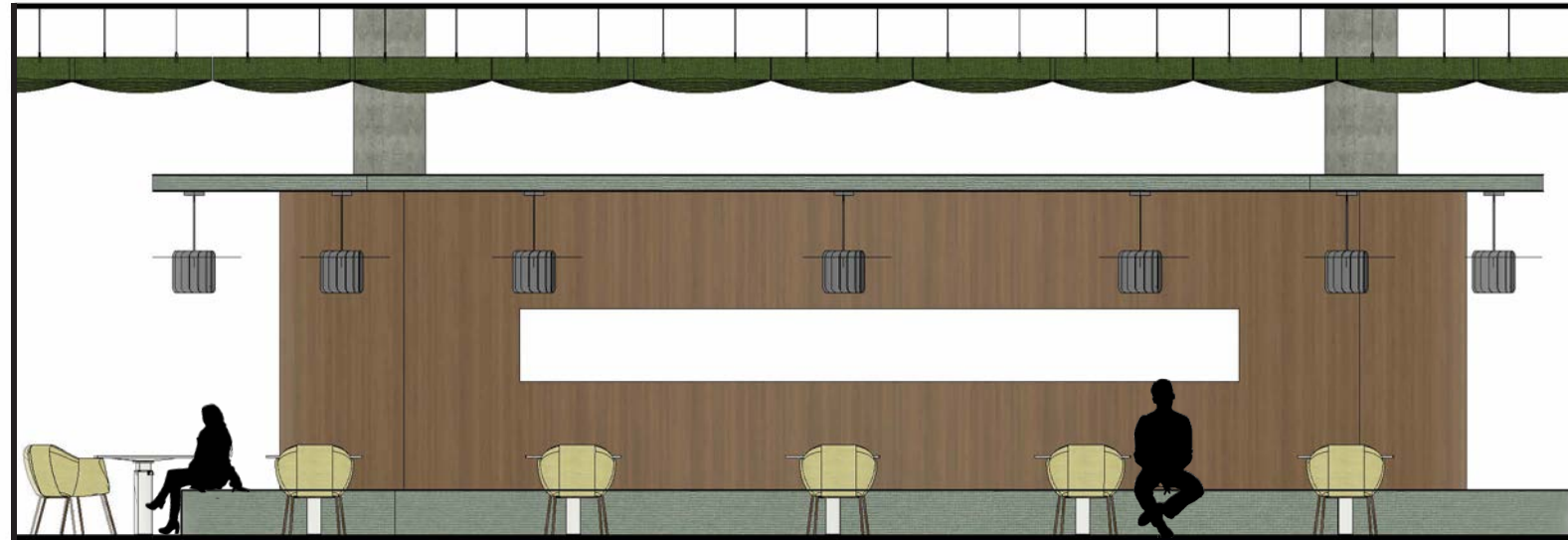
2: Column Seating Elevation Scale: 3/16" = 1' 0"
