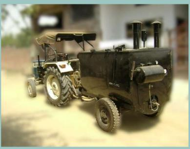
Tractor linked tyre mounted Bitumen-Emulsion Sprayer with Compressor for road dust cleaning is developed for tack / prime coat by hand spraying arrangement and intermittent spraying application with road dust deaning also. This equipment is capable of applying uniform coating of Hot Bitumen & Emulsion on specified surface. A perfect cleaning system cleans the bitumen/ emulsion pipe-line after use.
