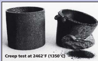
Creep test at 2462°F (1350°C) Schunk-INEX tube on left tested for 360 hours. The alloy tube on right was tested for less than one hour.
