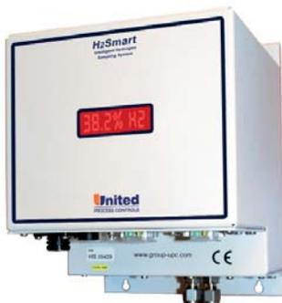
The **H2Smart™**, complete with an integrated sampling system, is designed to measure hydrogen content with high accuracy in nitriding and nitrocarburizing atmospheres and to calculate the parameters necessary for process control:  $p_{H_2}$ ,  $p_{NH_3}$ ,  $p_{O_2}$ ,  $p_{CO}$ ,  $p_{CO_2}$ ,  $K_N$ ,  $K_C$ ,  $K_O$  and % dissociation.
