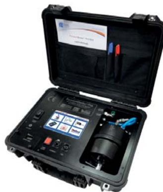
The **FurnaceDoctor®-Pro** provides accurate infrared measurement of  $CO$ ,  $CO_2$ , and  $CH_4$  and computes the % carbon, Dew-point and expected carbon probe millivolts.
