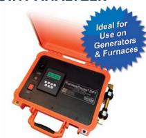
The easy-to-use **The FurnaceDoctor®-DPT Dewpoint Analyzer** can provide oxygen probe operation verifications. Includes equivalent % carbon calculation.
