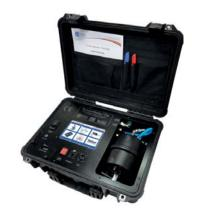
**The FurnaceDoctor®-Pro** provides accurate infrared measurement of CO, CO<sub>2</sub>, and CH<sub>4</sub> and computes the % carbon, Dew-point and expected carbon probe millivolts.
