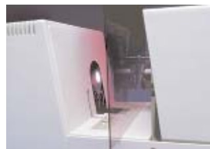
A spacious transmission compartment allows convenient manipulation of samples to obtain the most accurate measurements possible.
