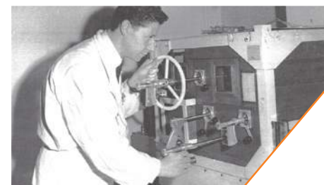
1959 - M. Robert JAMES handling 131 I dose in a Lemer shielded hot cell (the first user of a French hot cell) in the radioisotope service of Professor Tubiana at the Gustave Roussy Institute, Paris, France.
