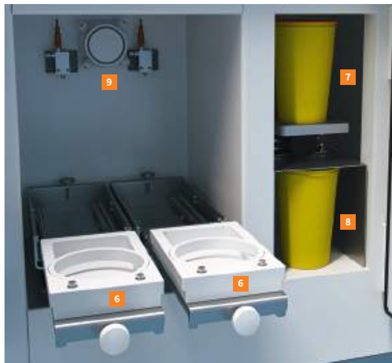
1 | 2 Independent accesses for 2 generators 2 | Access to the dose calibrator chamber 3 | Choice of electrical, USB and RJ45 sockets 4 | 2 UV germicidal tubes 5 | 2 independent accesses for 2 waste bins 6 | 2 independent slide trays with lifts for 2 generators 7 | Waste compartment 8 | Storage or decay area 9 | Very high efficiency filter 10 | Airlock chamber inner shielded door with manual opening handle 11 | Lateral shielded airlock chamber with front opening and integrated sliding tray
