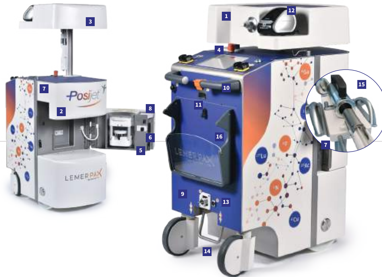
1 | Manual injection plunger 2 | Dose calibrator for real-time measurement of radiopharmaceutical dose 3 | Secure automatic preparation and controlled injection system in automatic or manual mode 4 | Touch screen for control and command 5 | Secure shielded door accommodating the multi-dose vial in its shielded transport container 6 | Air bubble detector 7 | Saline solution holder connected to the mother solution kit 8 | Removable spill containment tray 9 | Mains outlet 10 | Motorised rotary assistance control (independent battery) 11 | Bar code reader for kit traceability 12 | Printer for customisable injection and quality control reports 13 | Ethernet connection if no Wifi 14 | Castor braking system 15 | Optional RIS (Remote Injection System) allows preparation and packaging of a patient dose for manual injection 16 | Maintenance hatch
