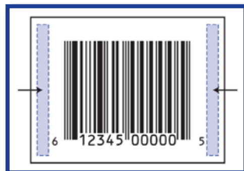
4.3.2d Quiet Zones: Quiet zones allow scanners to detect when a bar code starts and stops. Minimum quiet zone specifications depend on the symbol specified and its magnification.
