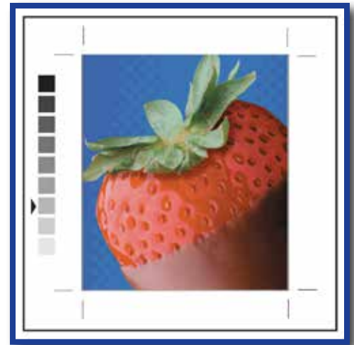
5.3 Grayscale Aim Point: The aim point of the shot should be the 40% neutral gray swatch or the number 3 or 4 block on the photographer's scale.
