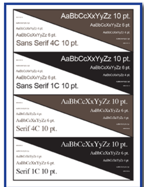
4.1b Minimum Type Size: Using type sizes below the printer's minimum recommended size can result in type filling and is not supported by FIRST.
