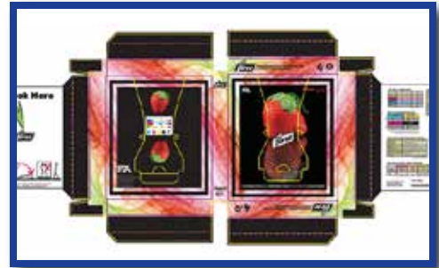
3.6a Profiled Contract Proof: The contract proof must include a control target as well as template layout markings.
