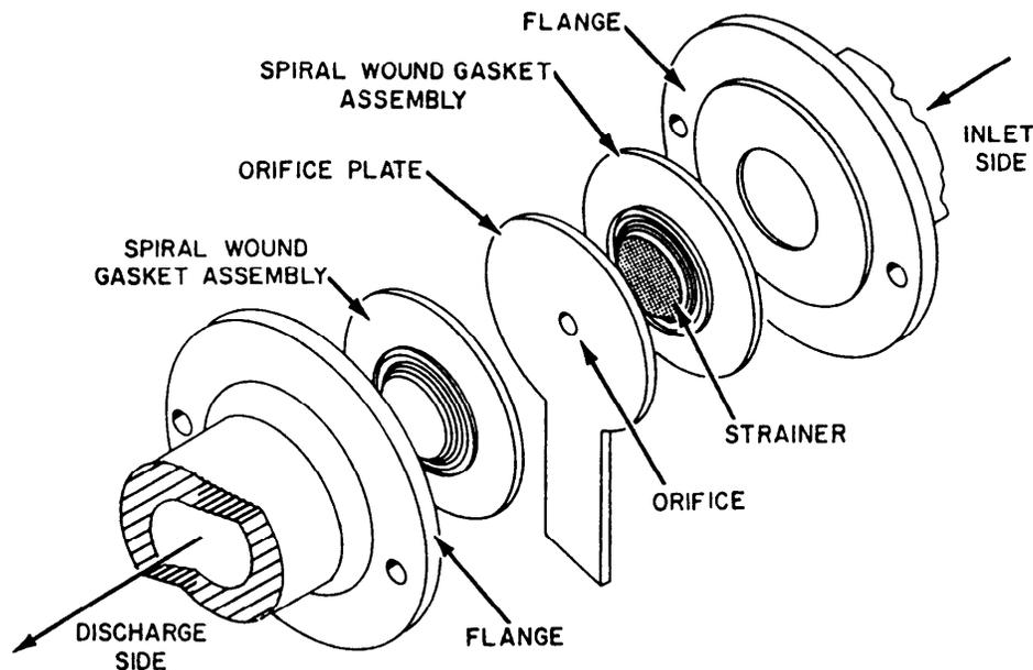
Figure 10-30.—Orifice-type steam trap assembly.
