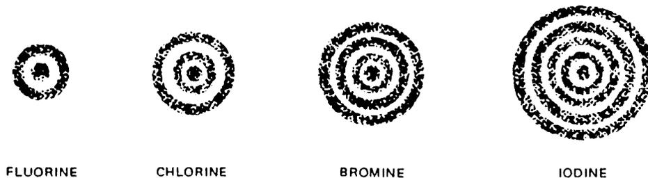
NOTE: THE DARK AREAS REPRESENT THE ELECTRON CLOUDS OR SHELLS. THE NUCLEI OF THE ATOMS HAVE NOT BEEN SHOWN. THE DARK AREAS IN THE CENTER REPRESENT THE INNERMOST SHELL.
