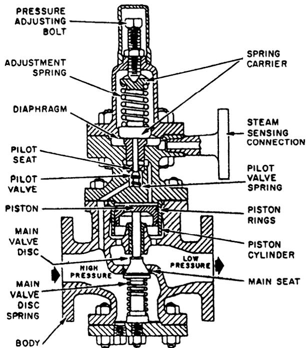
Figure 10-19.—Reducing valve (Atlas Valve Company).
