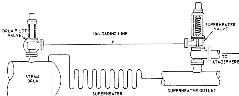
Figure 16-23.—Two-valve superheater outlet safety valve assembly.
