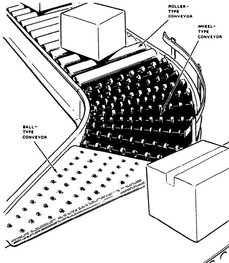
Figure 14-5.—Gravity conveyor.
