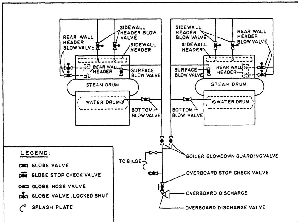
Figure 16-16.—Boiler blow piping.
