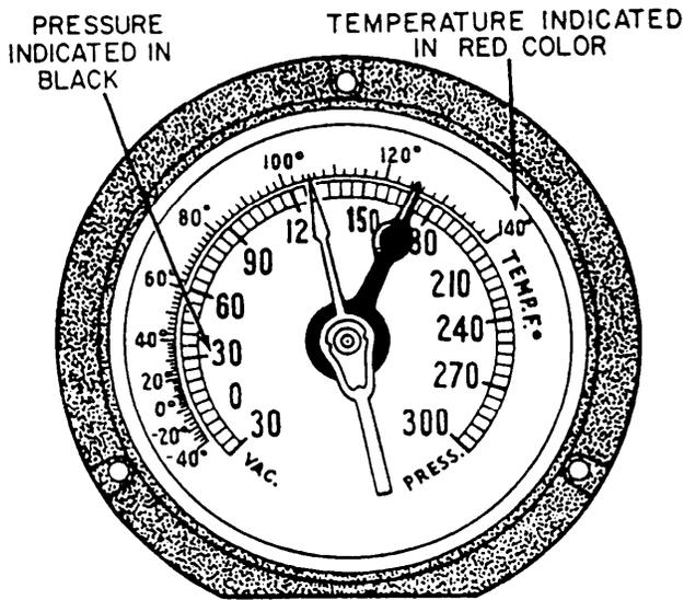
Figure 11-18.—Compound R-12 pressure gauge.
