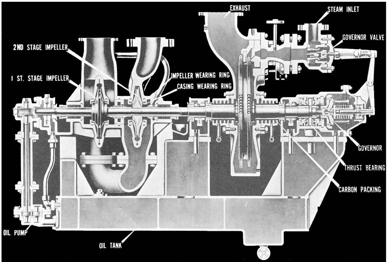
Figure 5-4.—Two-stage main feed pump.
