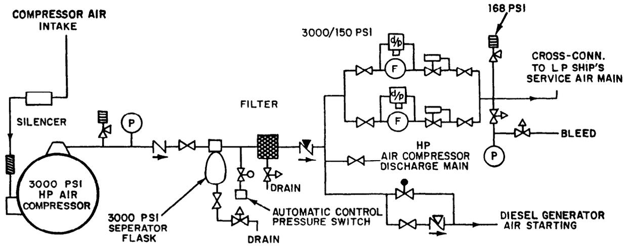
(A) HP AIR COMPRESSOR AND CROSS CONNECTION REDUCING STATION
