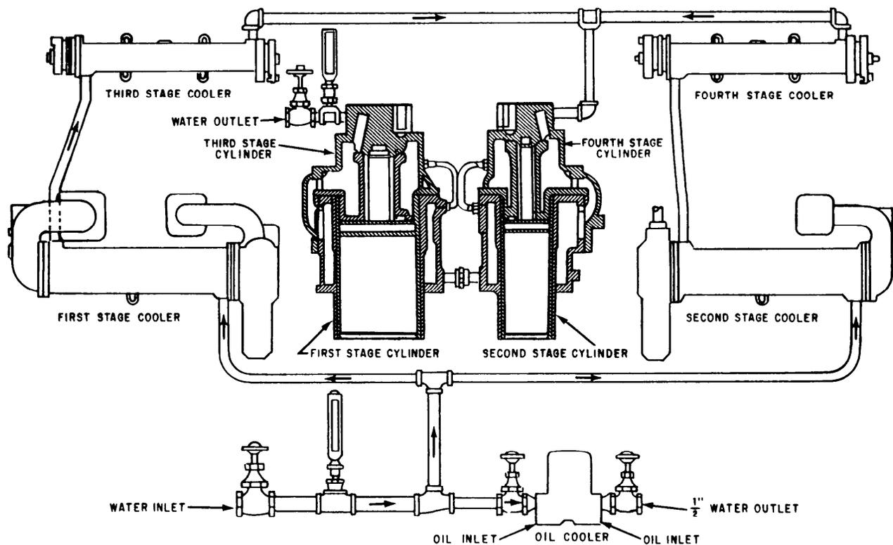
Figure 13-9.—Cooling water system in a typical multistage air compressor.
