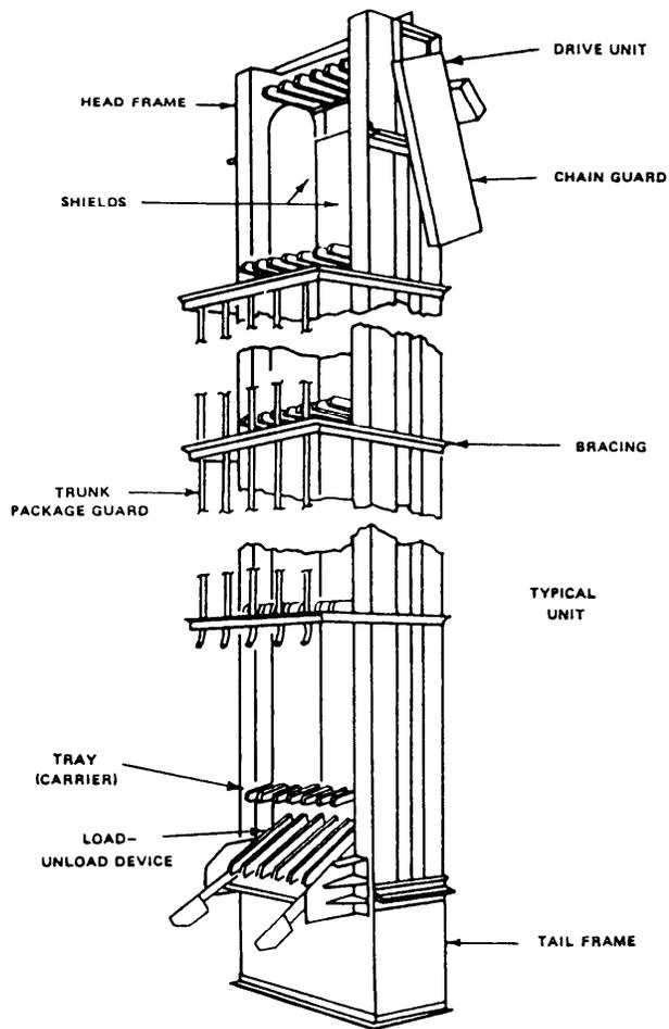
Figure 14-6.—Vertical conveyor, package, tray type.
