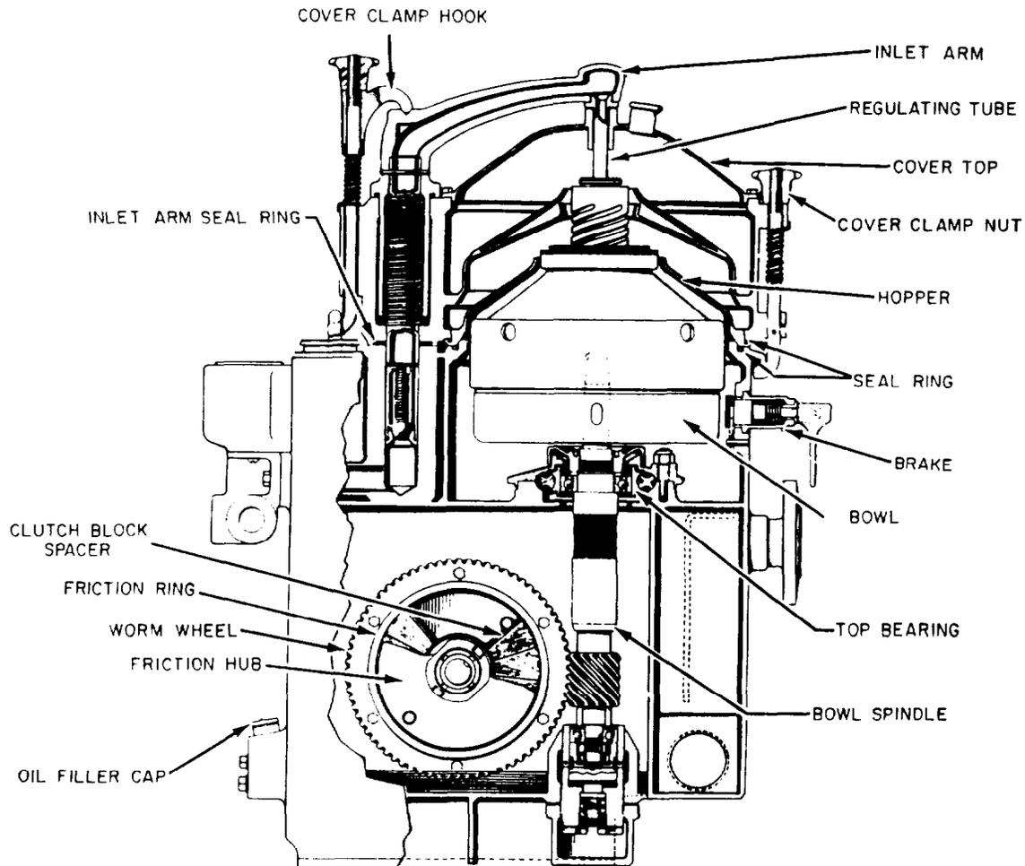
Figure 4-5.—Disk-type centrifugal purifier.
