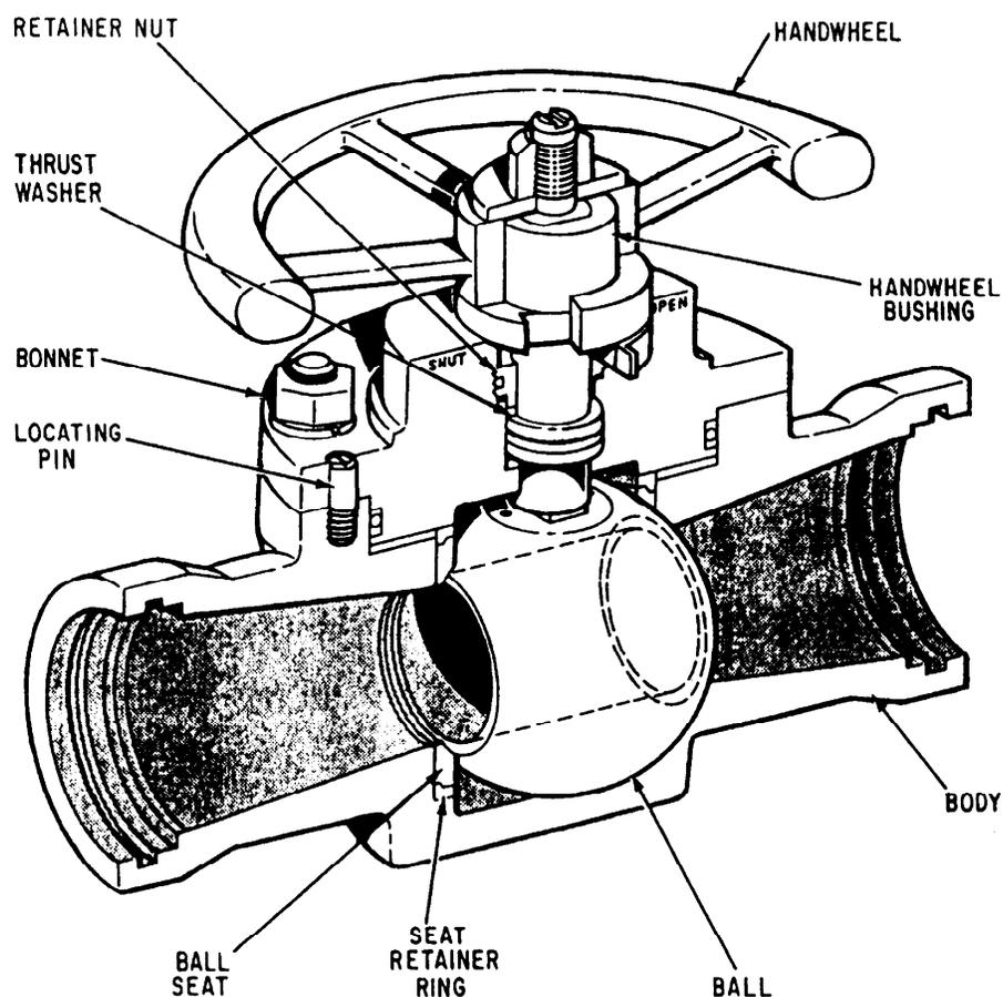
Figure 10-14.—Typical seawater ball valve.
