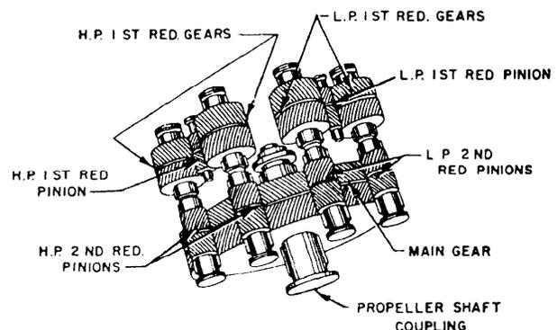
Figure 3-1.—Articulated locked train, double-reduction gear.
