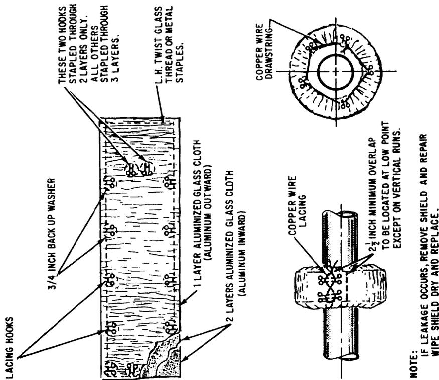
Figure 10-7.—Flange safety shields.
