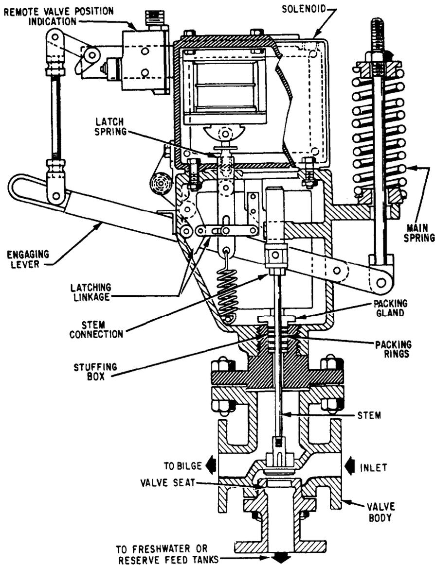
Figure 9-6.—Three-way solenoid trip valve.
