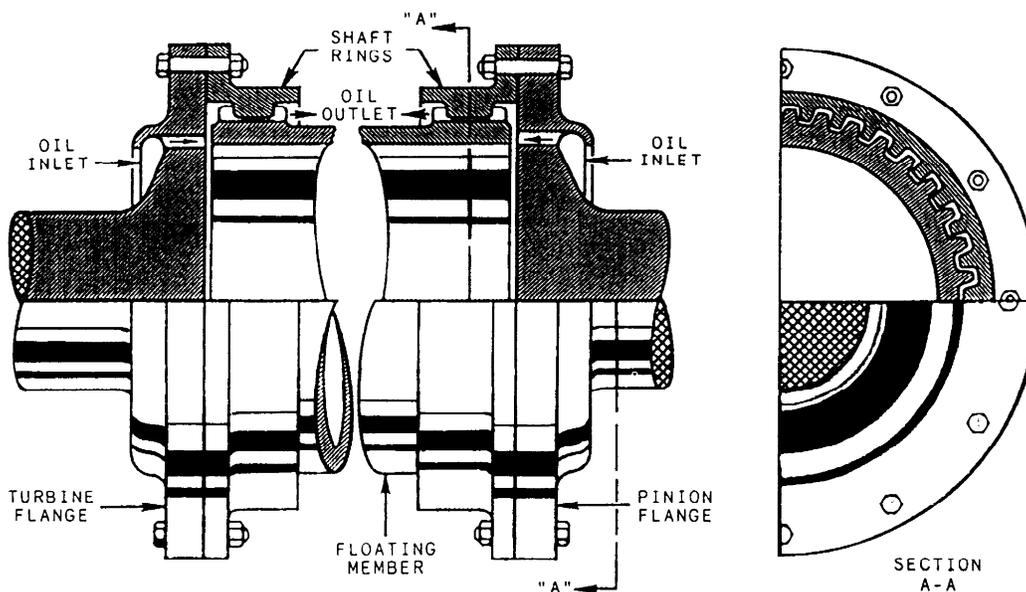
Figure 3-6.—Gear-type flexible coupling.
