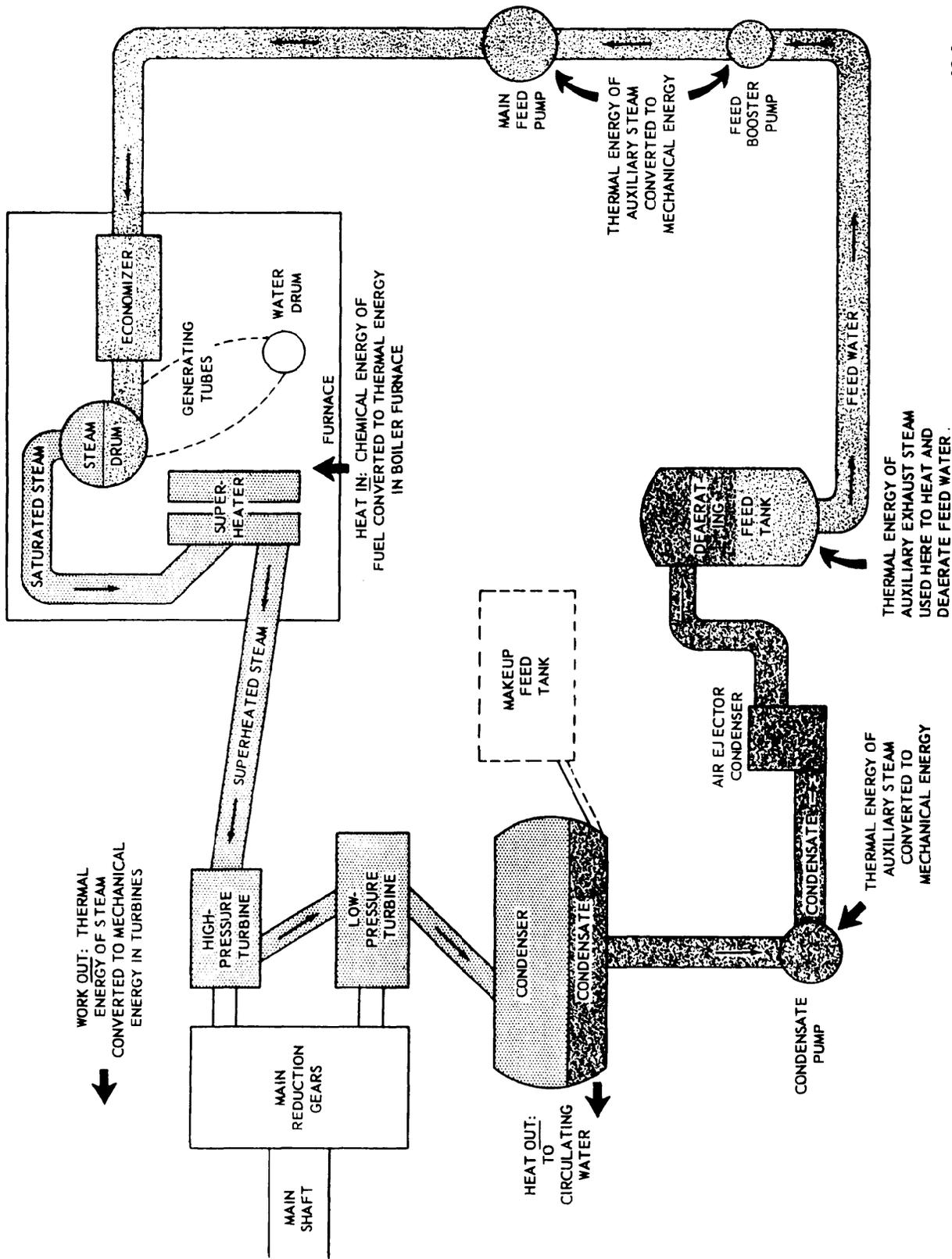
Figure 2-1.—Energy relationships in the basic propulsion cycle.
