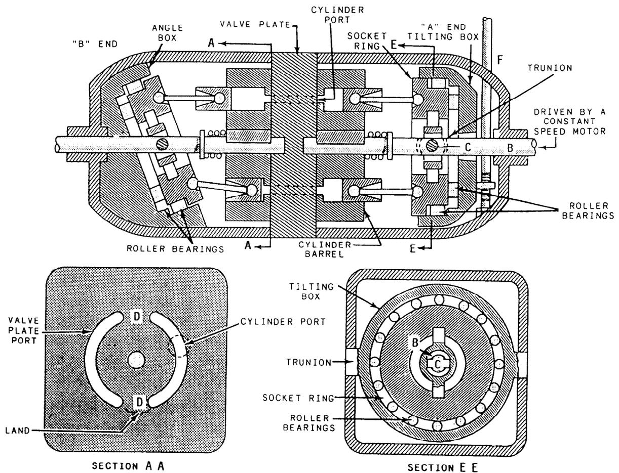
Figure 5-14.—Axial piston hydraulic speed gear.
