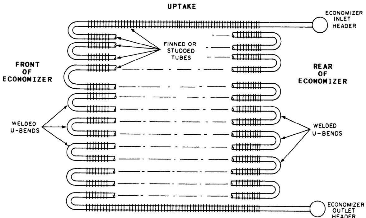
Figure 15-8.—Side view of economizer showing one element.
