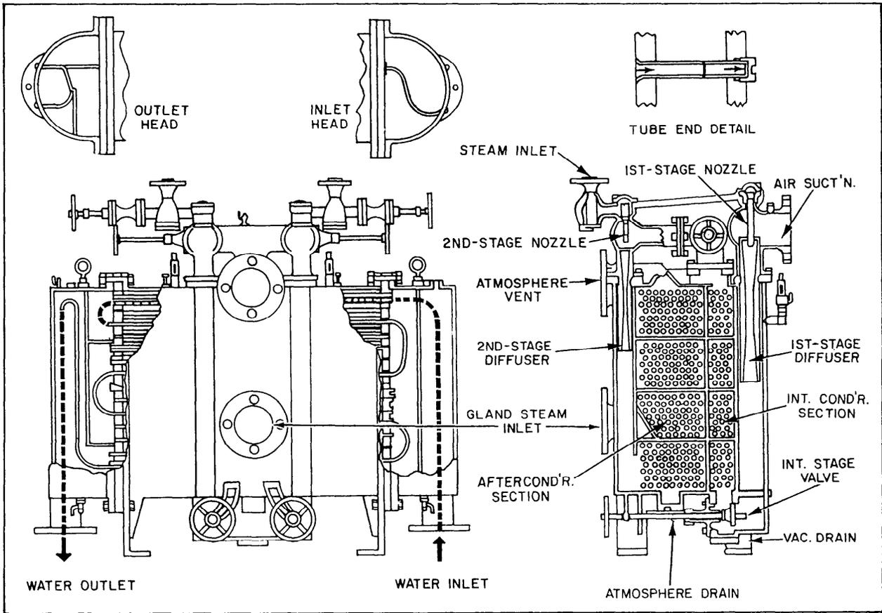
Figure 6-14.—A main air ejector and condenser assembly.
