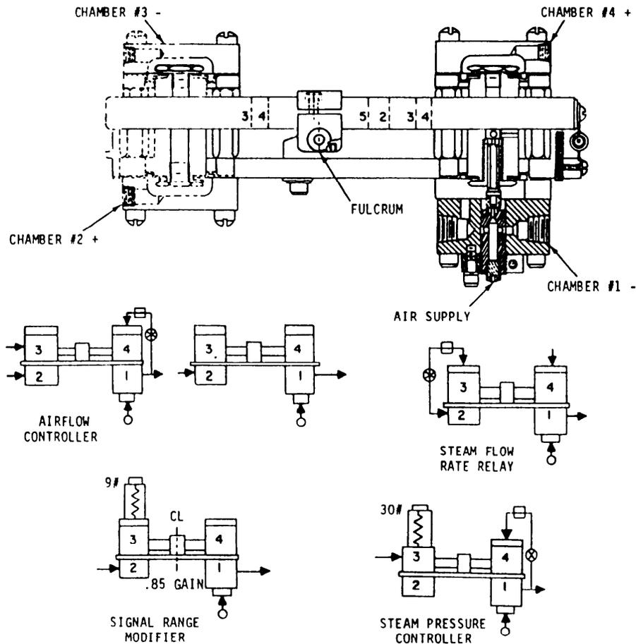
**NOTE:** A SPRING BARREL AND SPRING ASSEMBLY CAN BE ATTACHED TO CHAMBERS 2, 3, OR 4 TO INDUCE A MECHANICAL INPUT FORCE.
