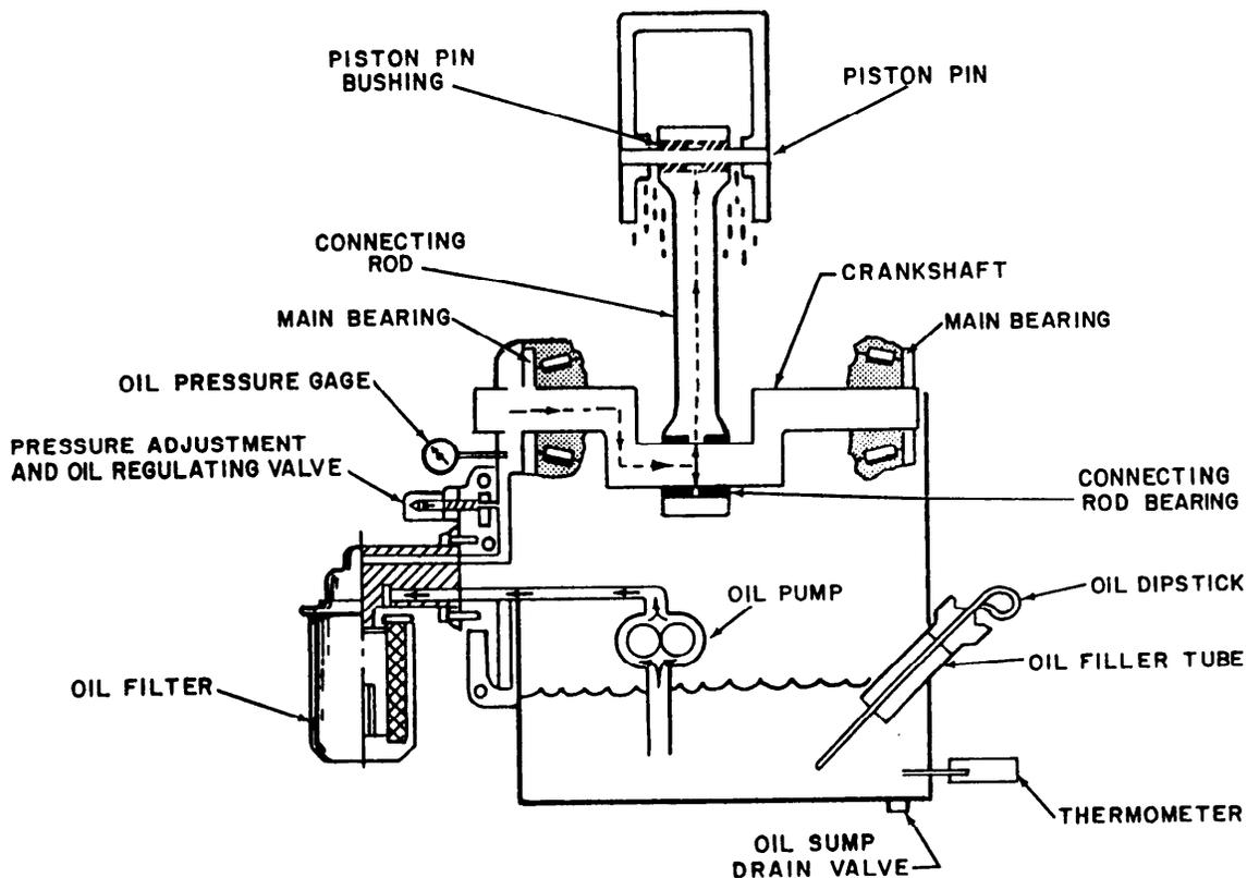
Figure 13-8.—Lubricating oil system of a low-pressure air compressor.
