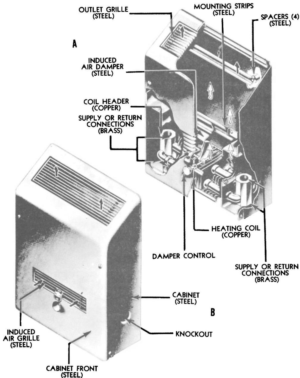
Figure 12-11.—Convection heater: A. Cutaway view. B. Exterior view.
