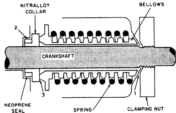
Figure 11-8.—Rotating bellows seal.
