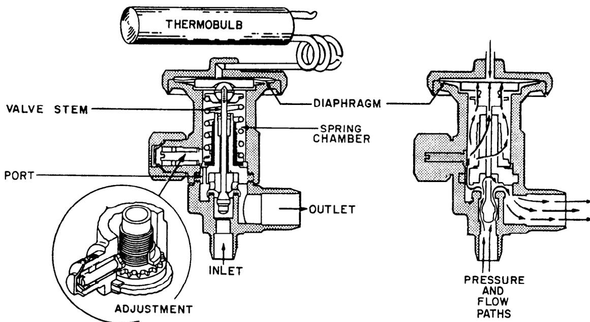
Figure 11-20.—Thermostatic expansion valve.
