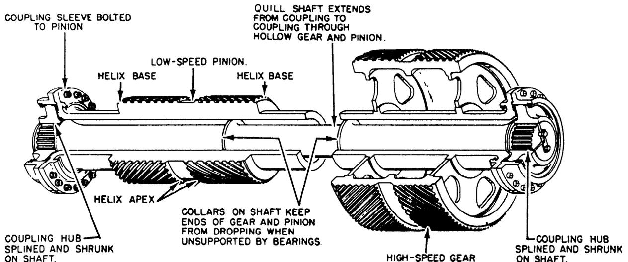
Figure 3-4.—Cutaway view of intermediate rotor assembly articulated gear.
