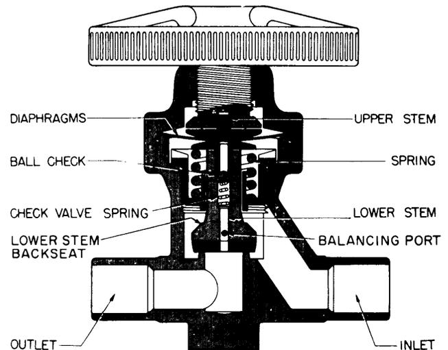
Figure 11-19.—Packless valve for refrigeration system.
