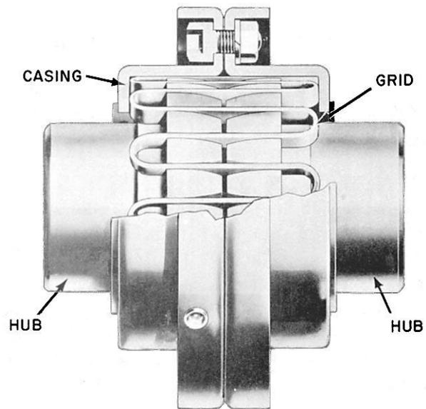
Figure 5-7.—Grid-type flexible coupling.
