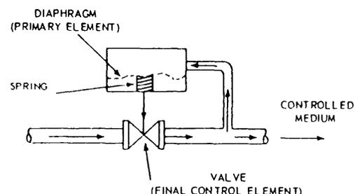
Figure 17-4.—Self-operated controller.
