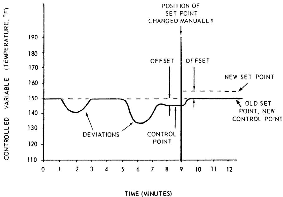
Figure 17-7.—Proportional-position action applied to a heat exchanged process.
