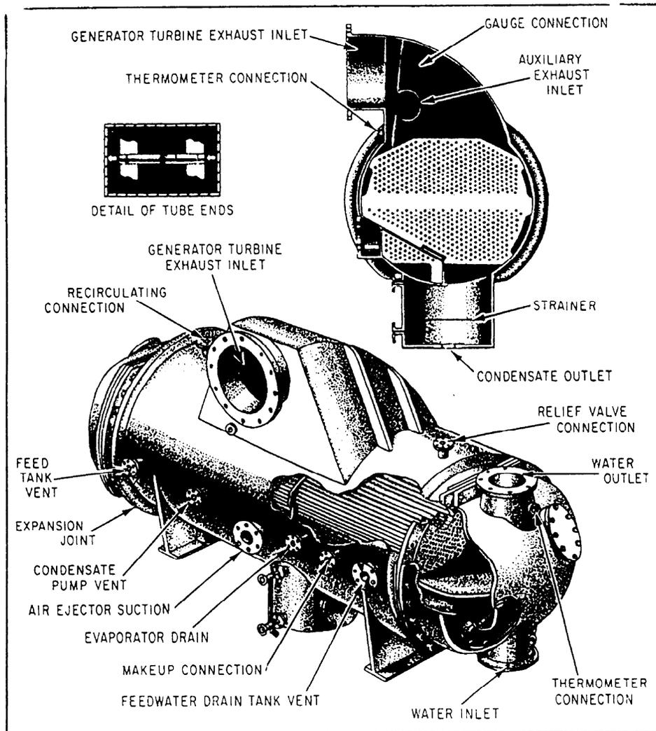
Figure 6-7.—Auxiliary condenser (turbogenerator).
