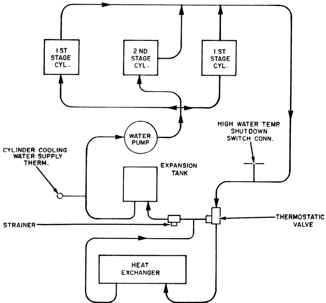
Figure 13-22.—Cylinder cooling water flow diagram.
