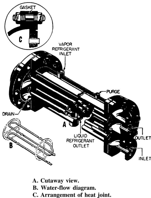
Figure 11-11.—Watercooled condenser for R-12 refrigeration system.
