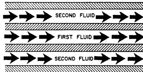
Figure 6-1.—Parallel flow in a heat exchanger.
