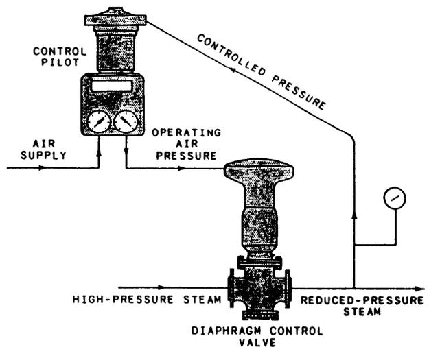
Figure 10-24.—Arrangement of control pilot and diaphragm control valve for supplying reduced steam pressure.
