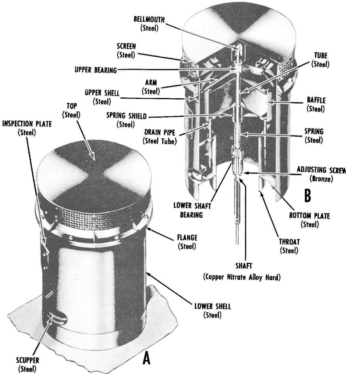
Figure 12-4.—Waterproof ventilators: A. Exterior view. B. Cutaway view.
