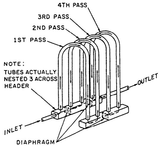
Figure 15-7.—Vertical U-shaped tubes and steam flow through the superheater.
