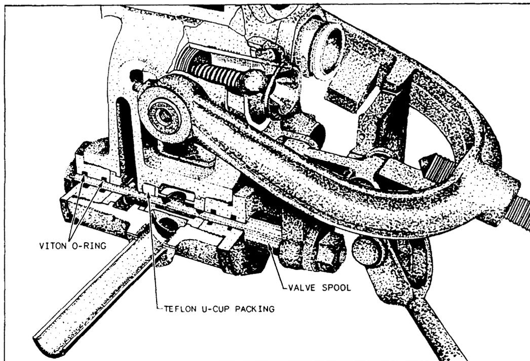
Figure 16-30.—Cutaway view of fuel-oil safety shutoff device.
