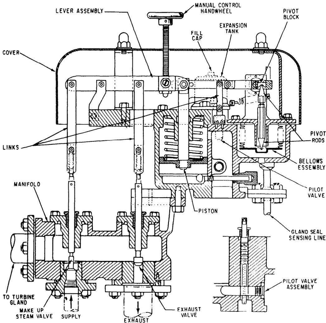
Figure 2-20.—Hydraulic type turbine gland seal regulator.
