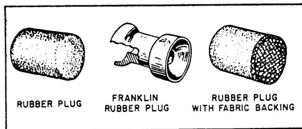
Figure 6-8.—Types of rubber plugs used for cleaning condenser tubes.
