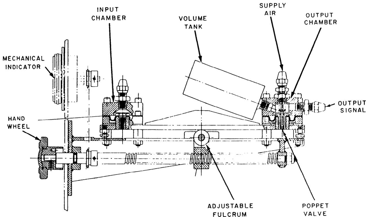
Figure 17-16.—F/A ratio signal generator (excess air adjuster).
