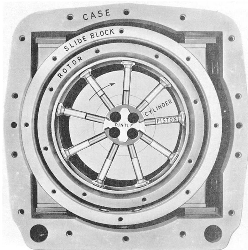
Figure 5-15.—Nine-piston radial piston pump.
