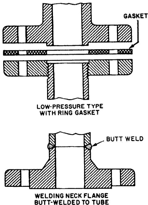
Figure 10-2.—Bolted flange piping joints.
