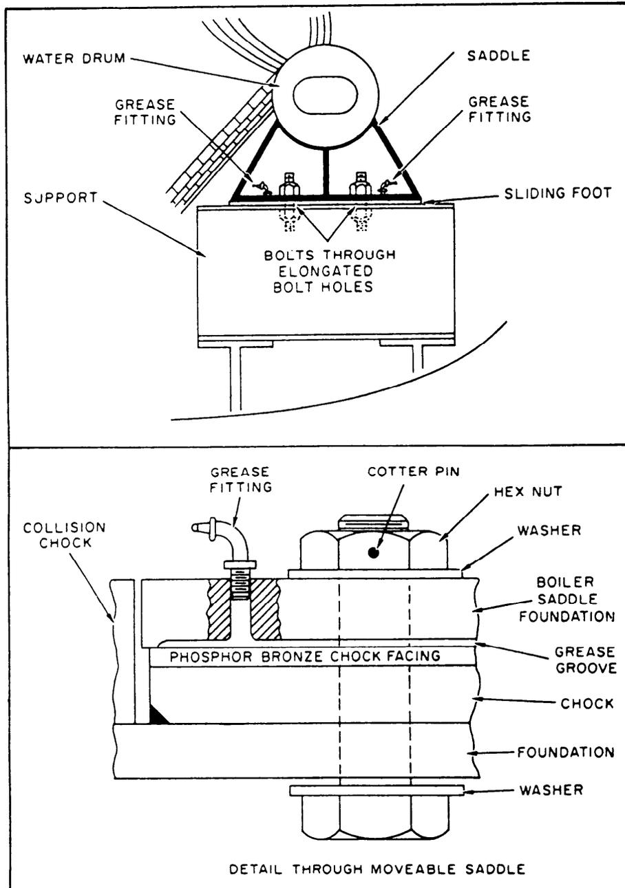
Figure 15-11.—Boiler saddle, support, and sliding feet.
