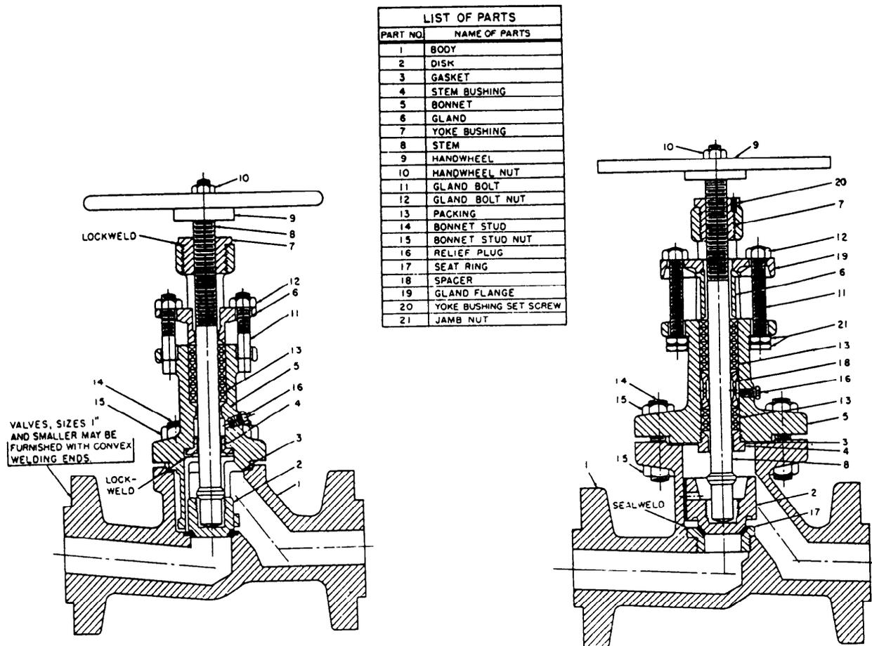
Figure 16-10.—Stop-check valves.
