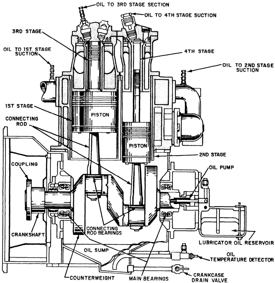
Figure 13-7.—High-pressure air compressor.
