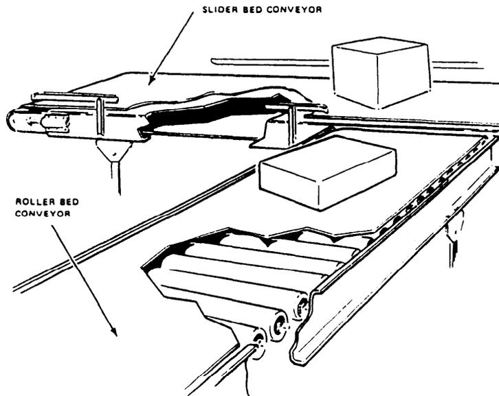
Figure 14-8.—Powered belt conveyor.
