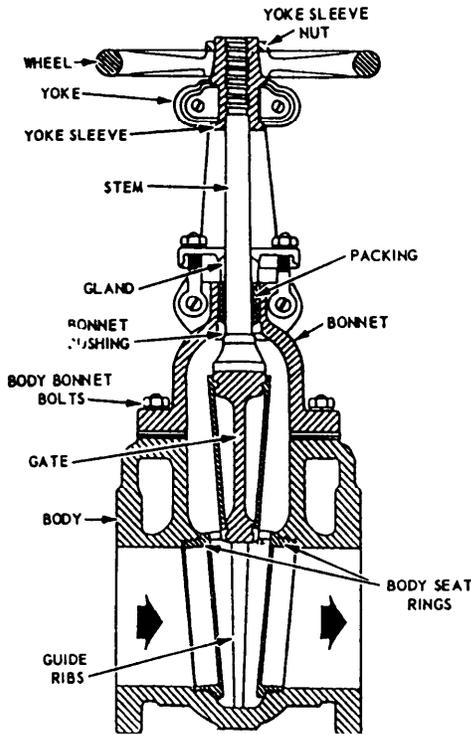
Figure 10-12.—Cutaway view of a gate stop valve (rising stem).
