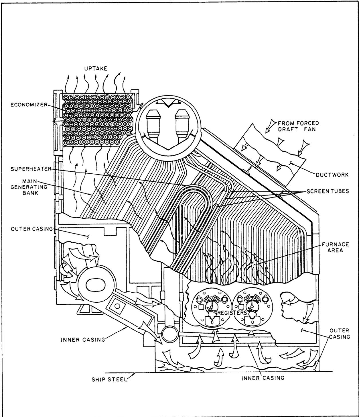
Figure 15-12.—Combustion air and gas flow.
