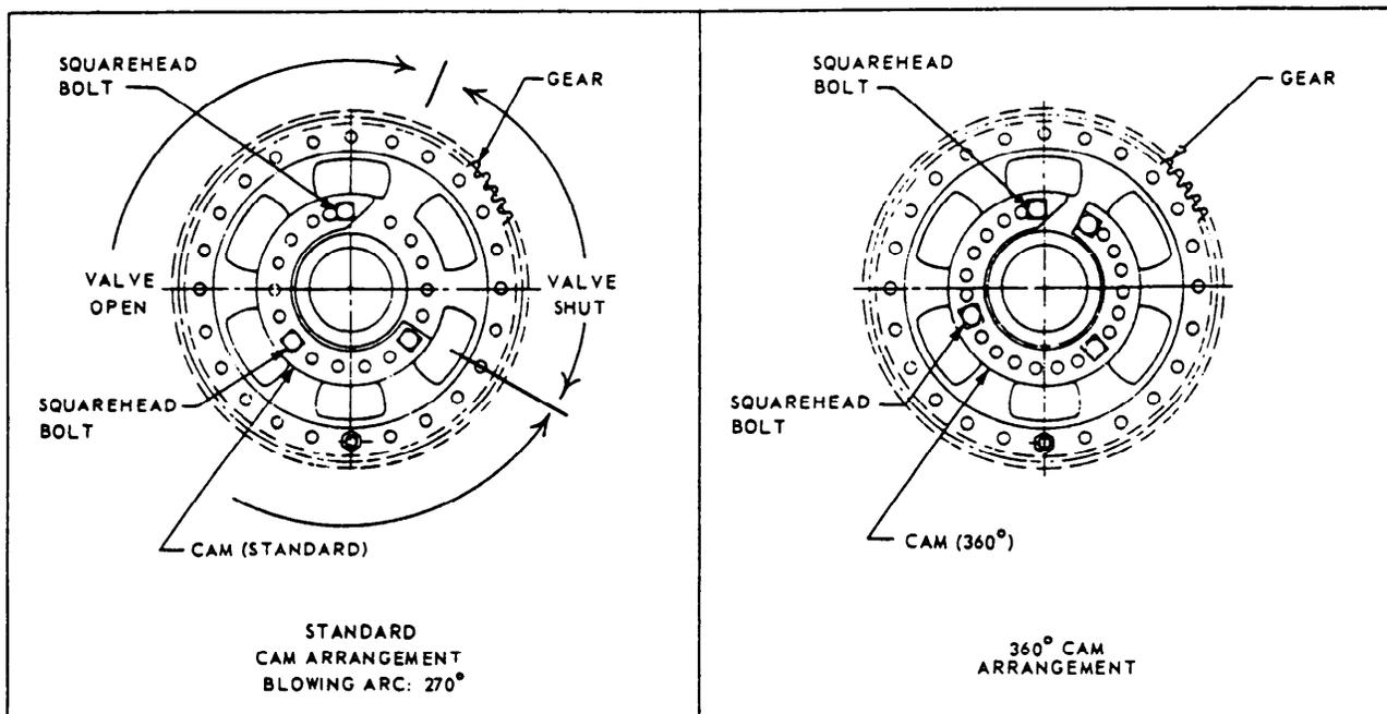
Figure 16-14.—Cam-and-gear assemblies for controlling blowing arcs on multinozzle soot blowers.
