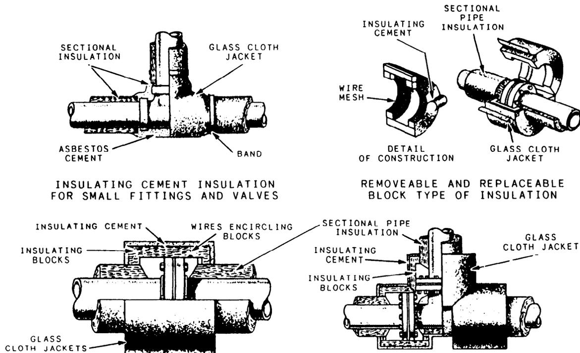
Figure 10-37.—Permanent-type insulation of pipe fittings, flanges, and valves.
