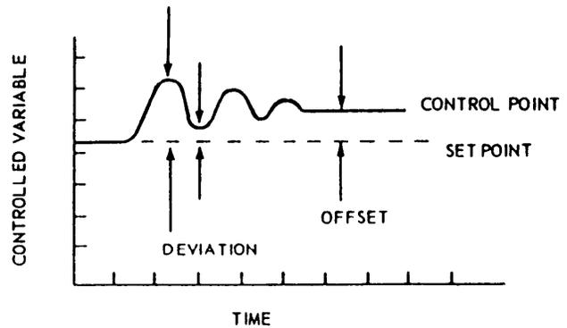
Figure 17-5.—Set point, deviation, control point, and offset in an automatic controller.
