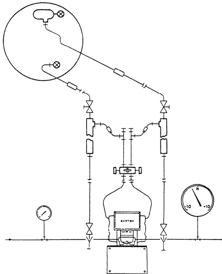
Figure 16-19.—Typical drum-level measurement installation for a second type of remote water-level indicator.
