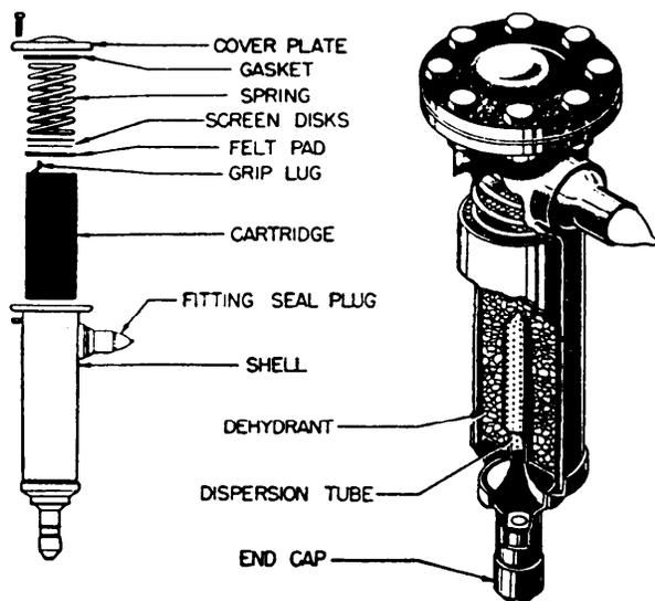
Figure 11-13.—Refrigeration dehydrator.
