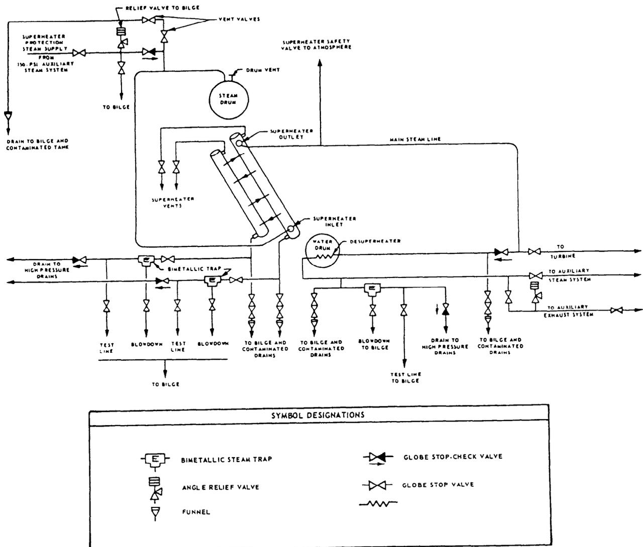
Figure 16-9.—Diagrammatic arrangement of superheater vents, drains, and protection steam connections.
