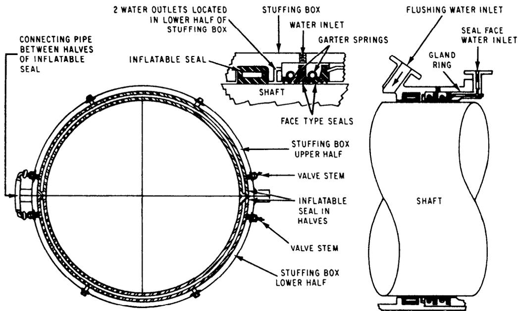
Figure 3-19.—Shaft seal and inflatable sealing ring.
