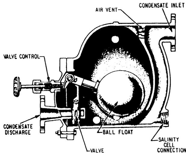
Figure 10-26.—A ball-float steam trap.
