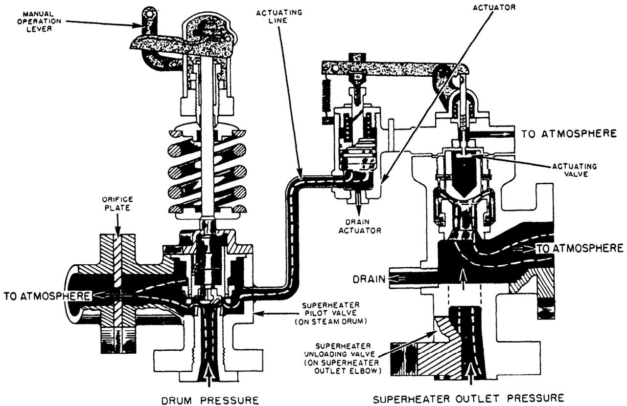
Figure 16-24.—Three-valve superheater outlet safety valve assembly.
