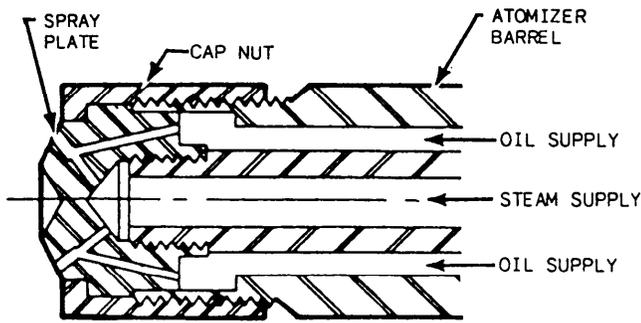
Figure 16-27.—Y-jet steam atomizer.
