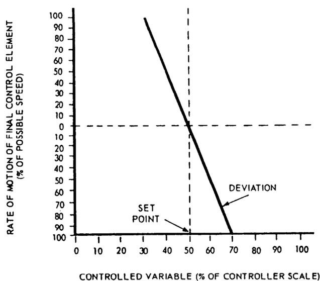
Figure 17-8.—Proportional-speed floating action.
