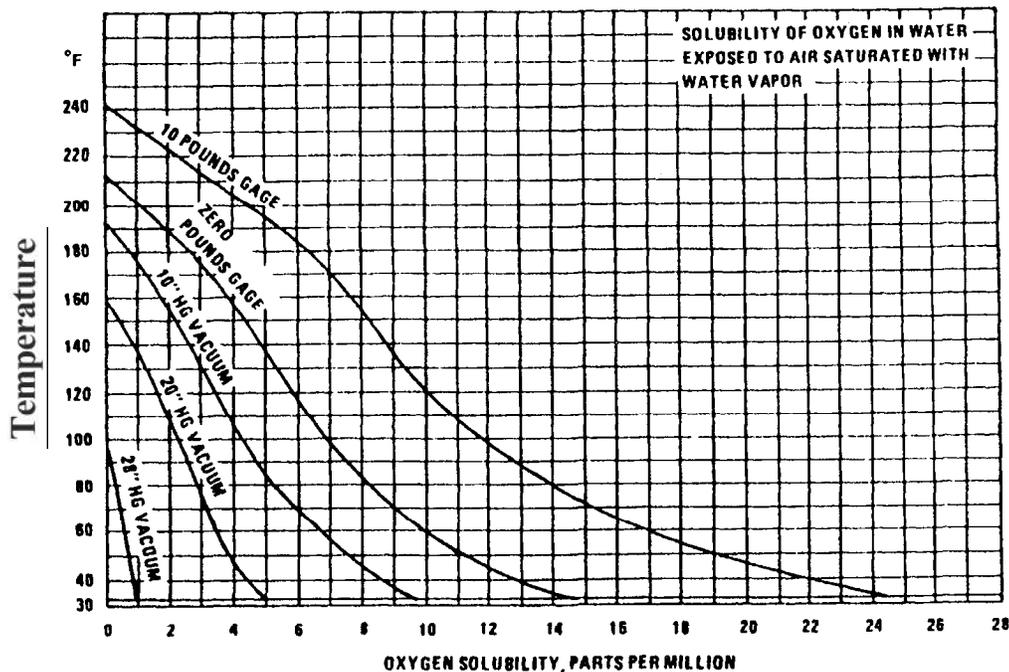
Figure 18-7.—Oxygen-dissolving capabilities of water.
