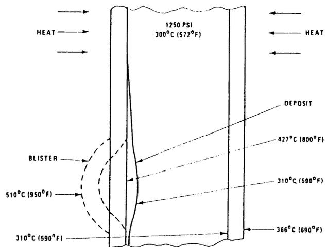
Figure 18-6.—Effect of boiler deposit.
