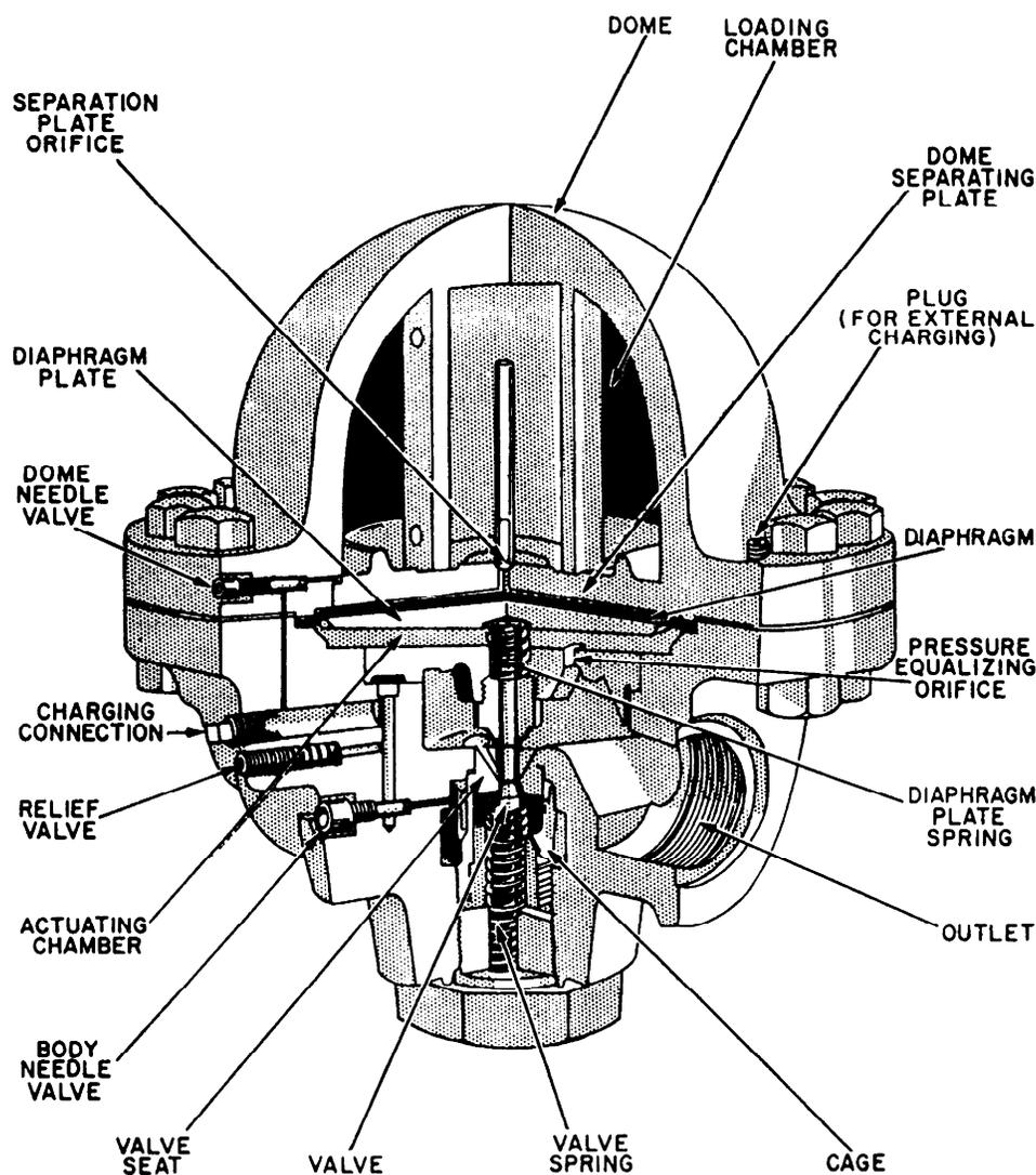
Figure 10-20.—Pneumatic-pressure-controlled reducing valve for low-temperature service.
