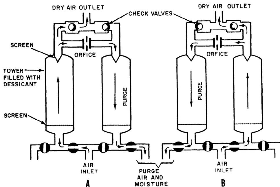
Figure 13-15.—Heat-less dehydrator.
