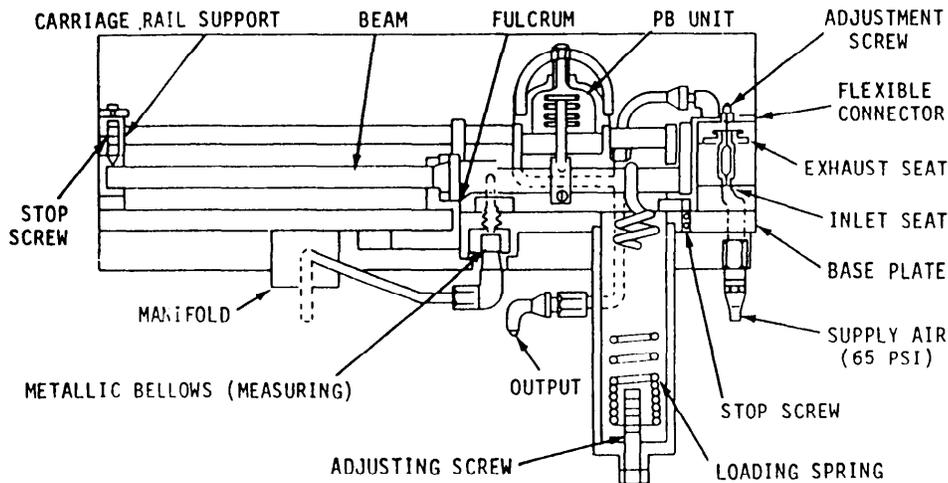
Figure 17-12.—Steam pressure transmitter.
