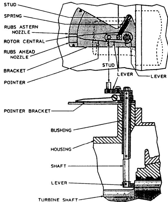
Figure 2-34.—Axial clearance indicator.
