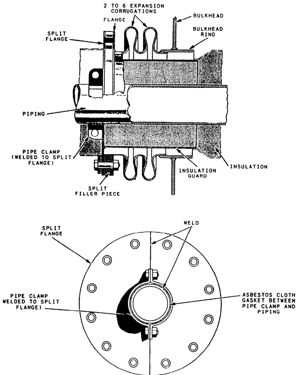
Figure 10-6.—Corrugated bulkhead expansion joints, showing details of installation.
