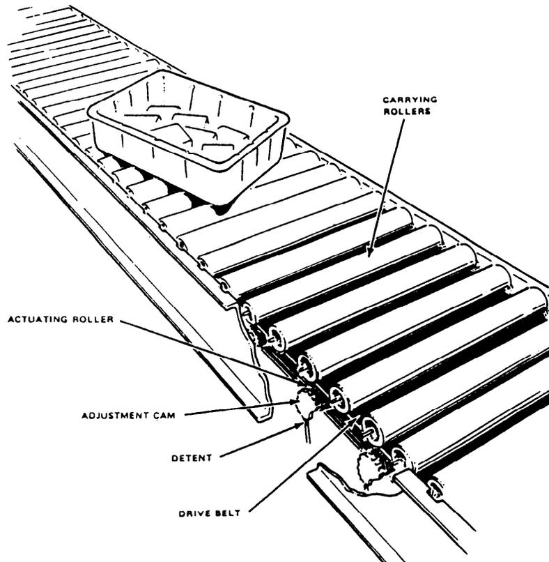
Figure 14-9.—Powered roller conveyor.
