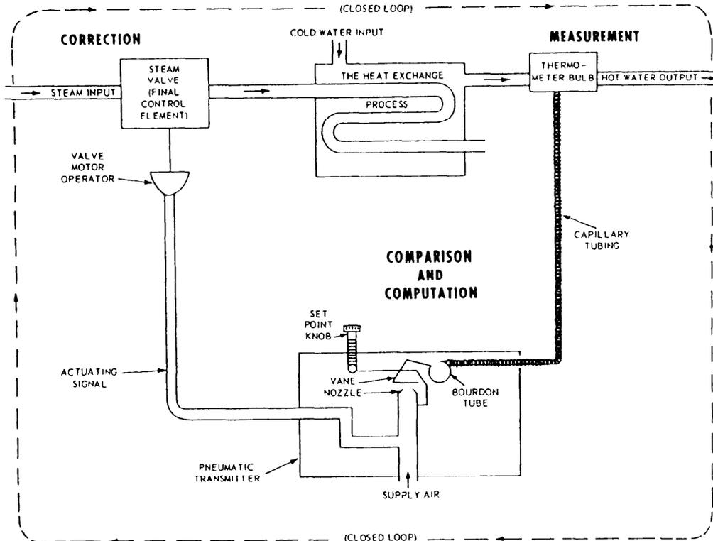
Figure 17-3.—Simple automatic control system (pneumatic) for control of heat exchange process.
