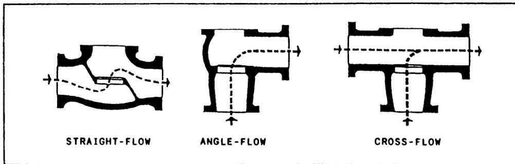
Figure 10-8.—Types of globe valve bodies.
