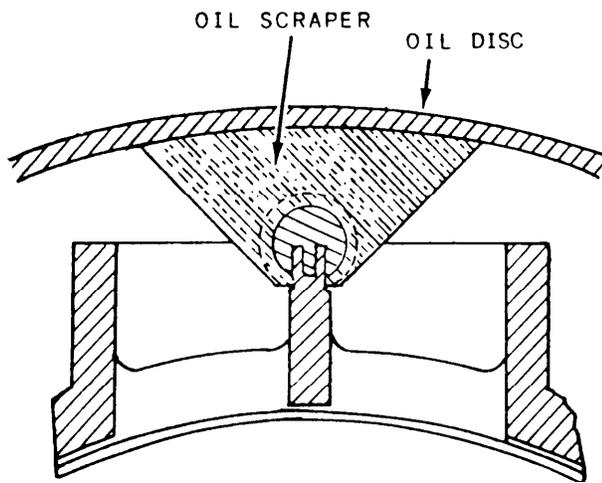
Figure 3-17.—Disc-oiled line shaft bearing scraper arrangement.
