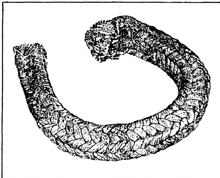
Figure 10-35.—Graphite filament yarn.
