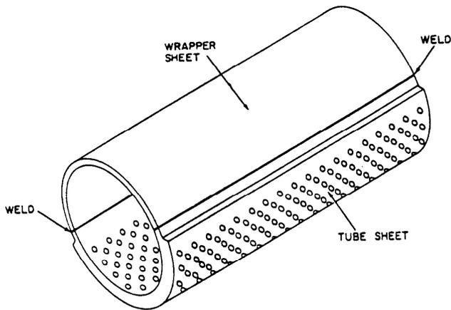
Figure 15-1.—Boiler steam drum.
