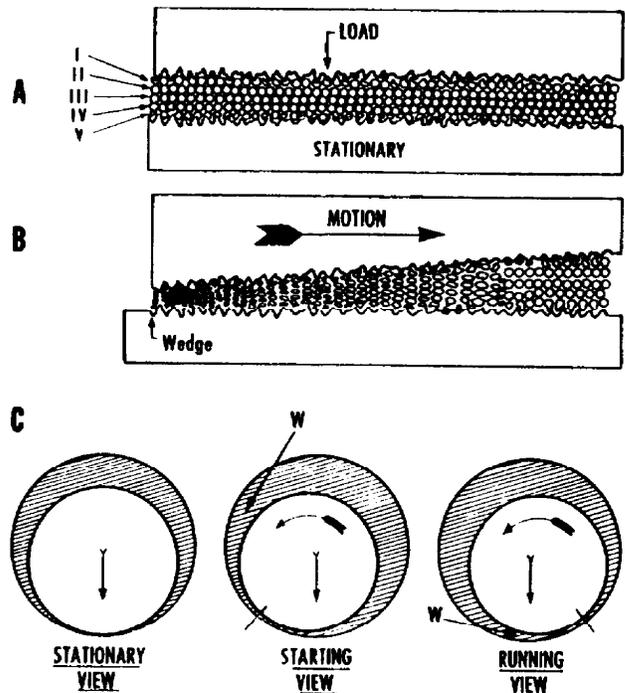
Figure 4-1.—Oil film lubrication.
