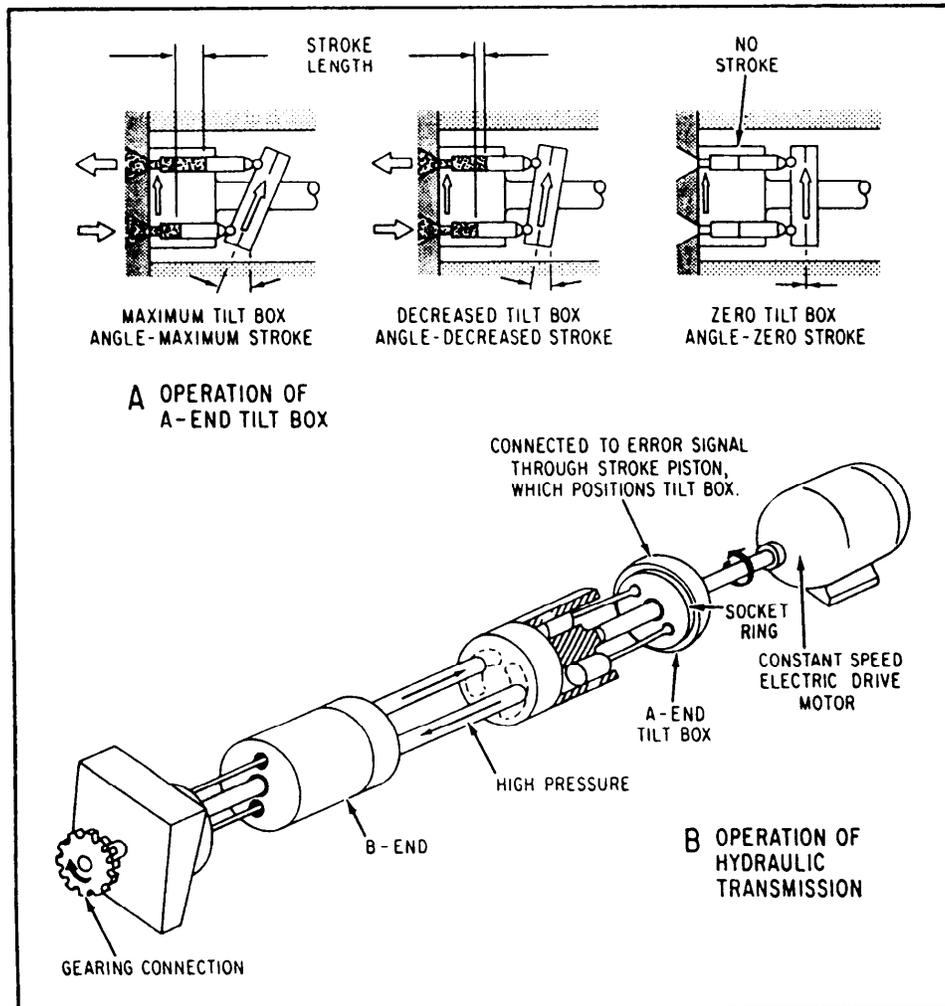
Figure 14-1.—Electrohydraulic speed gear.
