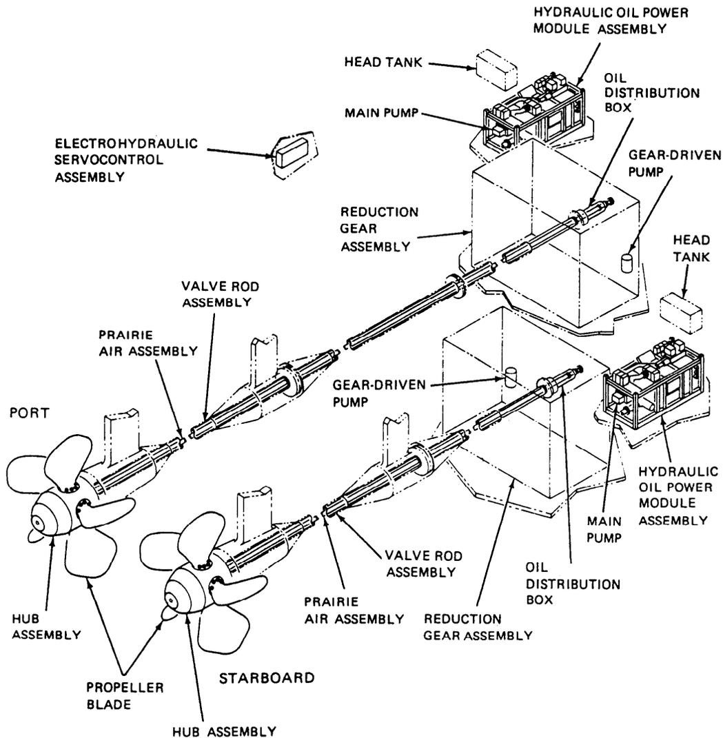
Figure 3-24.—Controllable pitch propeller in DD-963, DD-993, and DD-997 class ship.
