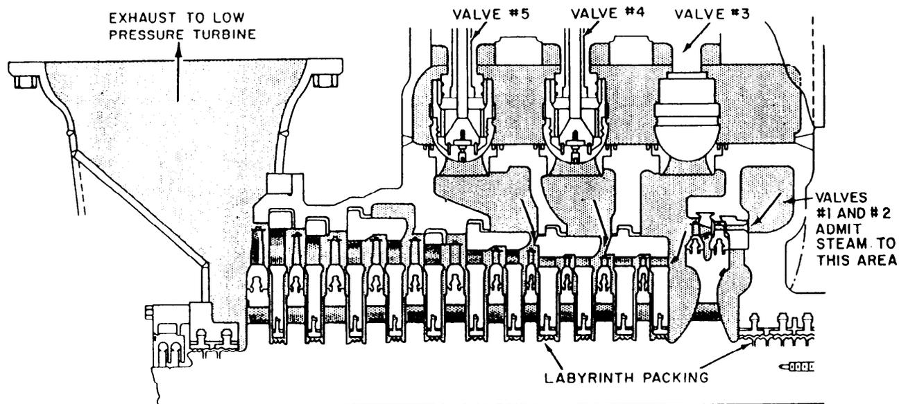
Figure 2-25.—High-pressure turbine showing valve arrangement.
