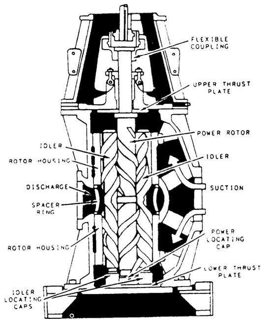
Figure 5-20A.—Triple-screw high-pitch pump.
