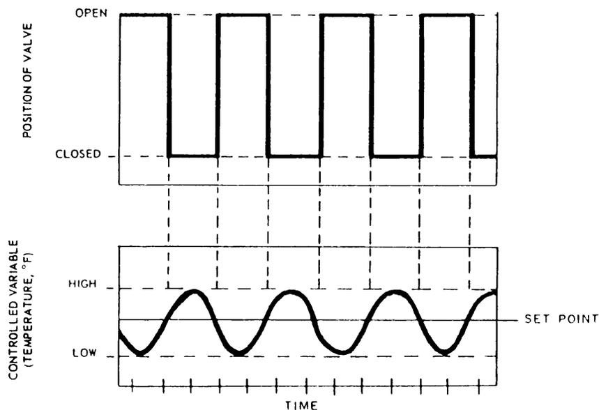
Figure 17-6.—Action of two-position single-point controller : valve position (top) and controlled variable (bottom).
