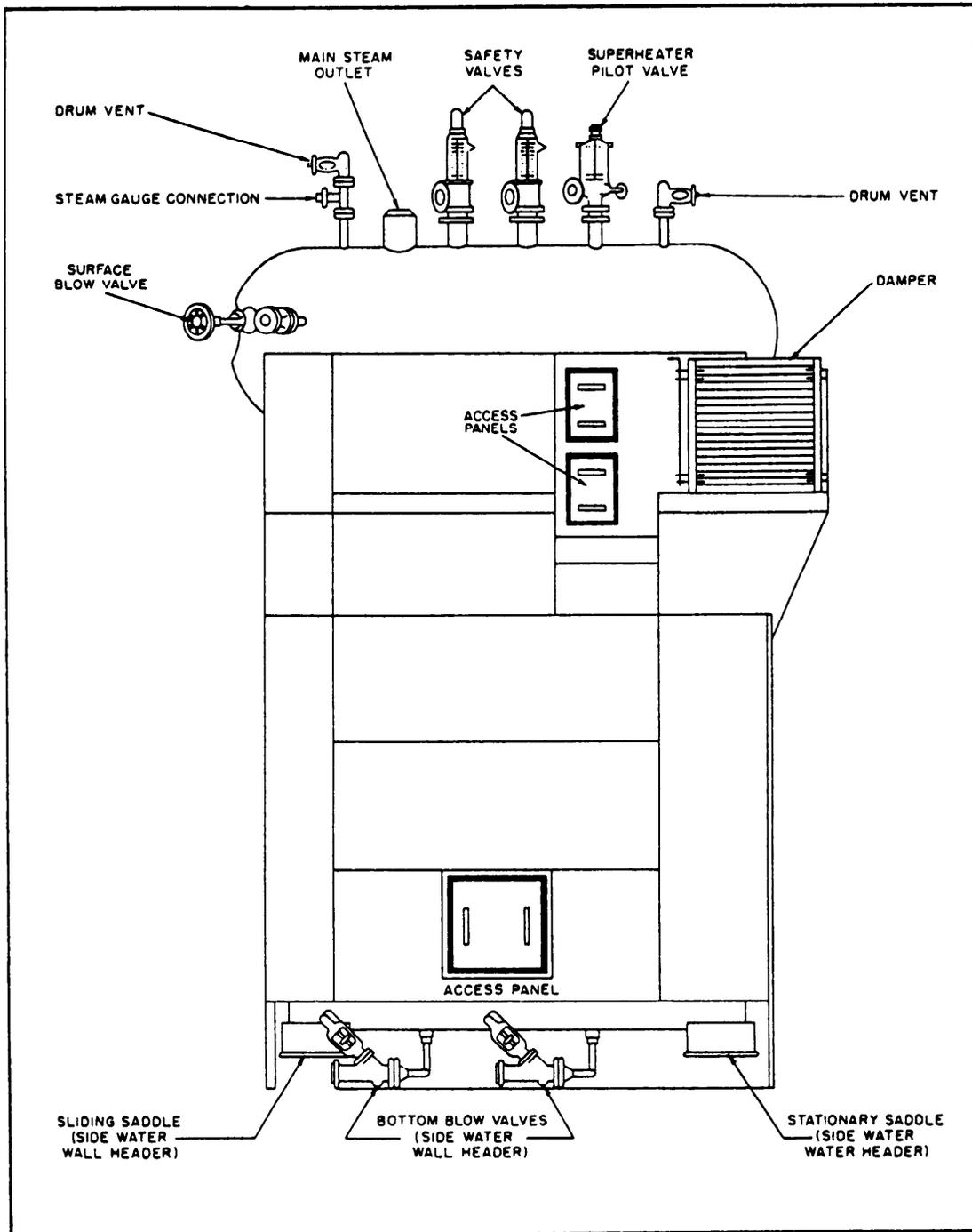
Figure 16-6.—External fittings and connections on a single-furnace boiler (side view).
