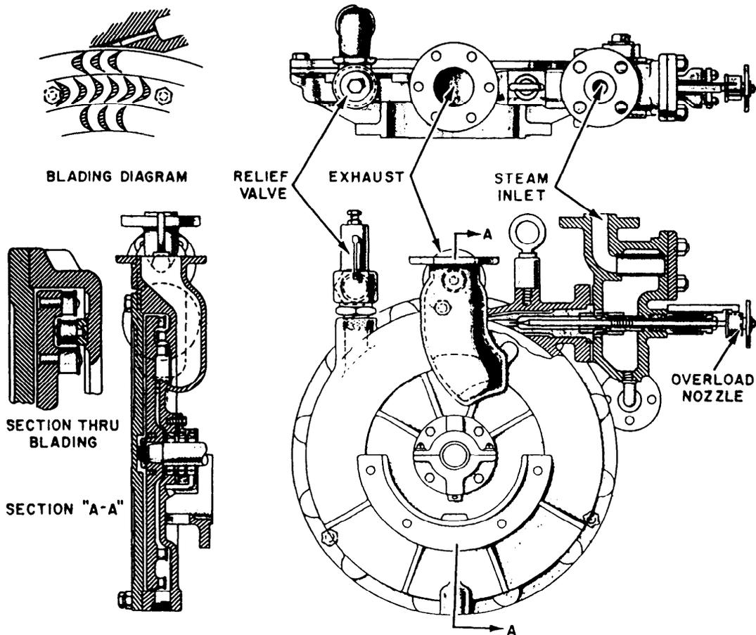
Figure 2-26.—Main lube oil pump turbine.
