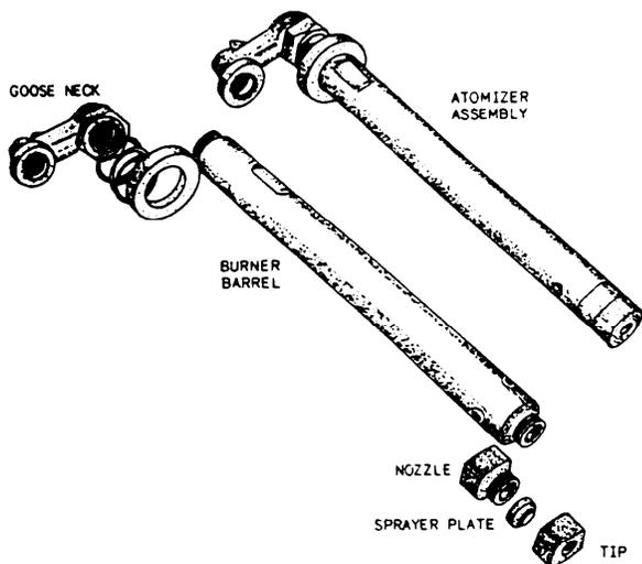
Figure 16-26.—Parts of a straight-through-flow atomizer assembly.
