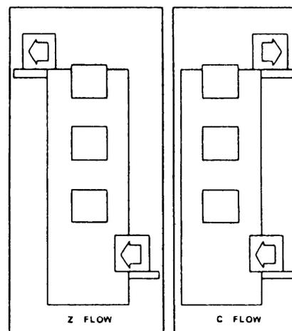
Figure 14-7.—Vertical conveyor, pallet, tray type.
