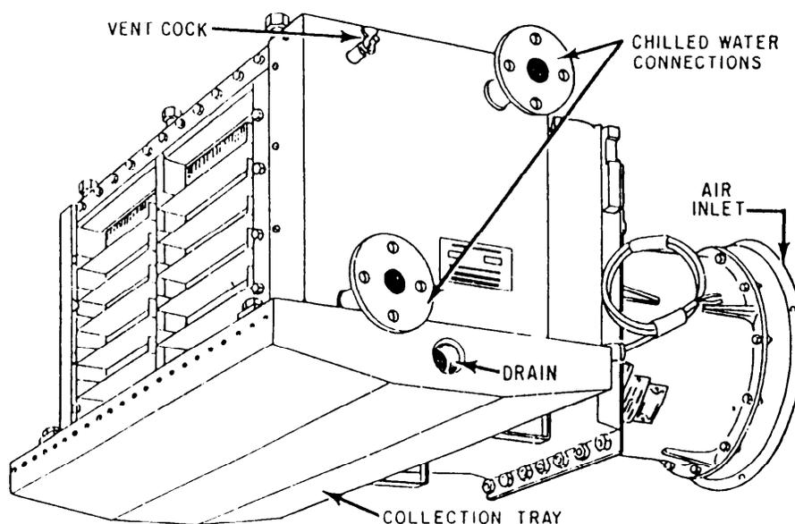
Figure 12-9.—Fan-coil assembly.
