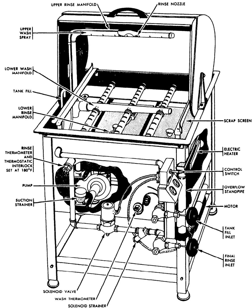
Figure 14-13.—Typical semiautomatic single-tank dishwashing machine.
