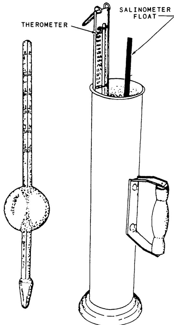
Figure 9-13.—Salinometer and sampling pot.
