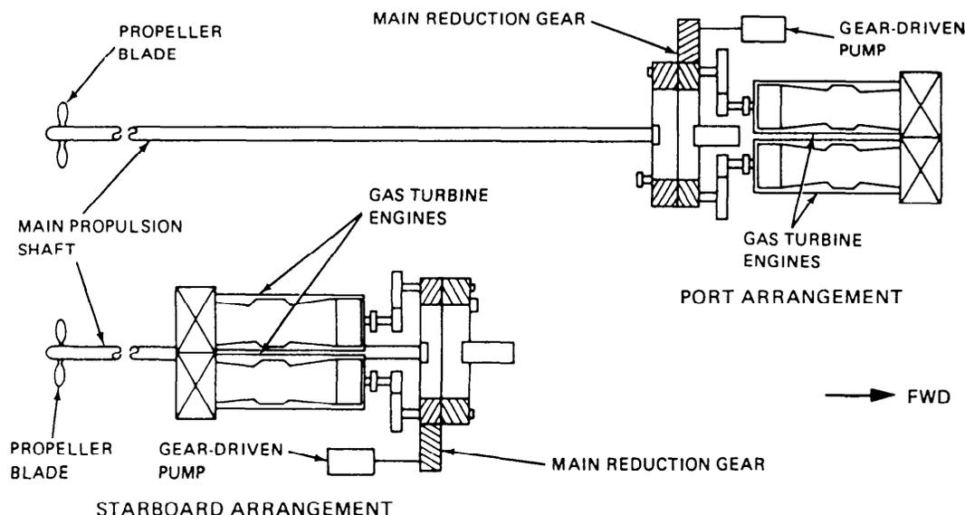
Figure 3-23.—Main propulsion system
