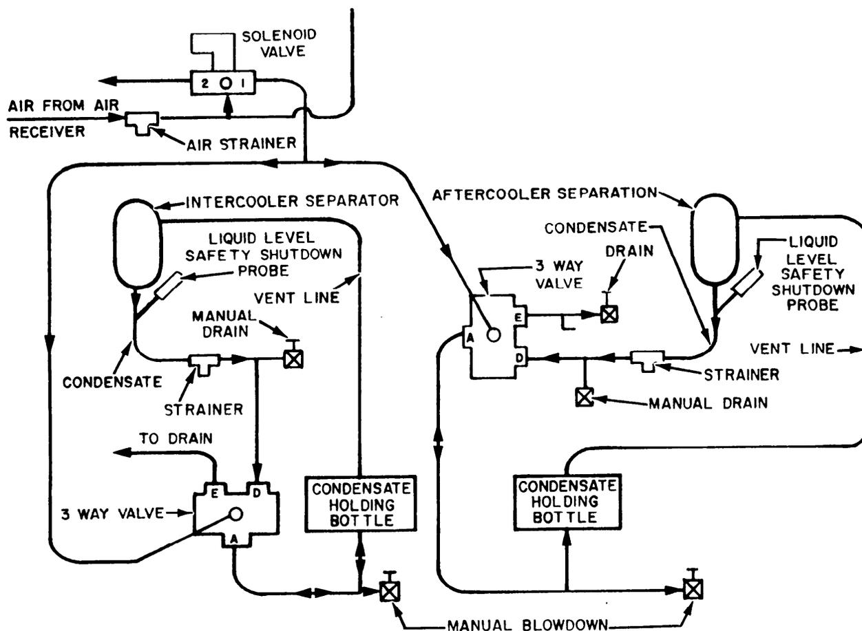
Figure 13-21B.—Condensate drain system.
