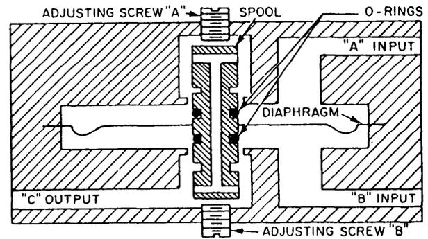
Figure 17-13.—High signal selector.
