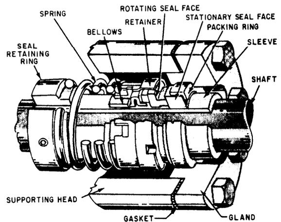
Figure 5-6.—Type-1 mechanical seal.
