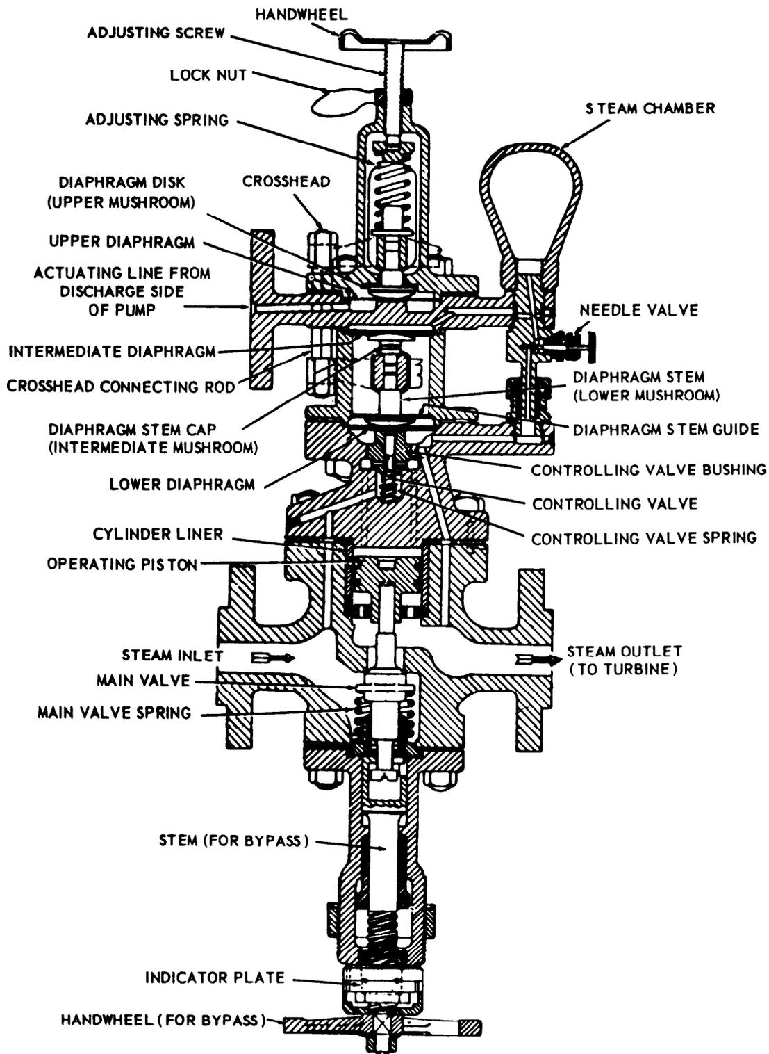
Figure 5-9.—Constant-pressure governor for main feed pump.
