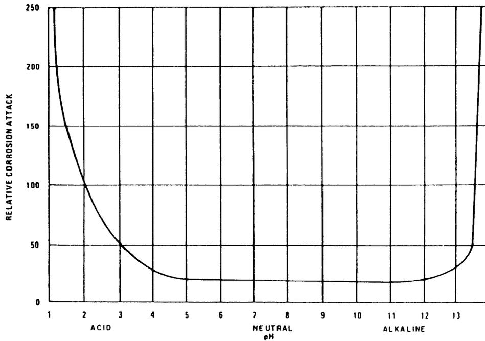
Figure 18-5.—pH effect on boiler metal corrosion.
