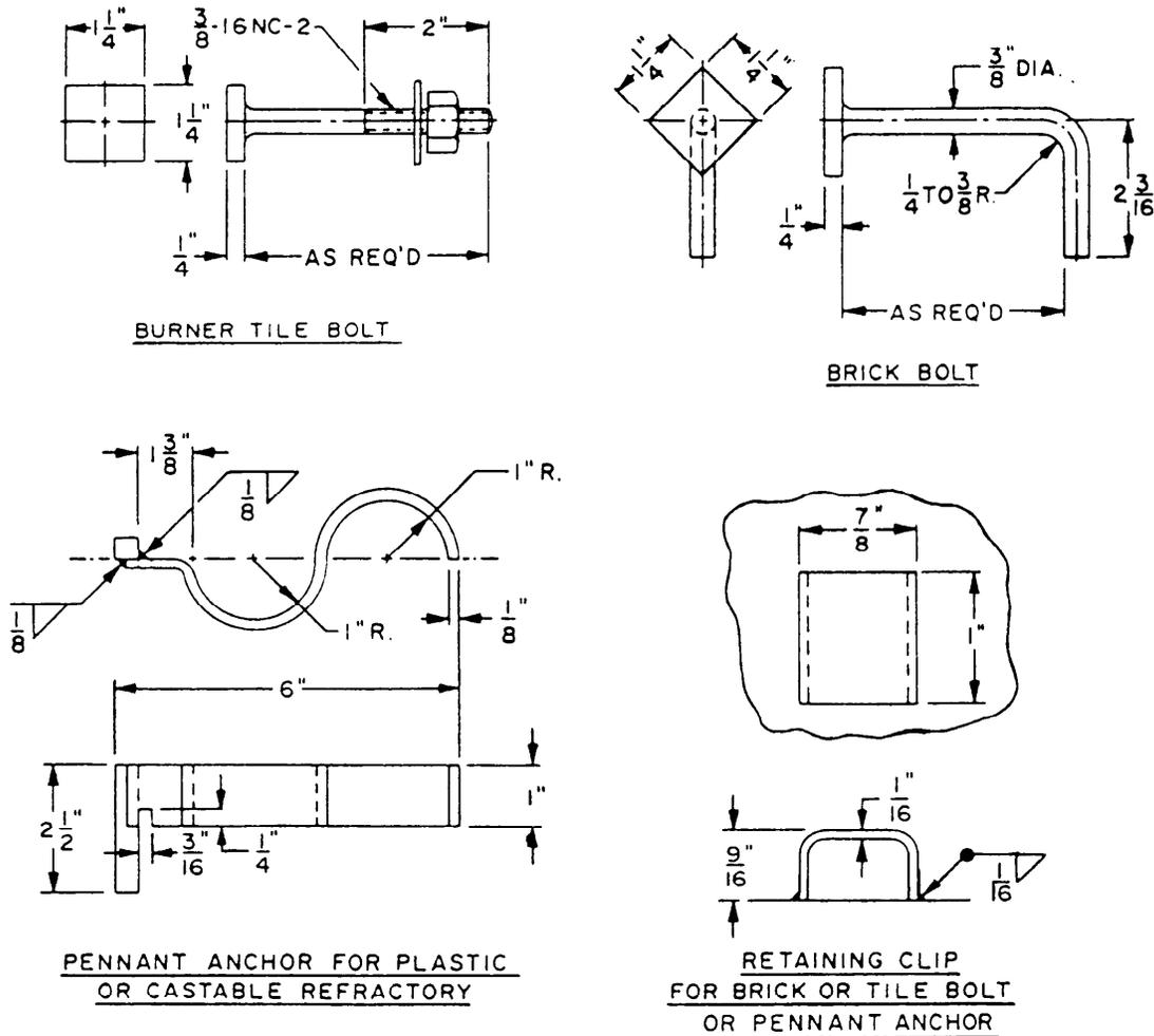
Figure 15-10.—Refractory anchor devices.
