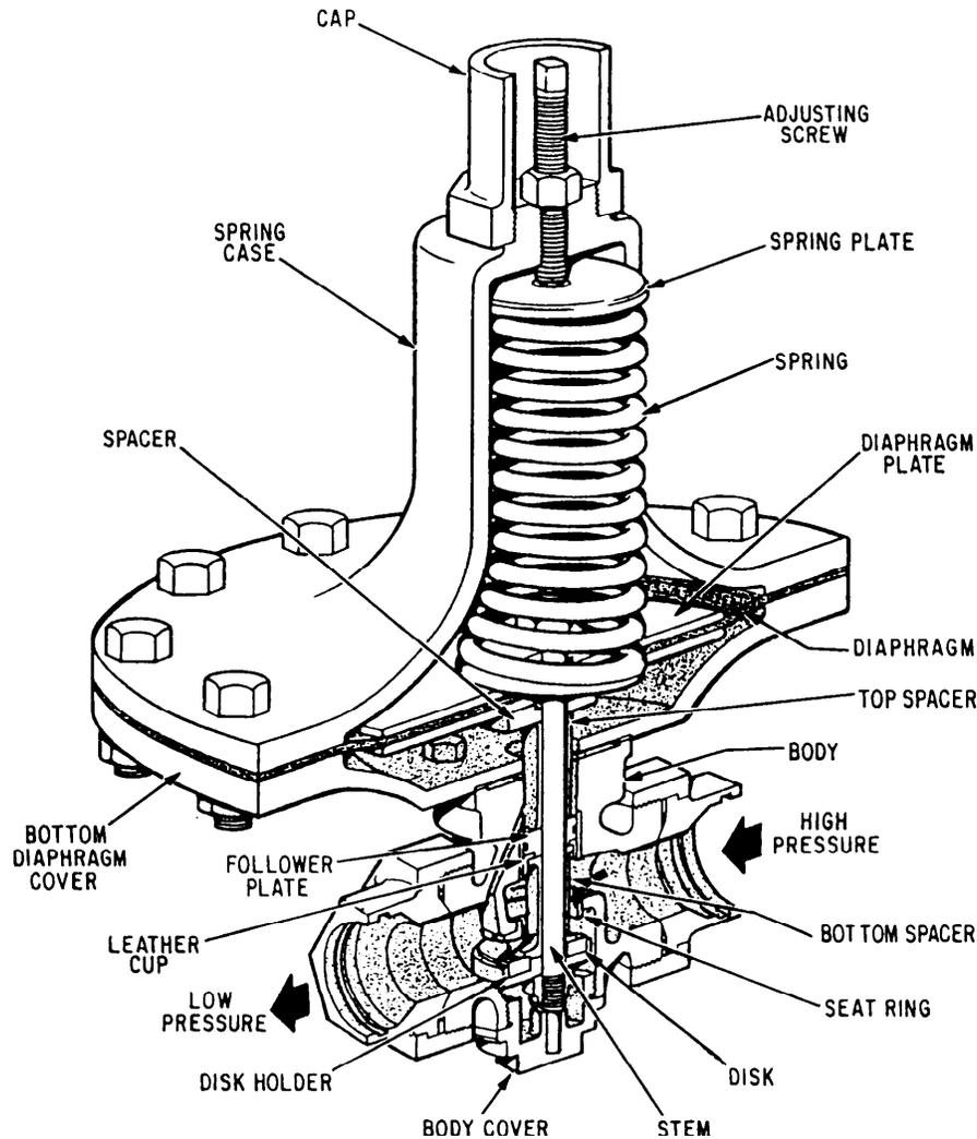
Figure 10-17.—Pressure-reducing (spring-loaded) valve.
