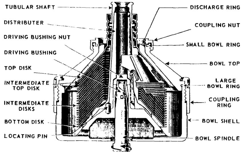
Figure 4-6.—Part of a disk-type purifier bowl.
