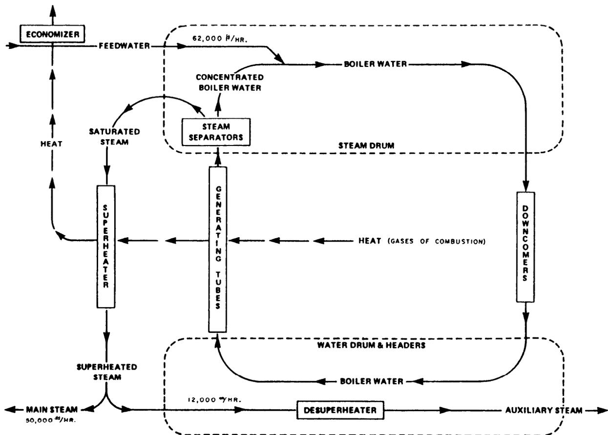
Figure 18-2.—Propulsion boiler water flow.
