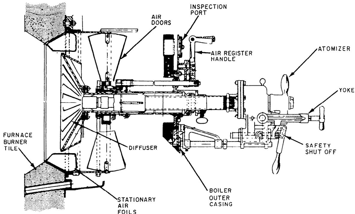
Figure 16-29.—Fuel-oil burner assembly.
