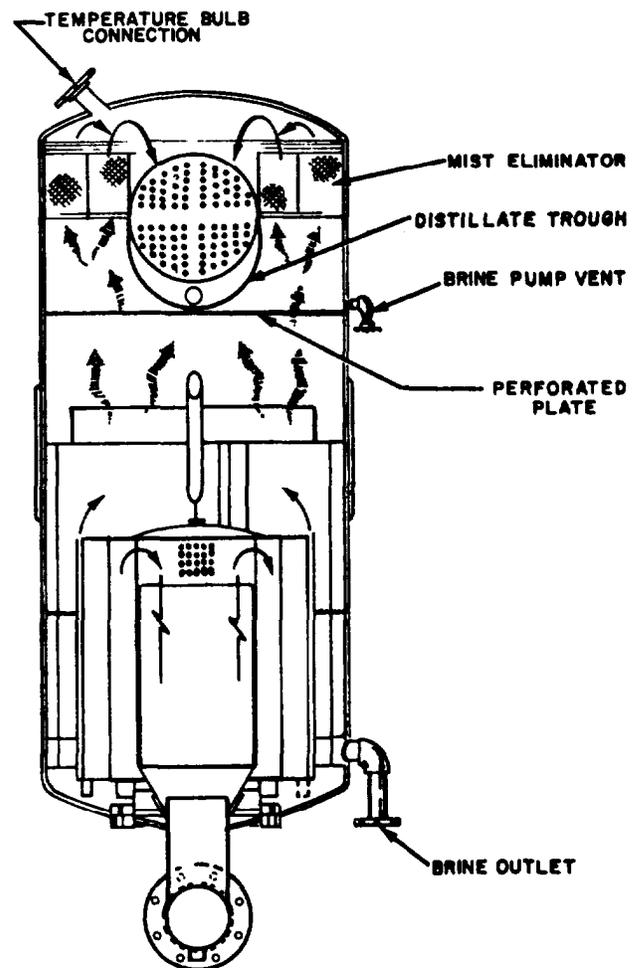
Figure 9-9.—Side view (cutaway) of vertical basket distilling plant.
