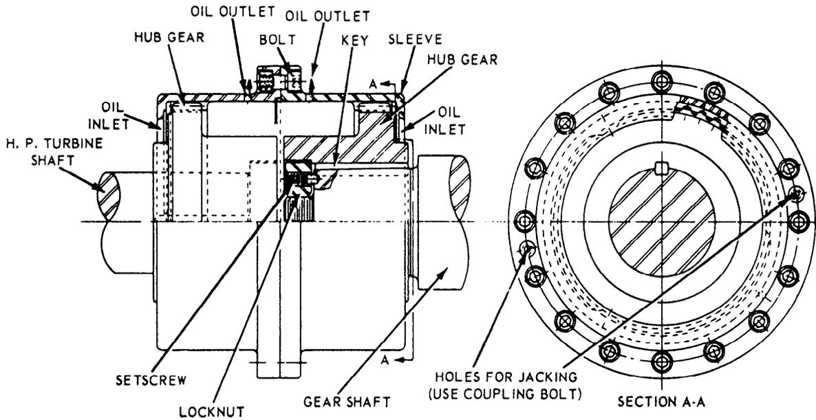
Figure 3-7.—Another gear-type flexible coupling.
