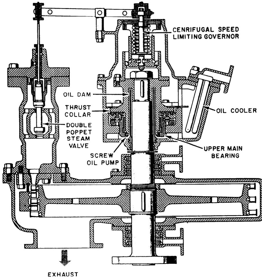
Figure 2-27.—Main condenser circulating pump turbine.
