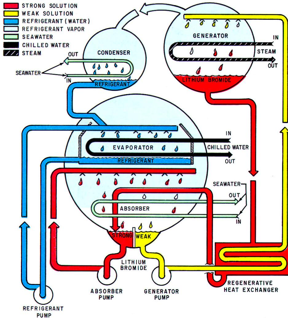
Figure 12-8.—Basic absorption cycle.
