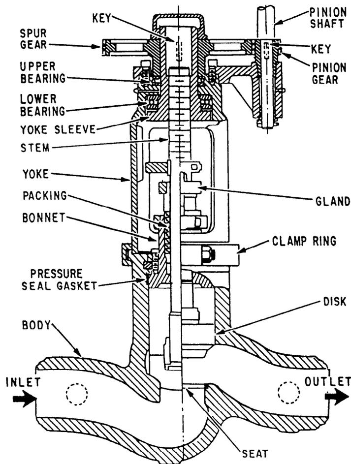
Figure 10-10.—Gear-operated globe stop valve.
