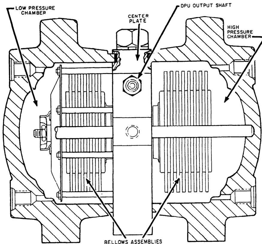
**Figure 16-20.—Differential Pressure-Sensing Unit (DPU).**
