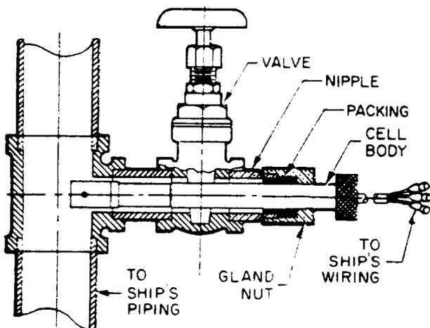
Figure 9-11.—Salinity cell installation.
