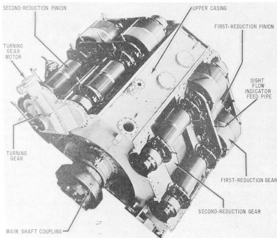
Figure 3-2.—Typical destroyer-type propulsion gear.
