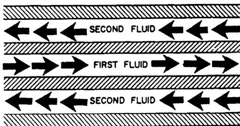
Figure 6-2.—Counterflow in a heat exchanger.
