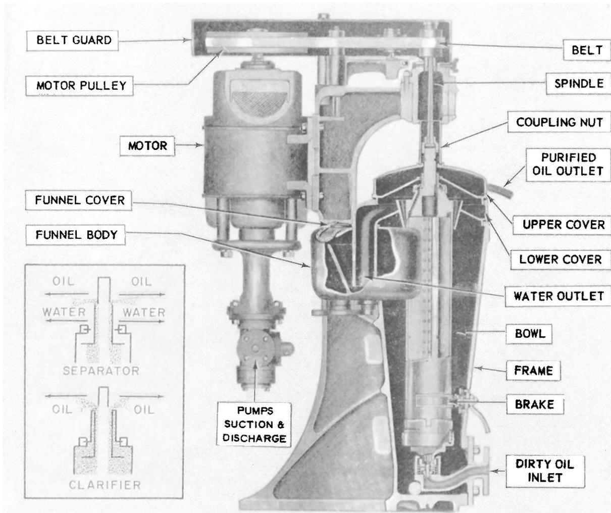
Figure 4-8.—Tubular-type centrifugal purifier.
