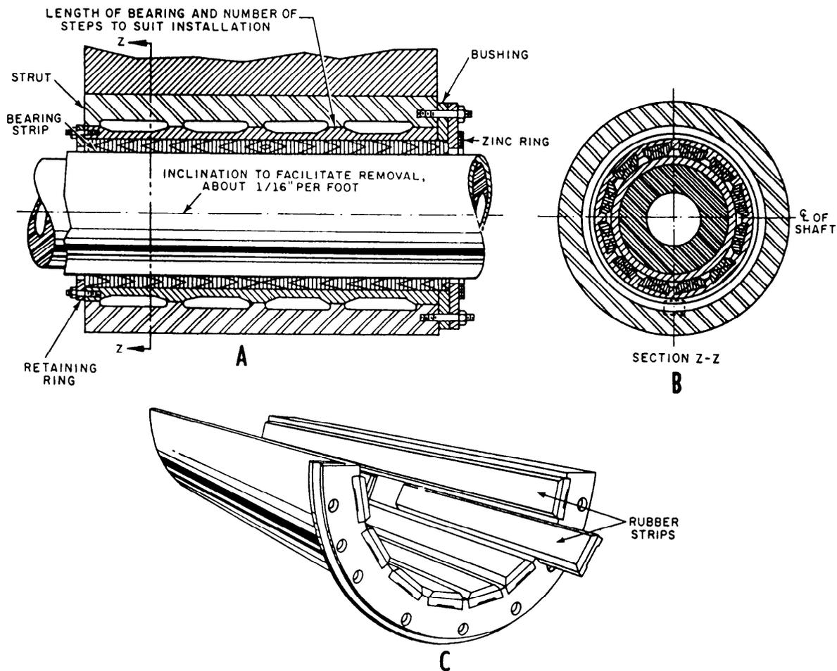
Figure 3-21.—Details of a strut bearing. A. Longitudinal view. B. Cross-sectional View. C. Rubber stripping in a bearing.
