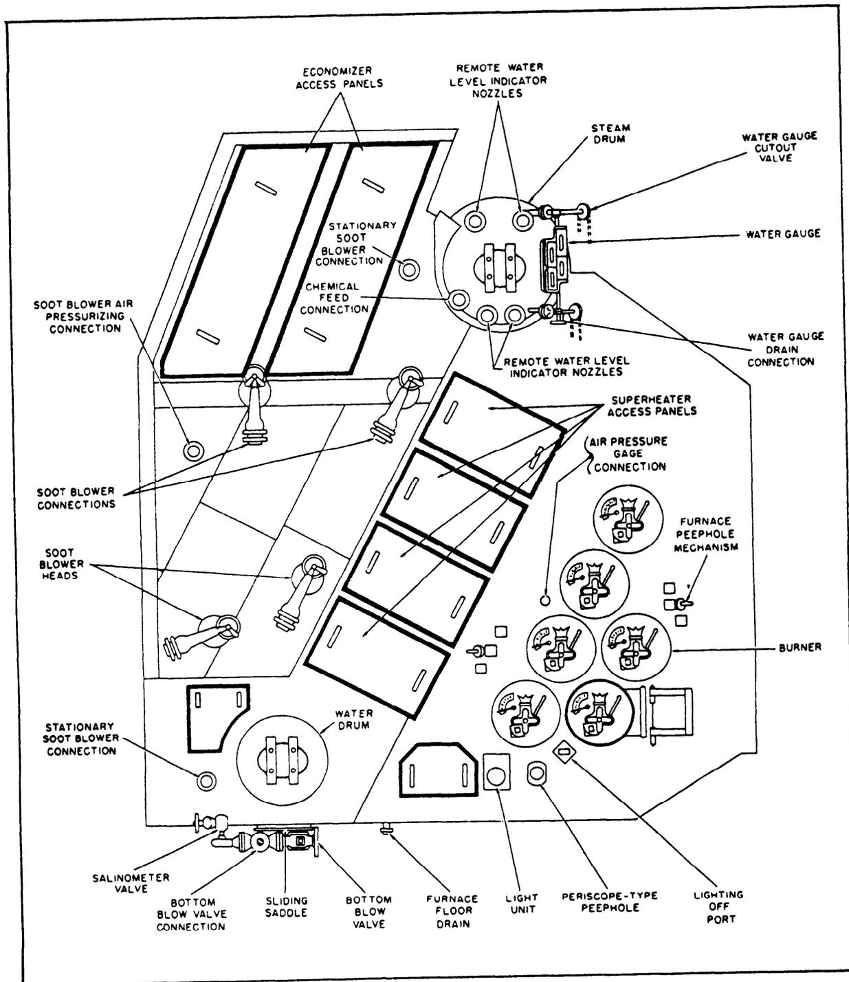
Figure 16-5.—External fittings and connections on a single-furnace boiler (front view).
