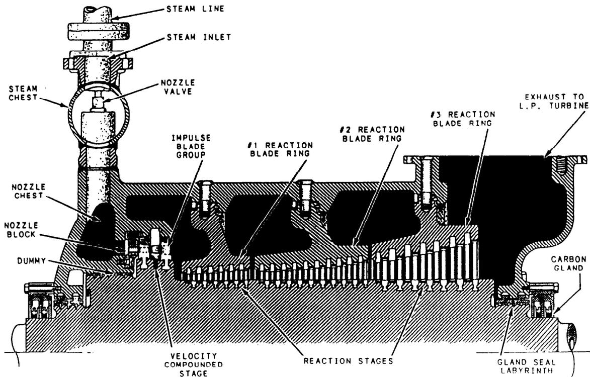
Figure 2-12.—Combination impulse and reaction turbine.
