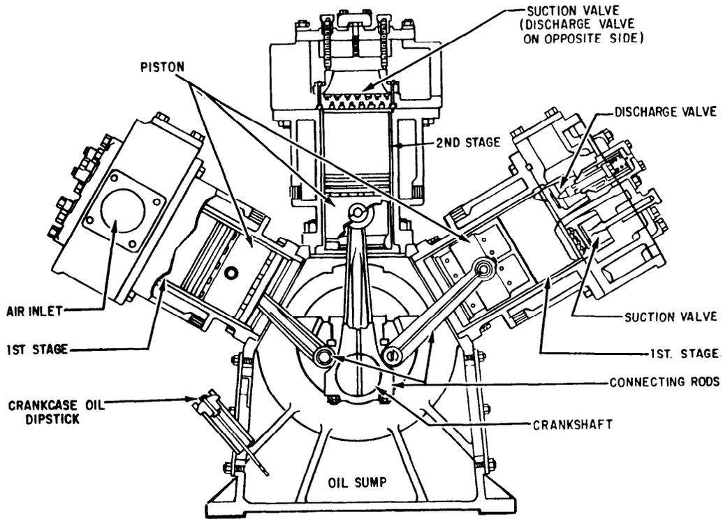
Figure 13-2.—Low-pressure reciprocating air compressor, vertical W configuration.
