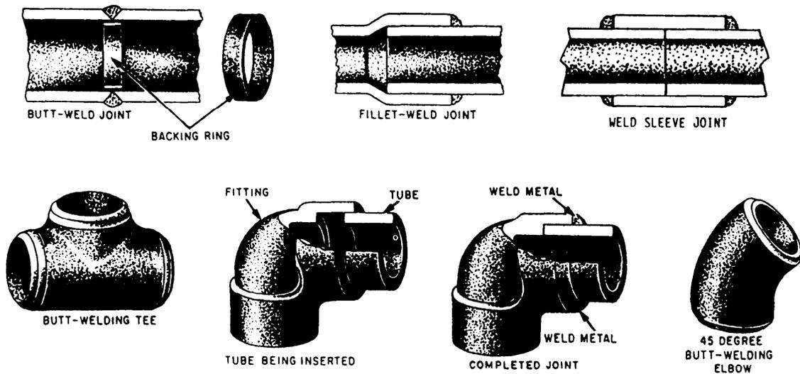
Figure 10-3.—Various types of welded joints.
