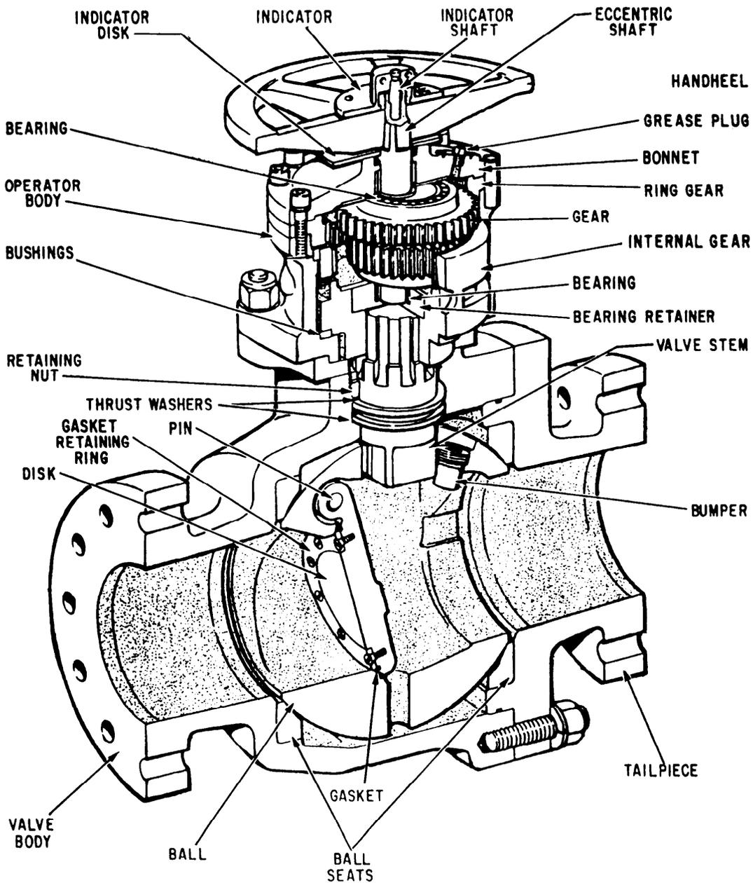
Figure 10-15.—Typical ball stop swing-check valve for seawater service.
