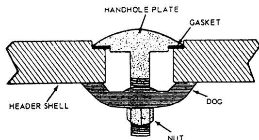
Figure 15-3.—Header handhole and handhole plate.
