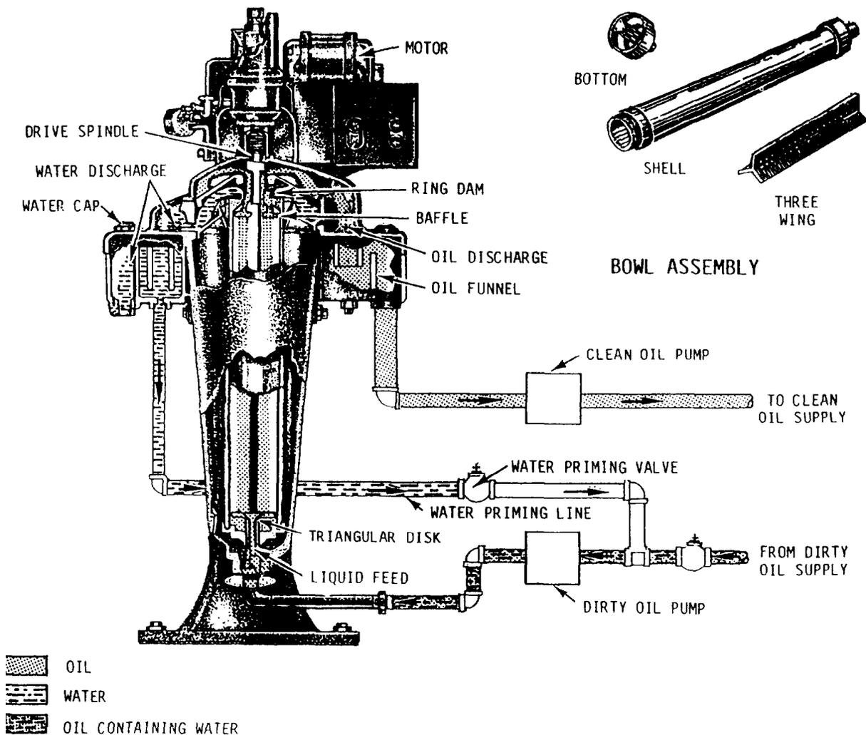
Figure 4-10.—Path of oil through the bowl-type purifier.
