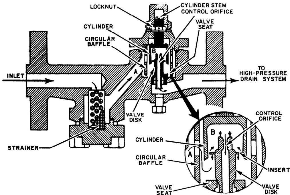
Figure 10-28.—Impulse steam trap.
