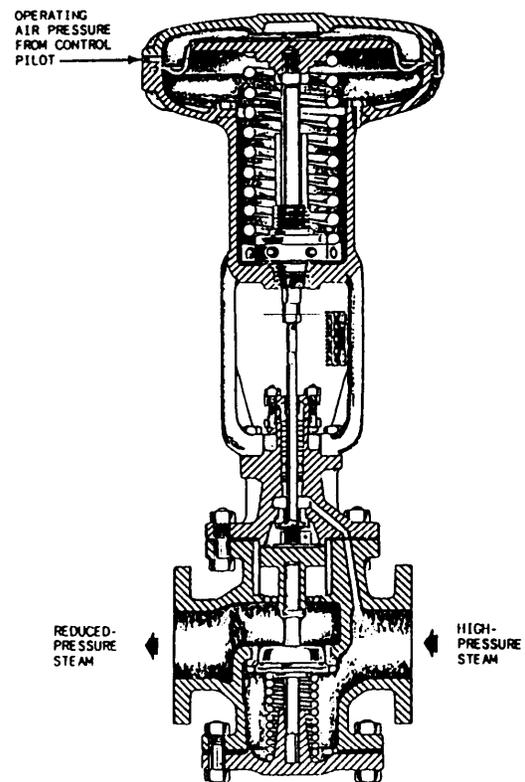
Figure 10-23.—Diaphragm control valve (upward seating).
