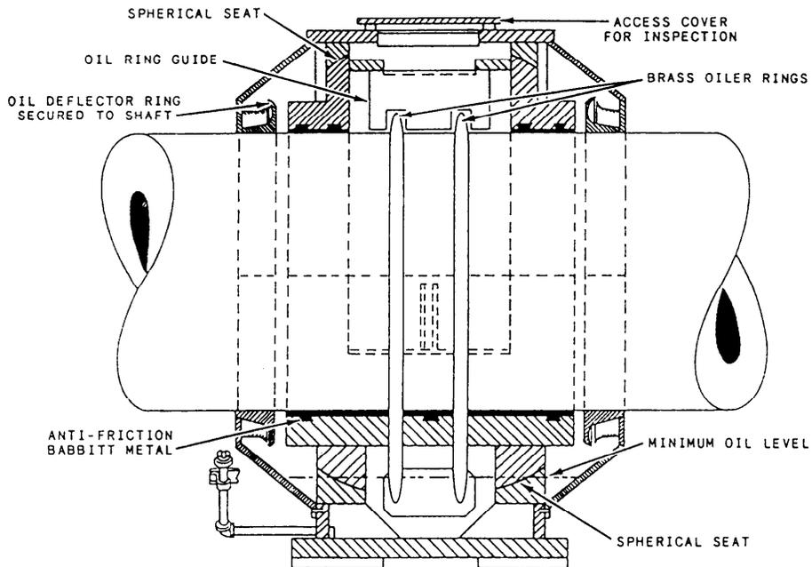
Figure 3-15.—Main line shaft bearing (ring oiled).
