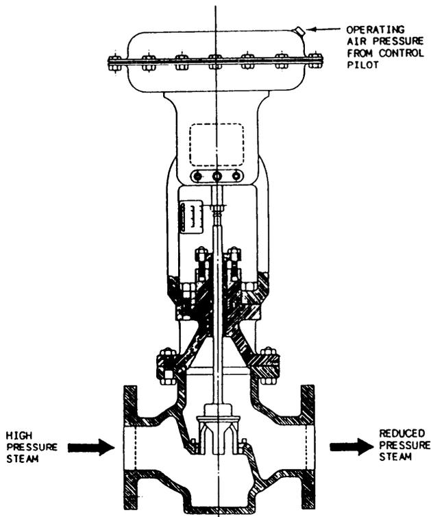
Figure 10-22.—Diaphragm control valve (downward seating).
