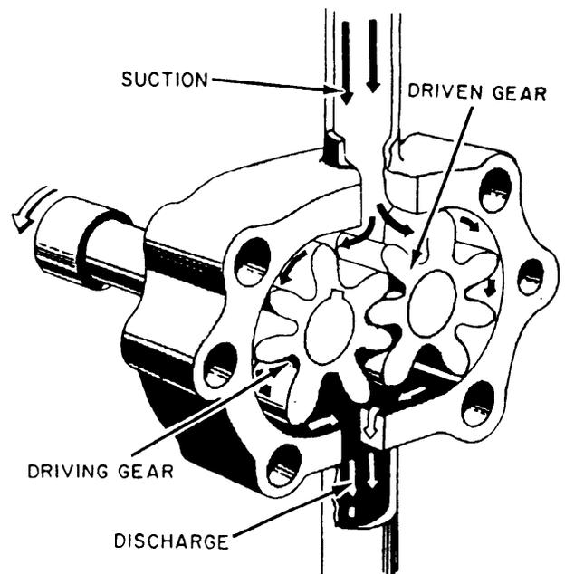
Figure 5-16.—Simple gear rotary pump.
