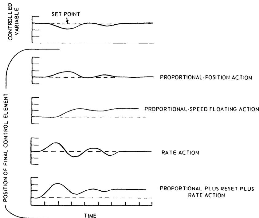
Figure 17-9.—Proportional plus reset plus rate action.
