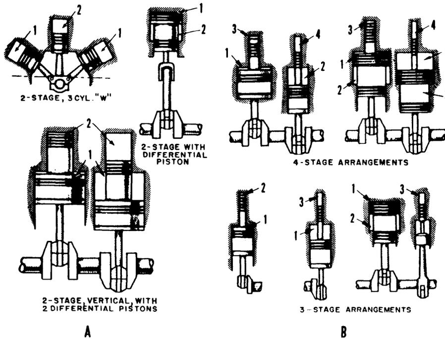
Figure 13-3.—Air compressor cylinder arrangements: (A) Low- and medium-pressure compressors; (B) High-pressure compressor.
