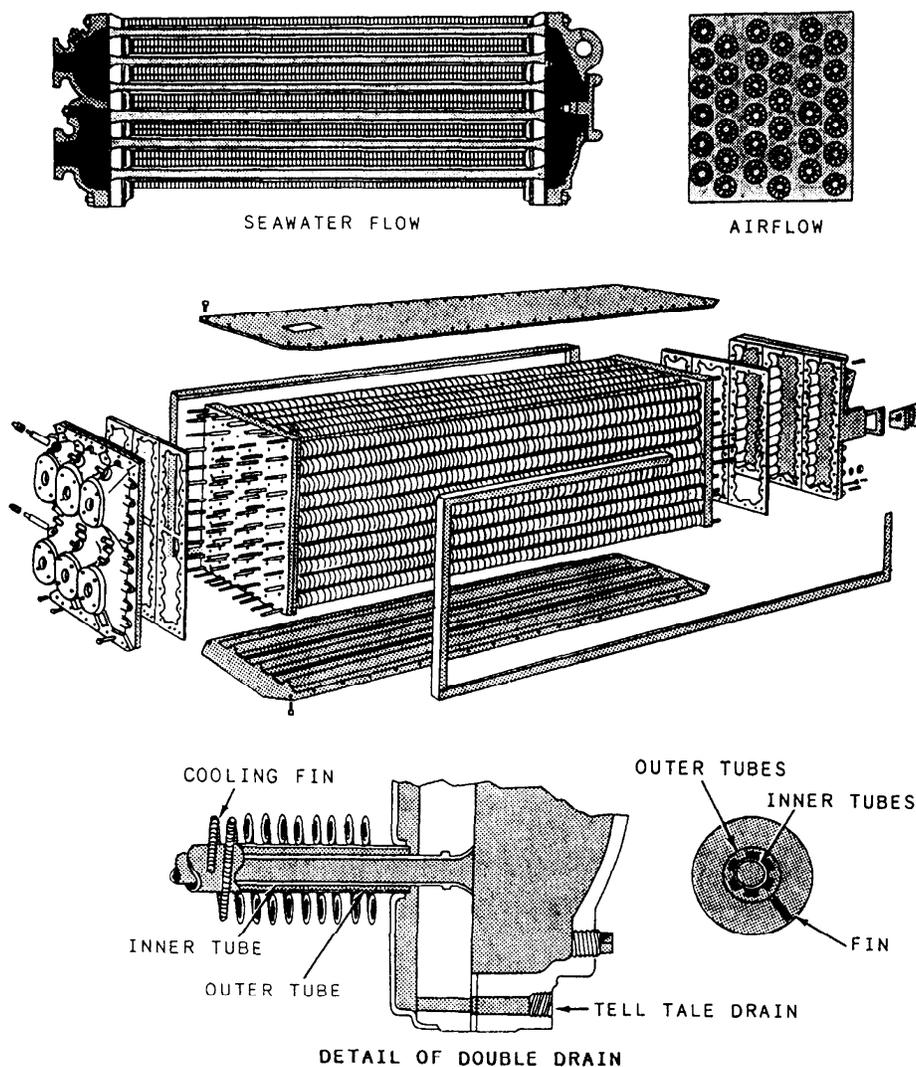
Figure 6-12.—Air cooler for a motor generator.
