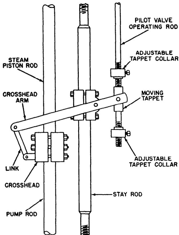
Figure 5-13.—Valve operating assembly.
