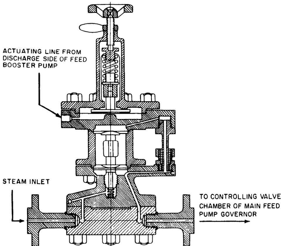
Figure 5-11.—Auxiliary pilot valve for automatic shutdown device.
