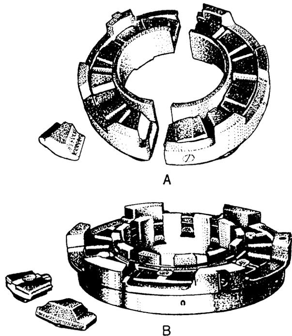
Figure 3-13.—Pivoted-shoe thrust bearing.
