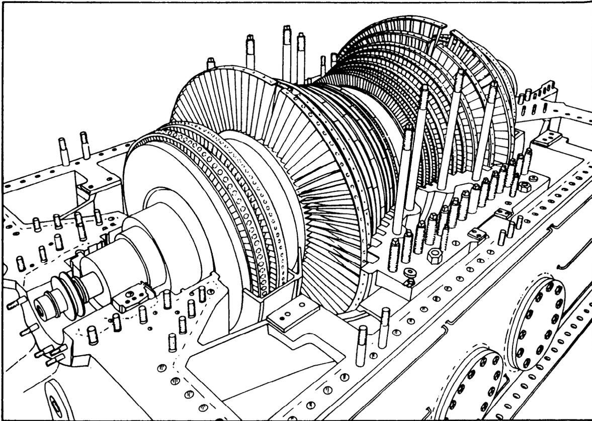
Figure 2-23.—L. P. turbine cylinder base with rotor installed, viewed from thrust end.
