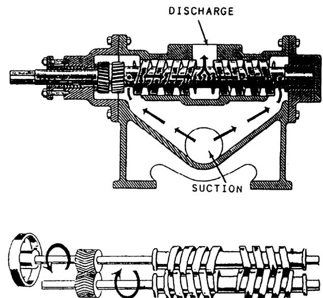
Figure 5-20.—Positive displacement, double-screw, low-pitch pump.
