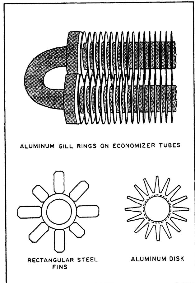
Figure 15-9.—Three types of metal projections used on economizer.
