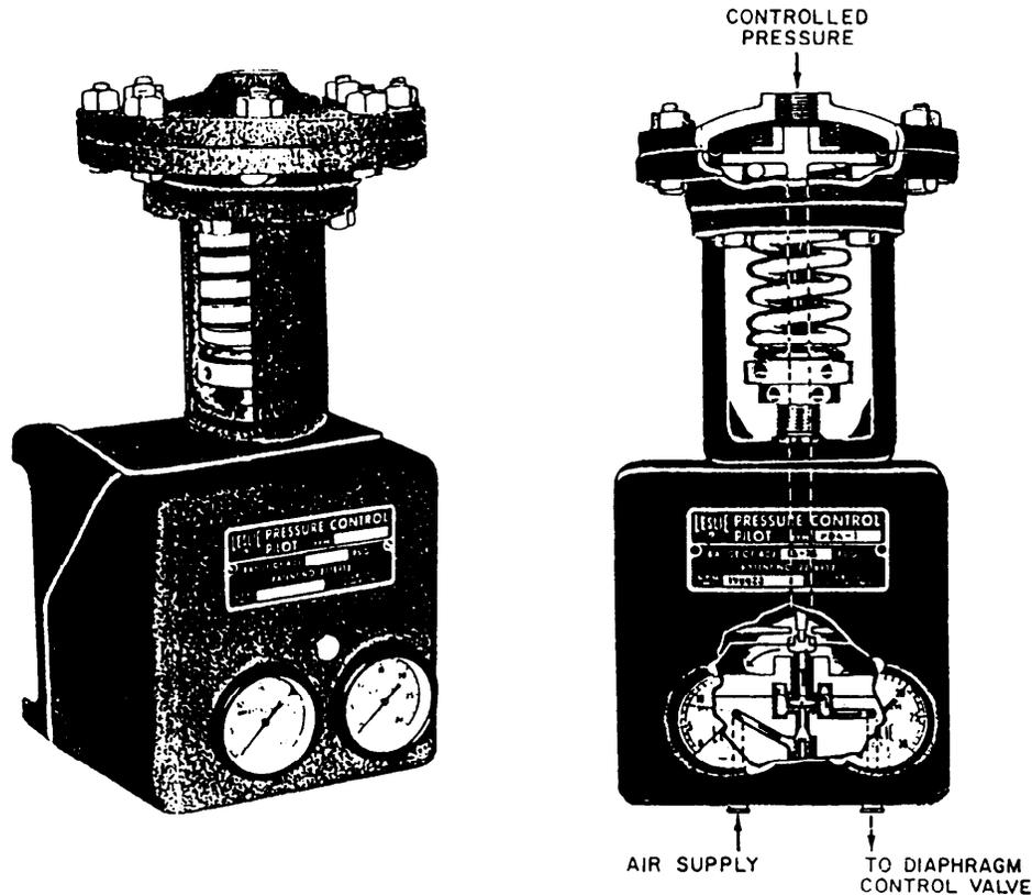
Figure 10-21.—Air-operated control pilot.
