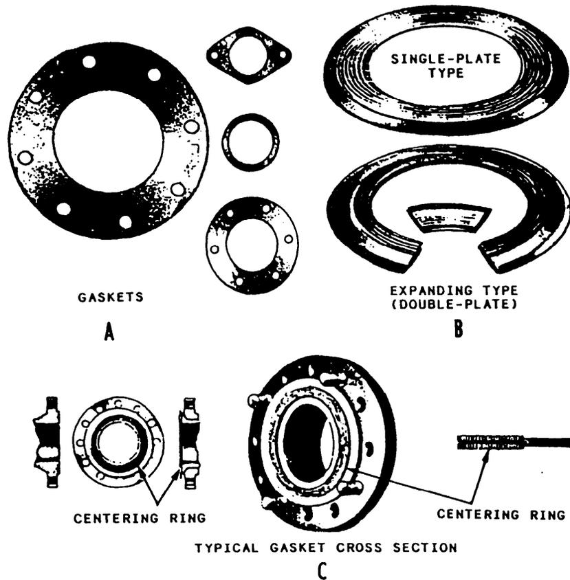
Figure 10-36.—Fixed joint gaskets. A. Sheet asbestos gaskets. B. Serrated-face metal gasket. C. Spiral-wound metallic asbestos gasket.
