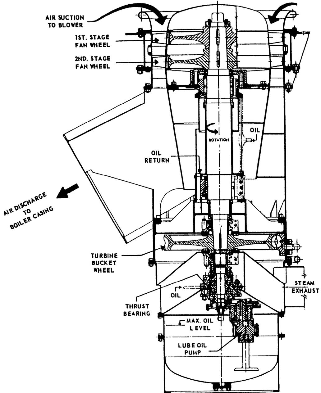
Figure 5-26.—Sectional view of a two-stage vertical propeller-type blower.
