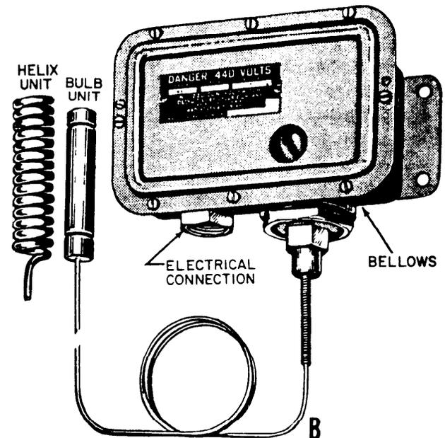
Figure 11-14.—Solenoid valve and thermostatic control switch.
