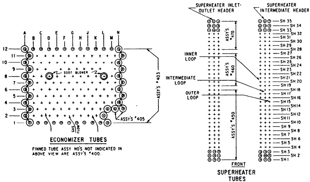
Figure 15-5.—Part of a boiler tube renewal sheet for a single-furnace boiler, showing tube identification.
