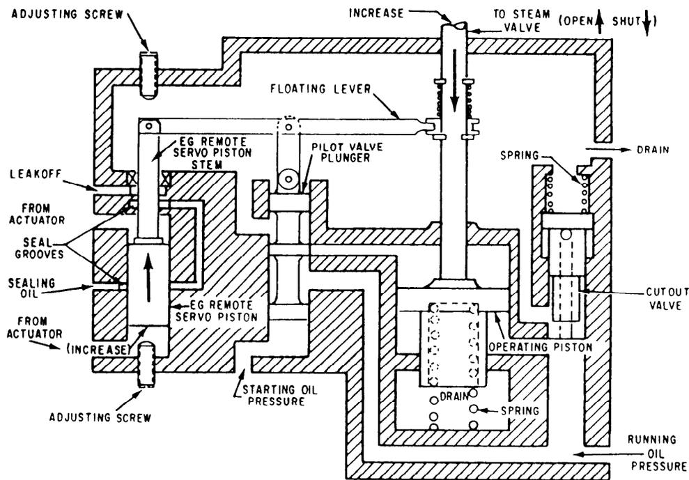
Figure 2-32.—Mechanical diagram of hydraulic valve operator.
