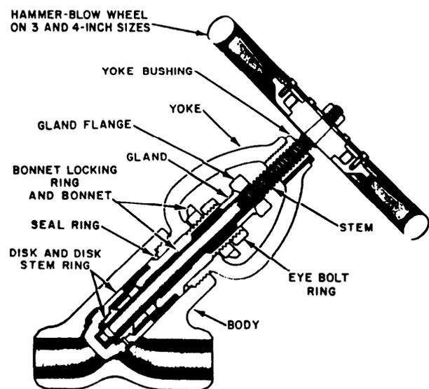
Figure 10-9.—1500-pound pressure seal bonnet globe valve.
