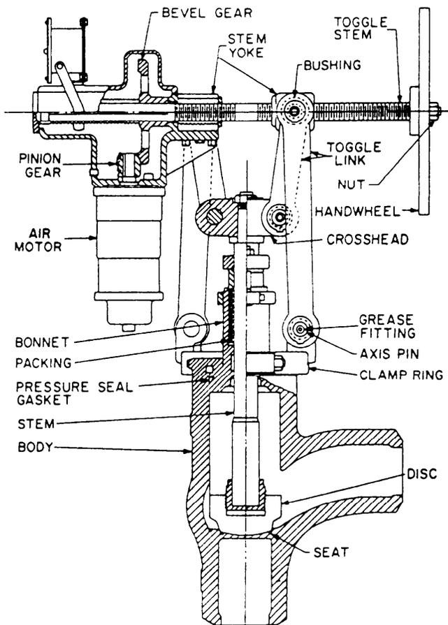
Figure 16-11.—Cross section of motor-operated gauge valve (main steam stop).
