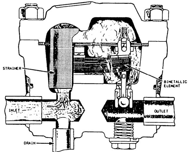
Figure 10-29.—Bimetallic steam trap.
