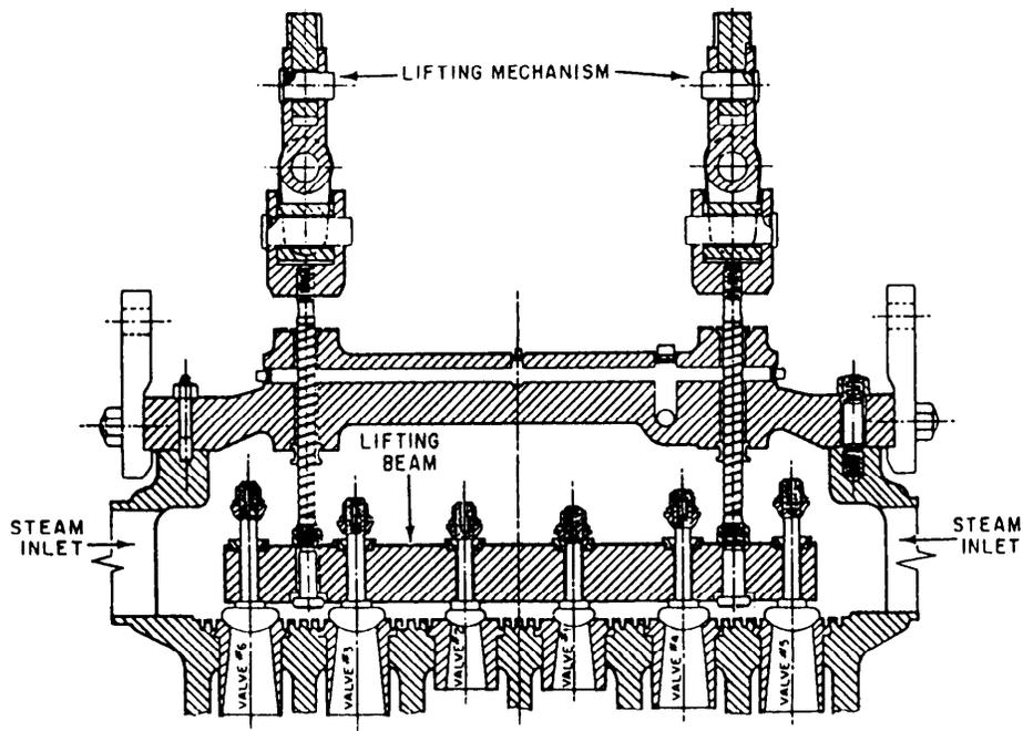
Figure 2-24.—Arrangement of nozzle control valves.
