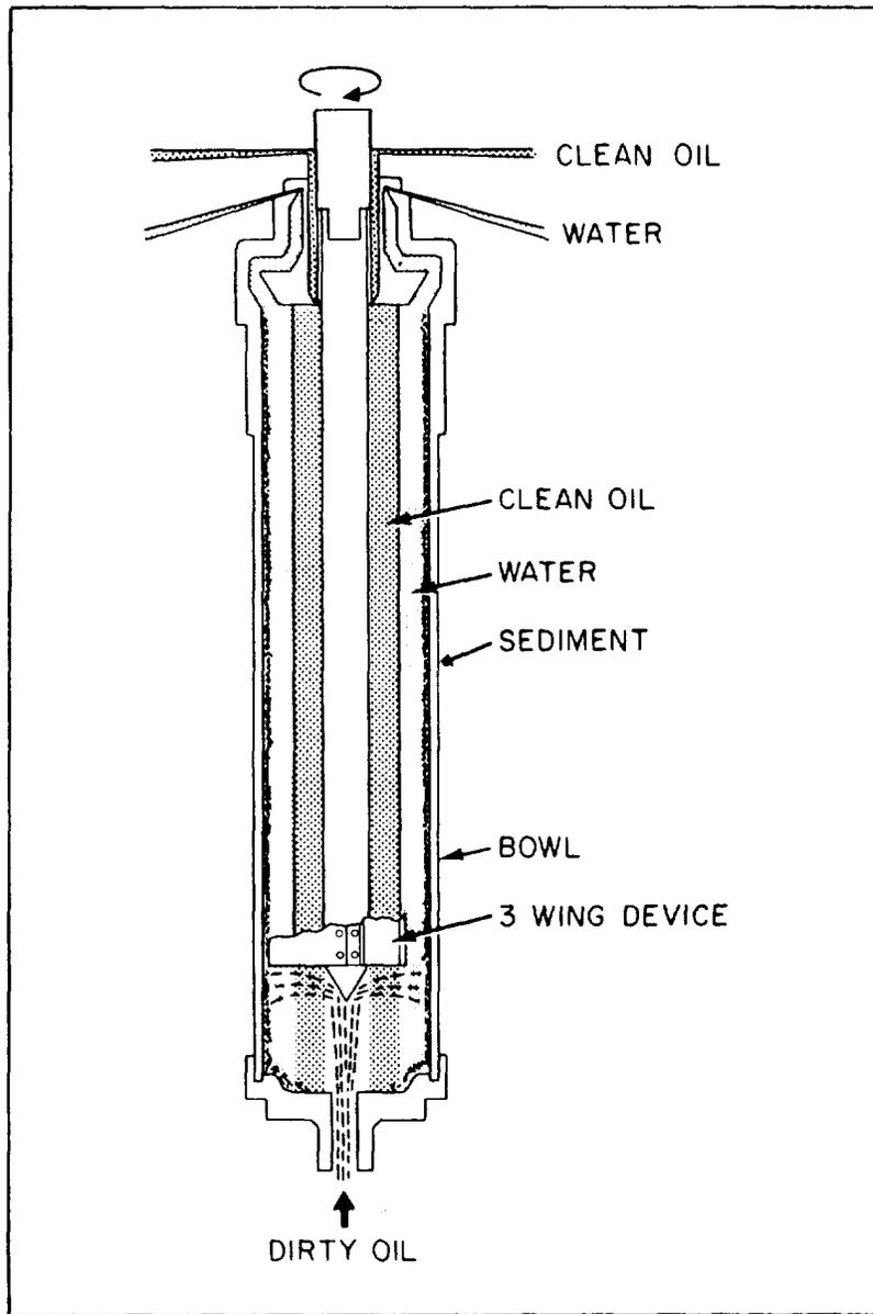
Figure 4-9.—Principles of a centrifugal purifier.
