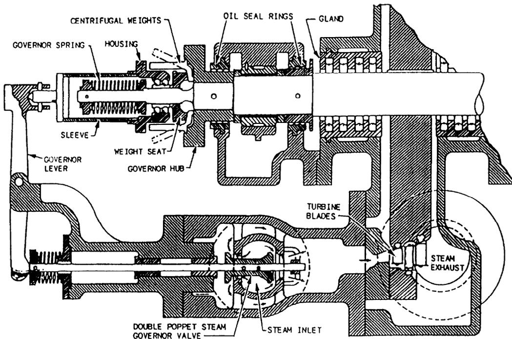
Figure 2-30.—Speed-limiting governor, main feed pump.
