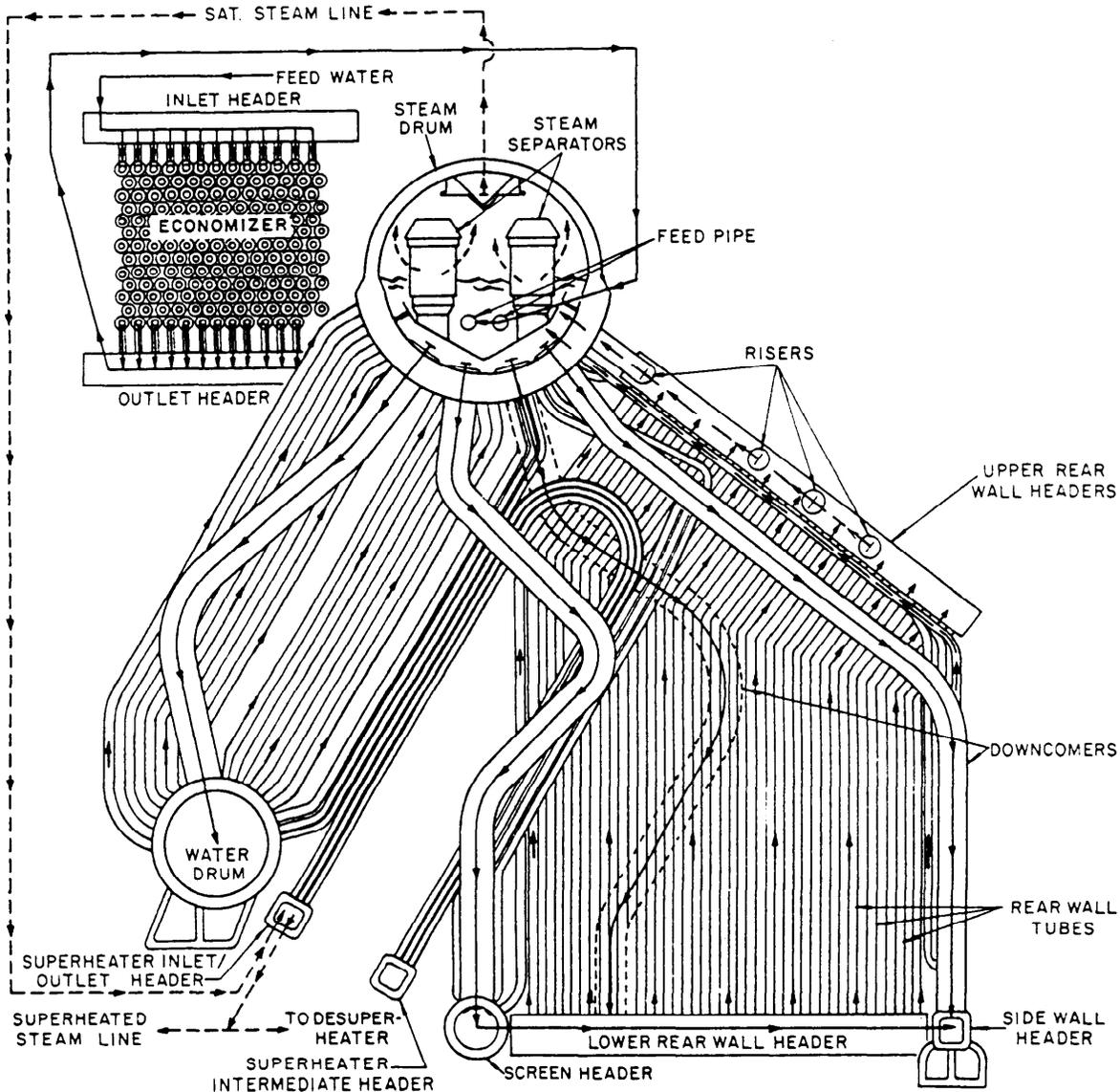
Figure 15-13.—Boiler water and steam flow.
