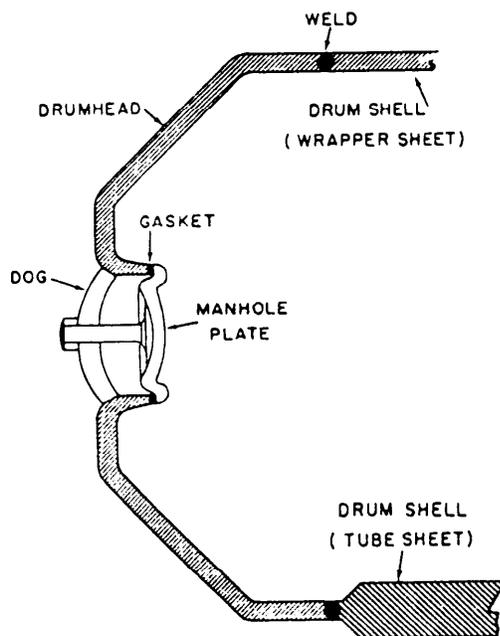
Figure 15-2.—Drumhead secured to steam drum.
