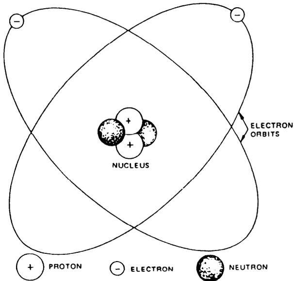
Figure 18-3.—Schematic diagram of a simple atom.
