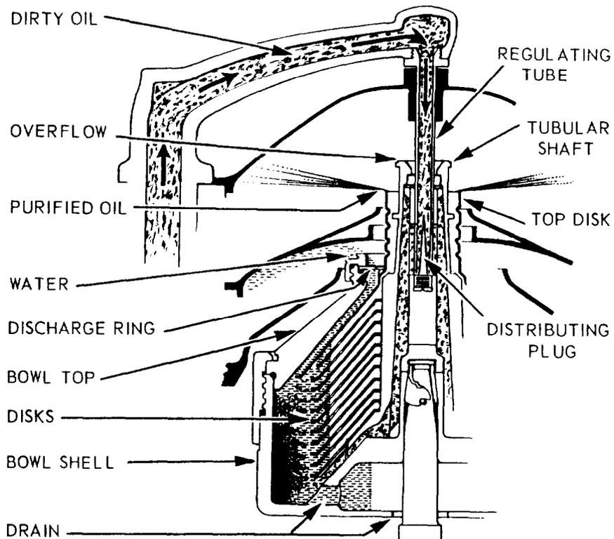
Figure 4-7.—Path of oil through disk-type purifier.
