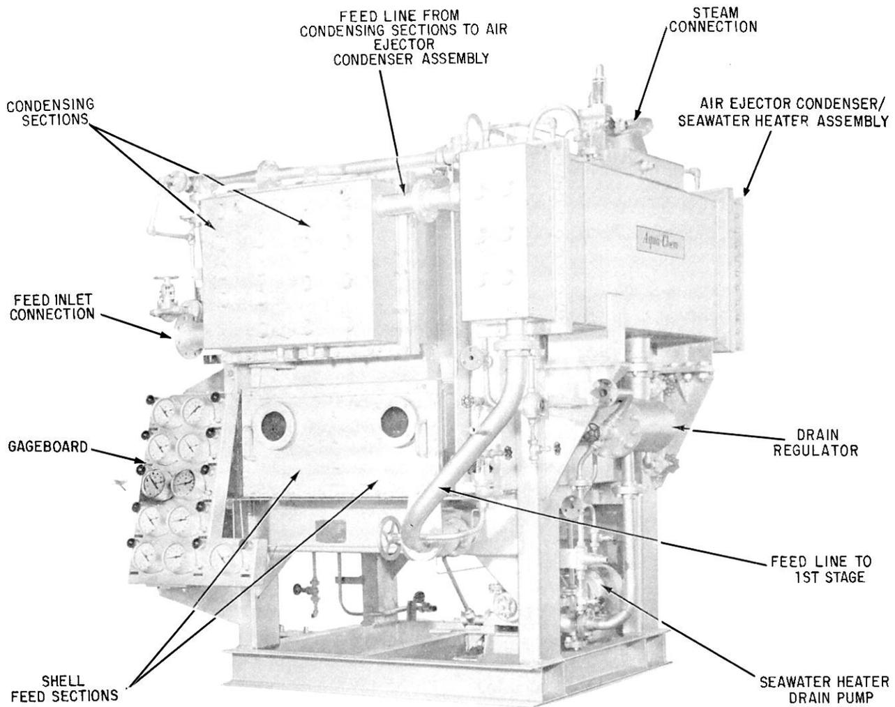
Figure 9-4.—Two-stage, 12,000 gpd flash-type distilling plant.
