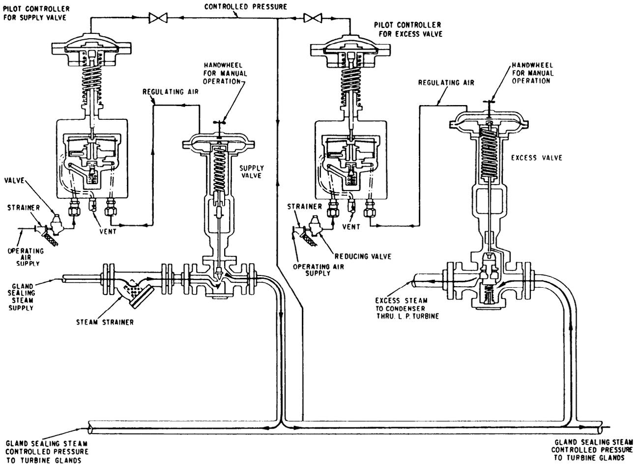
Figure 2-19.—Gland seal regulator mechanism.
