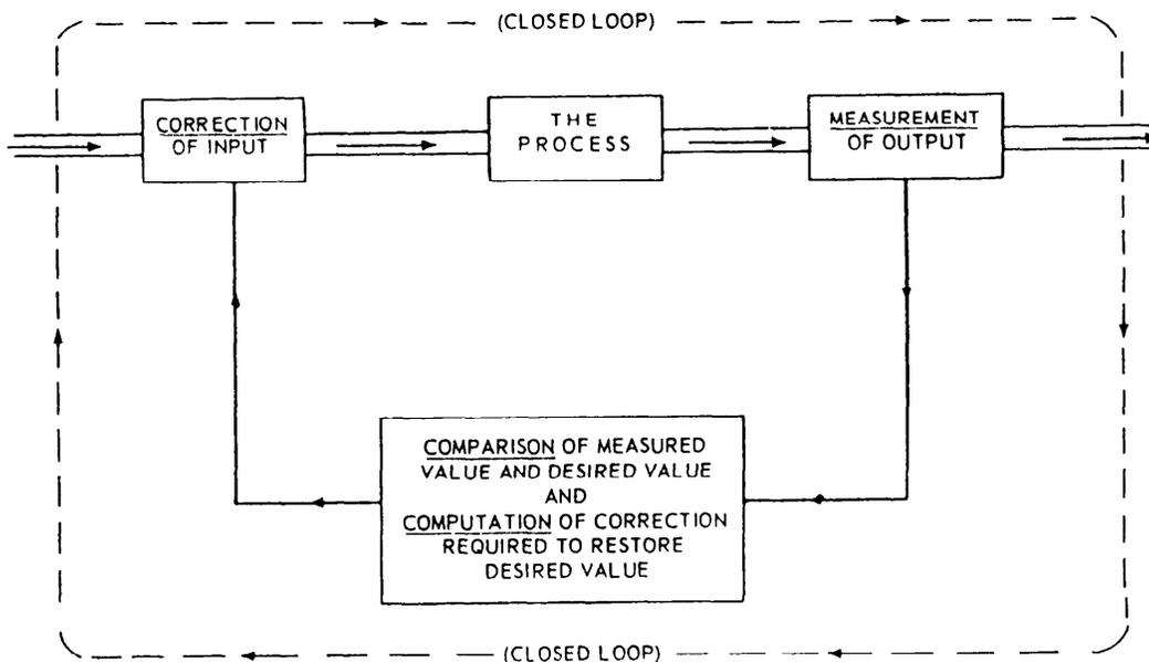
Figure 17-2.—Closed loop of control.
