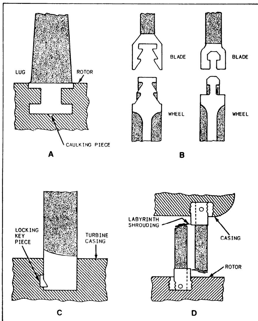
Figure 2-21.—Methods of securing turbine blades: A. Straight circumferential dovetail. B. Inverted circumferential dovetail. C. Side-locking key piece. D. Sawtooth serration.
