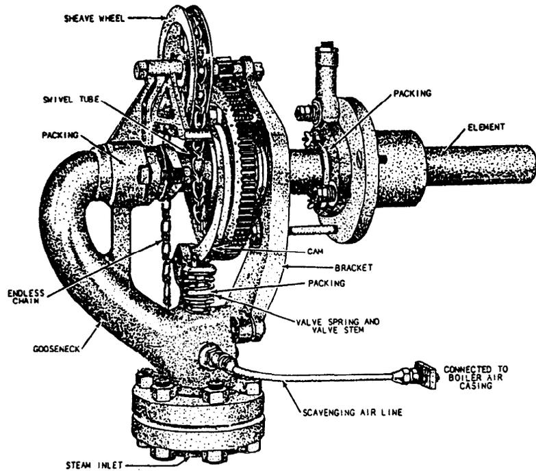
Figure 16-12.—External view of a rotary soot blower.
