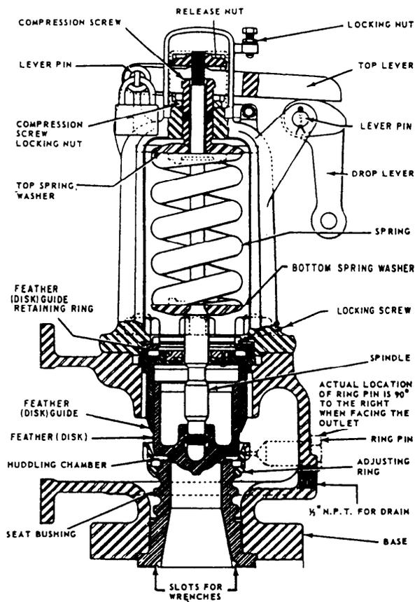
Figure 16-21.—Steam drum safety valve (huddling-chamber type).
