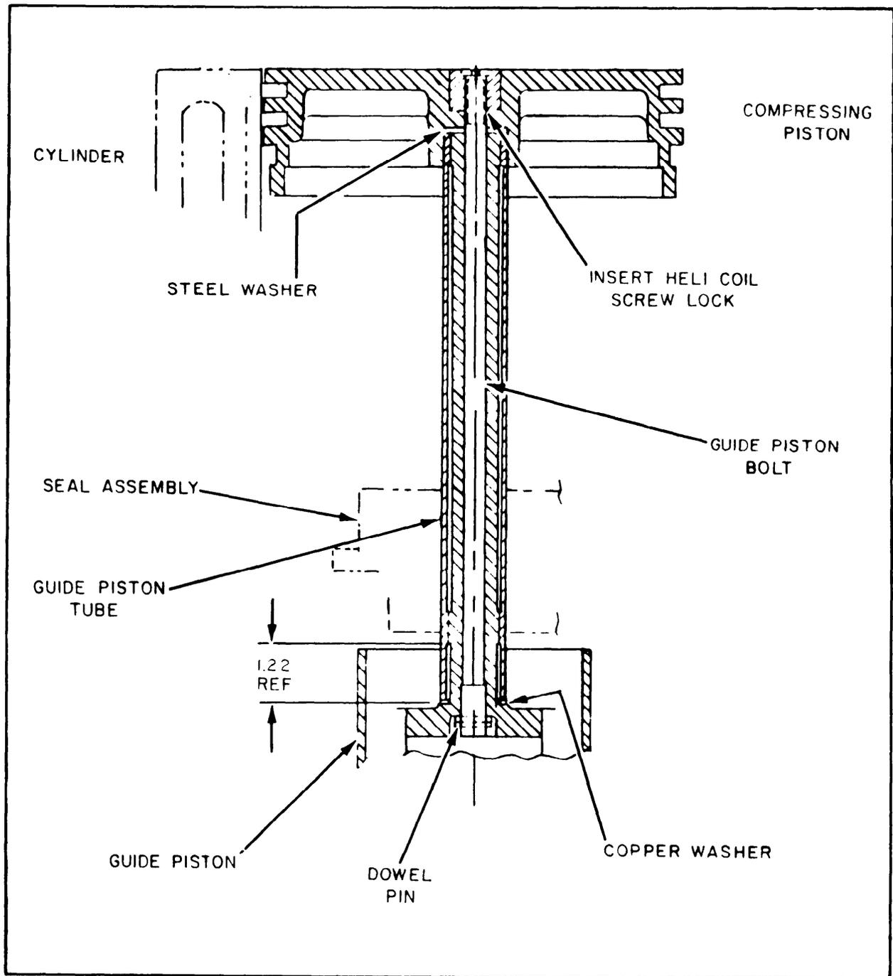
Figure 13-17.—Hollow-type piston assembly.
