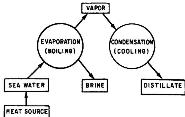
Figure 9-1.—Simplified diagram of shipboard distillation process.
