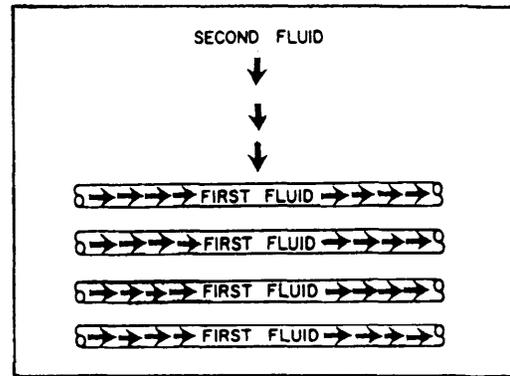
Figure 6-3.—Crossflow in a heat exchanger.
