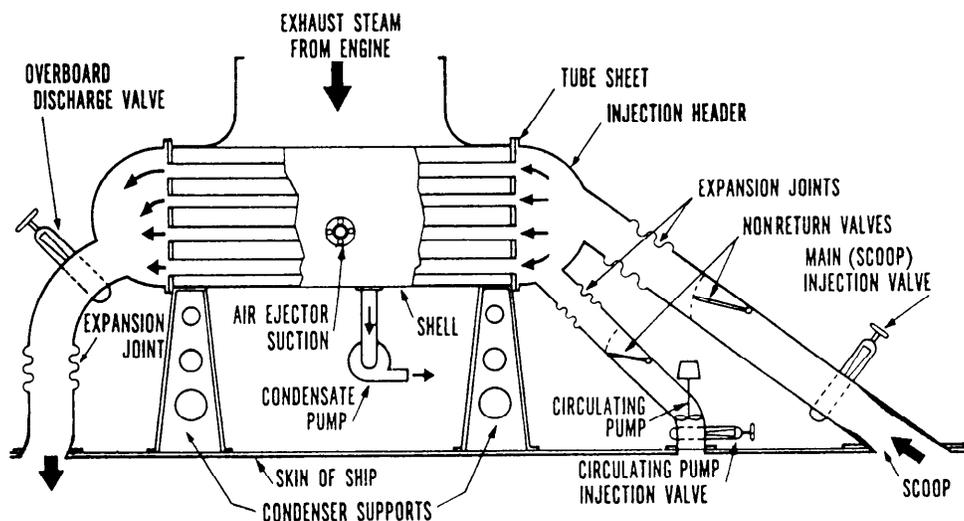
Figure 6-4.—Schematic arrangement of a main condensing system.
