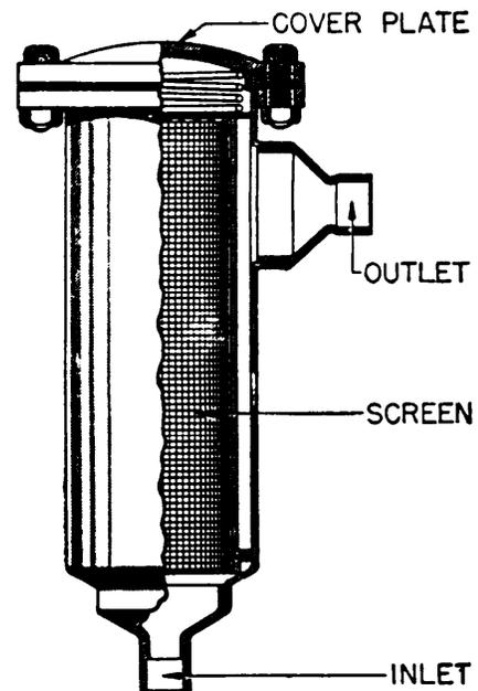
Figure 11-17.—Strainer of liquid refrigerant.
