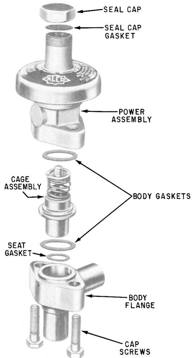
Figure 11-15.—Exploded view of a typical evaporator pressure regulating valve (EPR).
