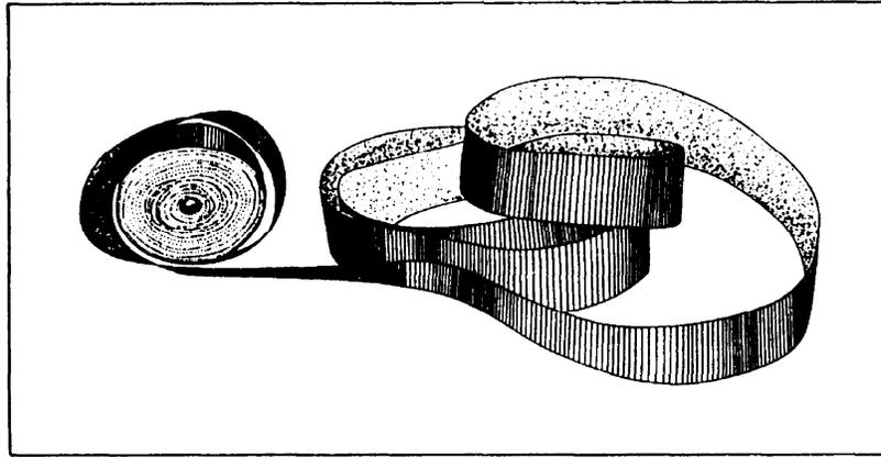
Figure 10-33.—Corrugated ribbon packing.
