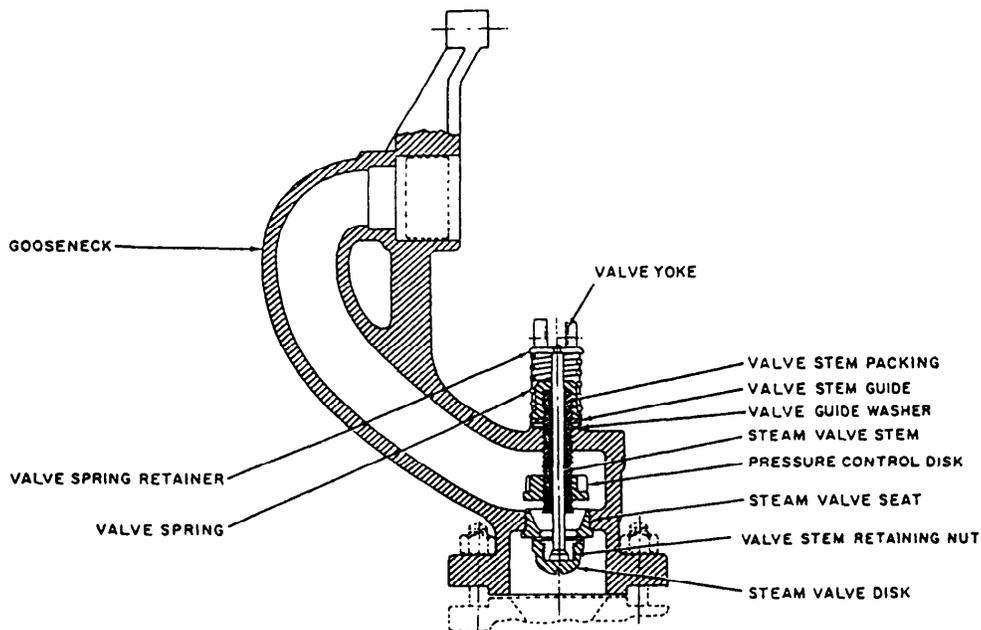
Figure 16-13.—Cross-sectional view of a rotary soot blower.
