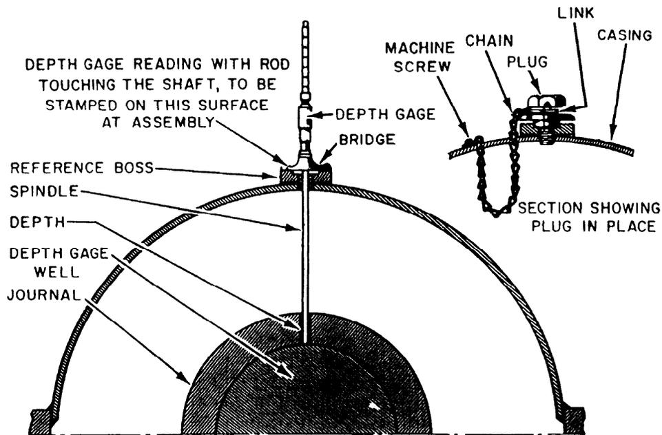
Figure 2-33.—Bearing wear micrometer depth gauge.
