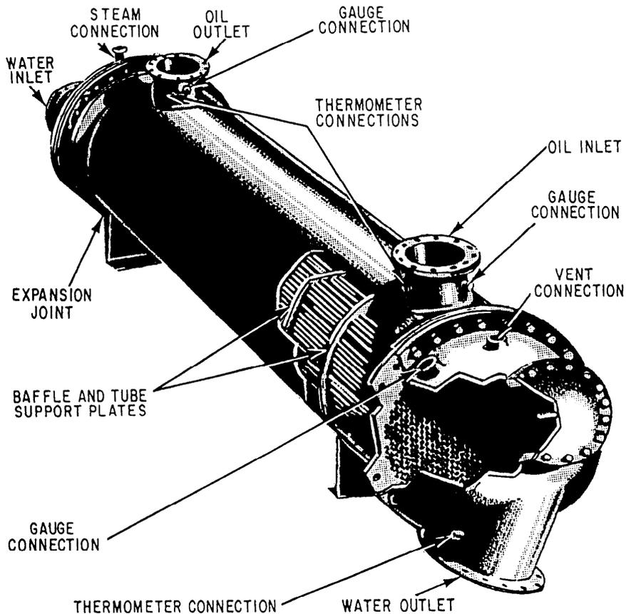
Figure 6-10.—Main lube oil cooler.
