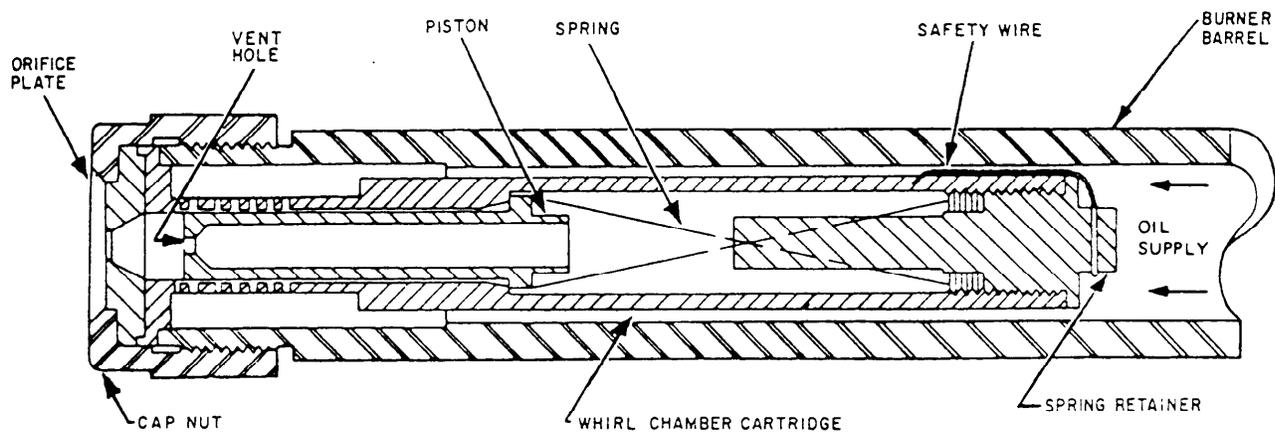
Figure 16-25.—Vented-plunger atomizer.
