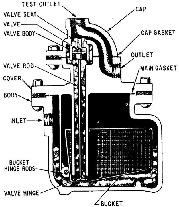
Figure 10-27.—Bucket-type steam trap.
