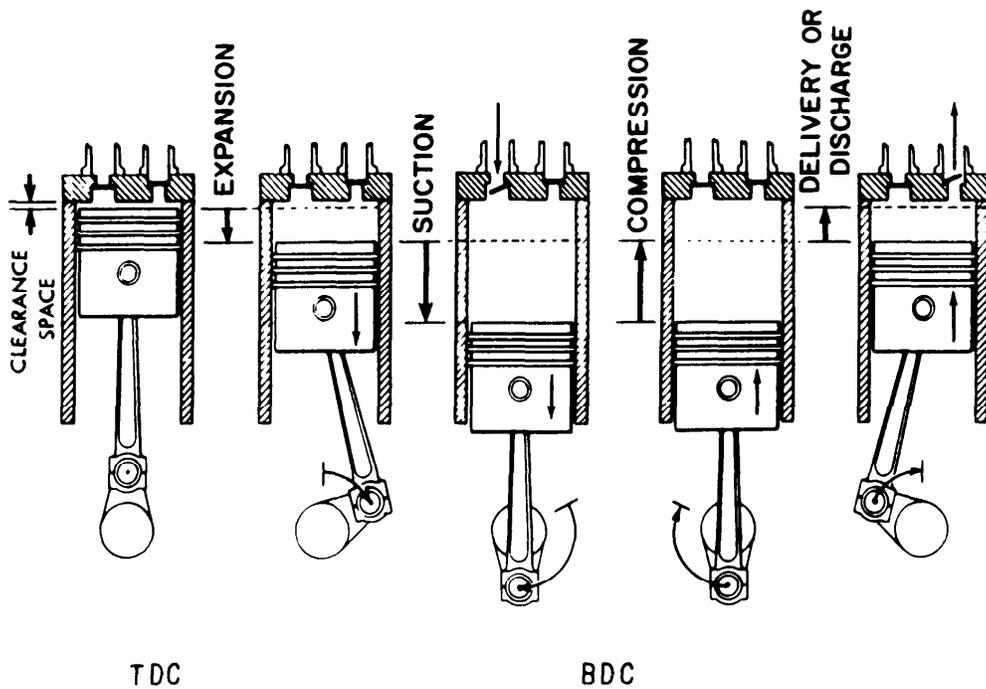
Figure 13-4.—The compression cycle.
