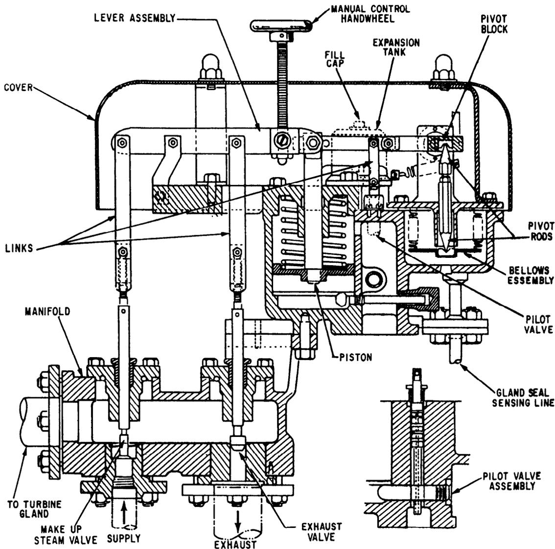
Figure 10-25.—Hydraulic steam seal regulator.
