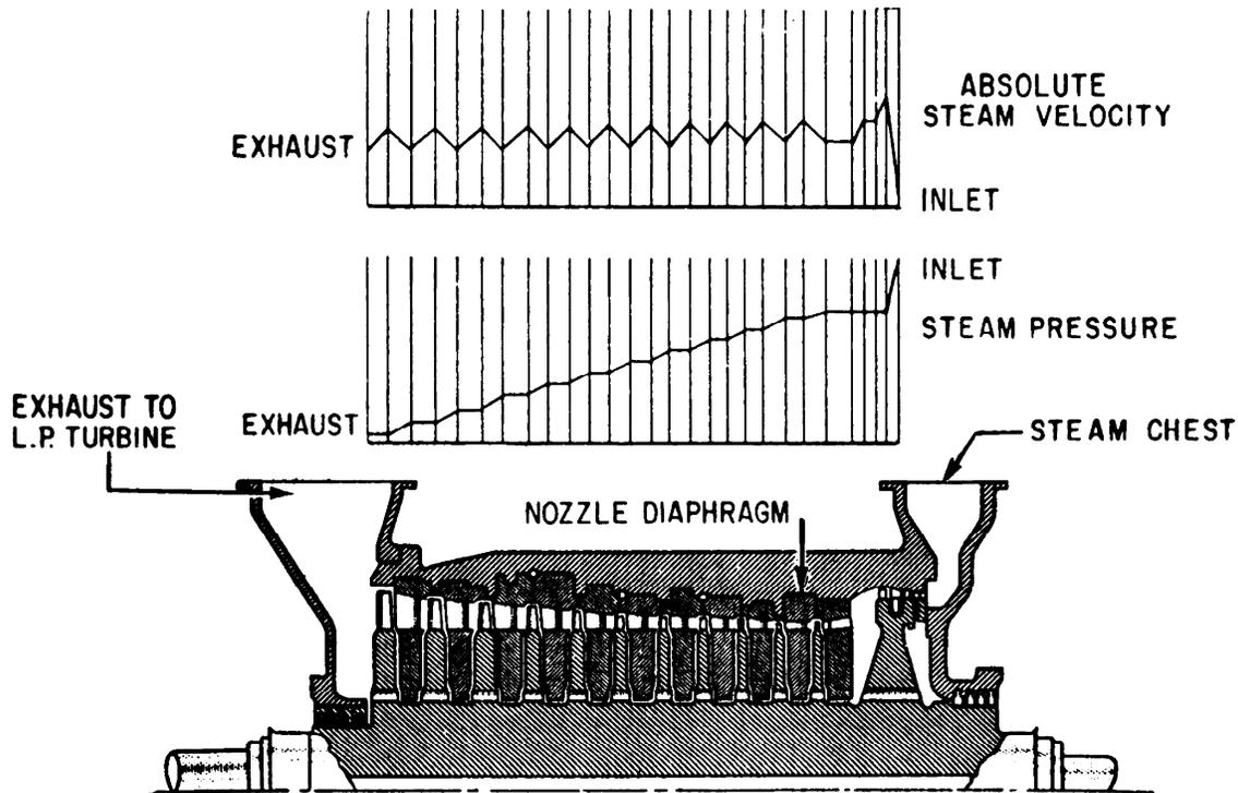
Figure 2-9.—Pressure-velocity-compounded impulse turbine showing velocity and pressure relationships.
