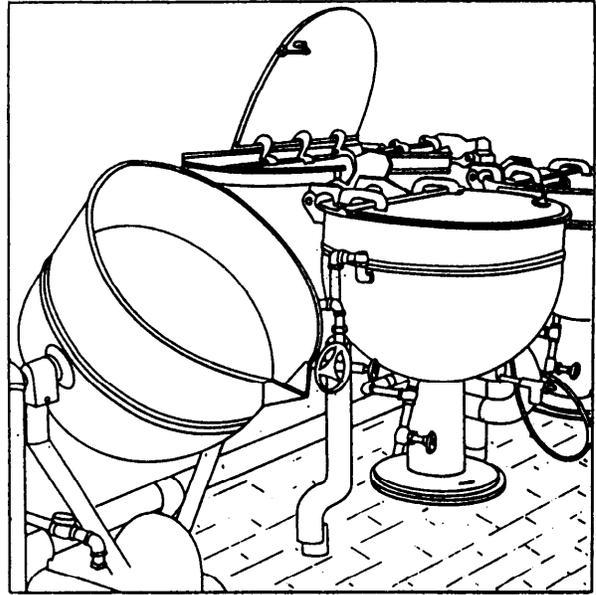
Figure 14-10.—Steam-jacketed kettles.
