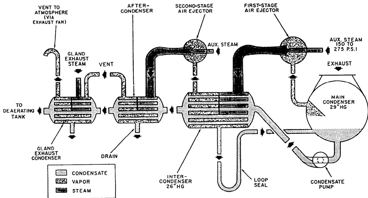
Figure 6-13.—Flow diagram of a two-stage air ejector.
