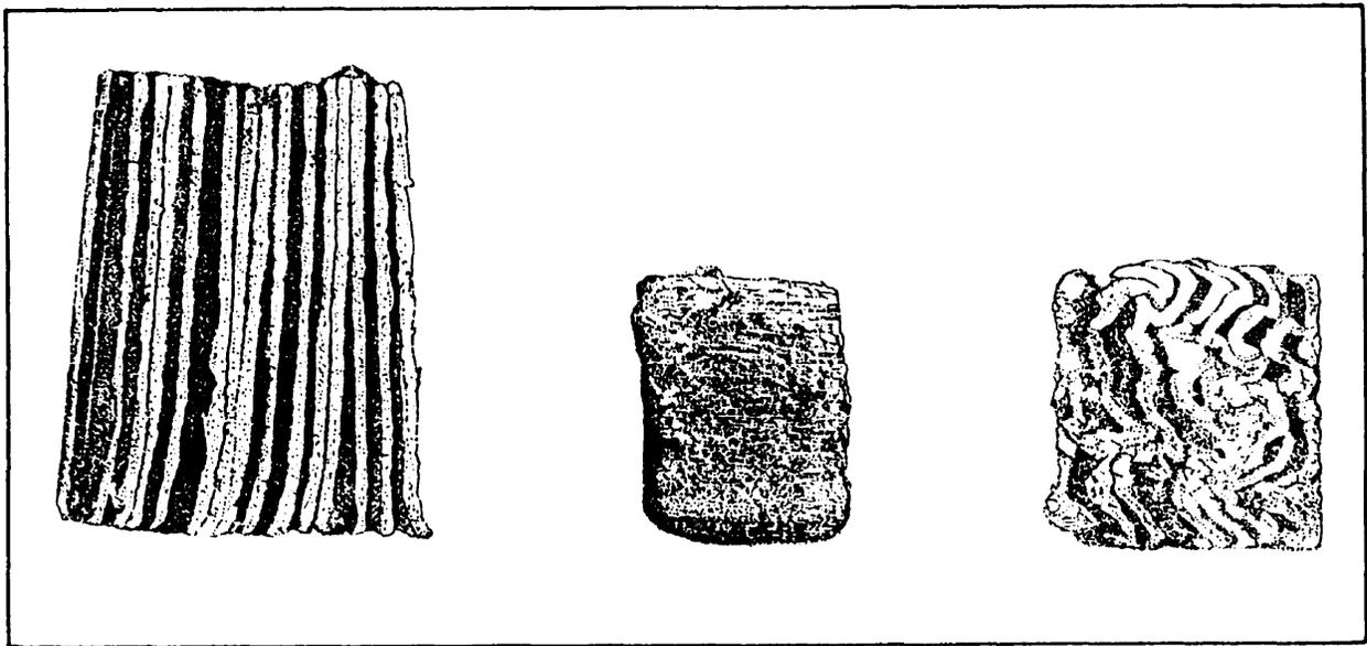
Figure 10-34.—Sectional views of corrugated ribbon packing after restructuring.
