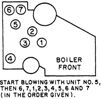
Figure 16-15.—Sequence of soot blowers on a single-furnace boiler.
