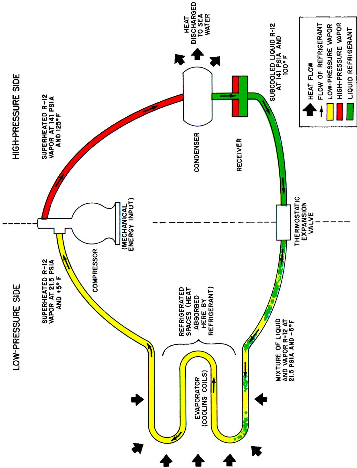
Figure 11-1.—Schematic representation of refrigeration cycle.
