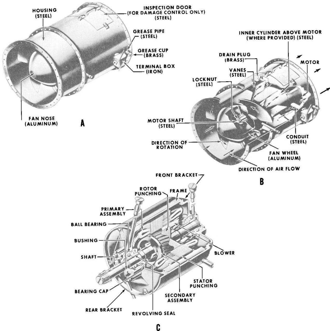
Figure 12-2.—Vane-axial ventilating fan: A. Exterior view. B. Cutaway view. C. Cutaway view of the fan motor.
