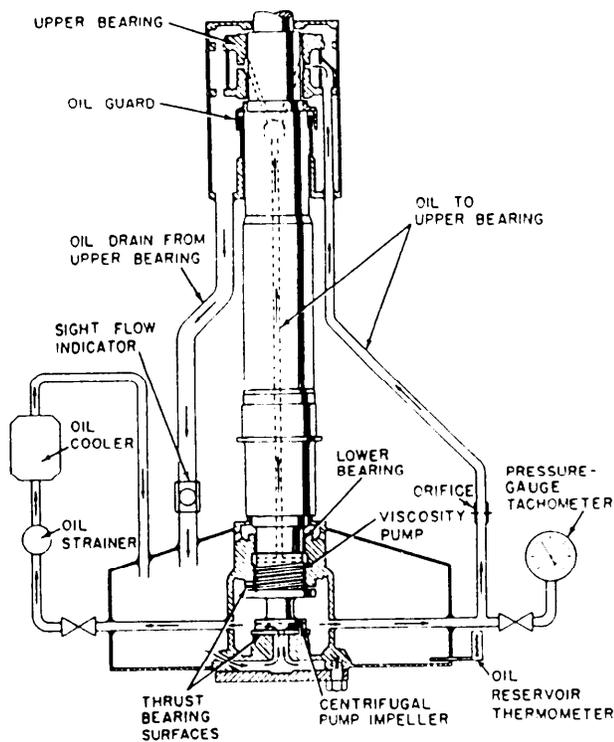
Figure 5-28.—Lubrication system for a vertical forced draft blower (oil supplied through hollow shaft and through external supply line).
