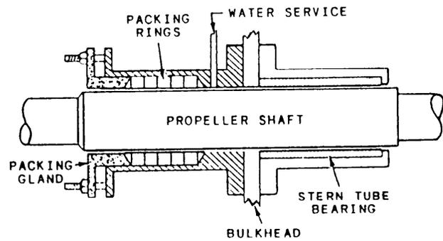
Figure 3-18.—Stern tube stuffing box and gland.
