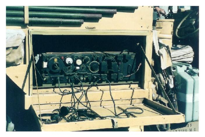
Wireless set No. 11, mounted in a 1½ ton Chevrolet truck. Note the right hand drive! Also note the headphones and straight key on the radio compartment door. There are also four 8½ foot poles mounted above the radio compartment. These were used to support the Windom antenna.
