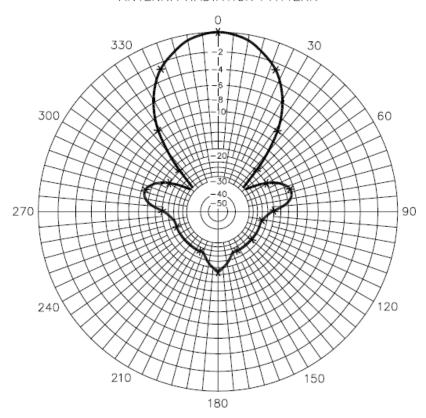
Note that this plot is only in <u>two</u> dimensions, and is usually specified in the direction of the azimuth. Your actual radiation pattern is <u>three</u> dimensional and far exceeds my ability to sketch!
