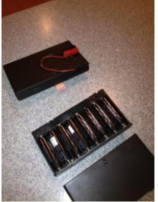
Battery clamshell used to power all the gear
