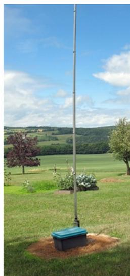
On the left is my 43' aluminum vertical antenna in my backyard. Below the antenna are 36 radials buried 1" to 2" in the ground. At the base of the antenna is a MFJ remote
