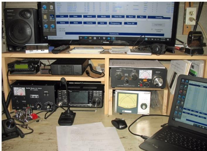
I have 3 complete stations on my desk. First is an Icom 7300. It feeds into a MFJ-962D tuner (used only for a SWR meter) to an Icom AH-4 remote tuner to a dipole antenna. Next is an Icom 7100 into an Ameritron ALS-600 solid state amp through a Daiwa SWR meter to a MFJ remote tuner at the base of my vertical antenna. My third station is an Icom 2300H transceiver for 2 meter FM.
