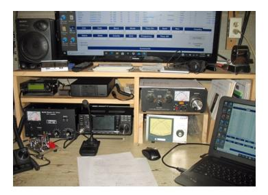
I have 3 complete stations on my desk. First is an Icom 7300. It feeds into a MFJ-962D tuner (used only for a SWR meter) to an Icom AH-4 remote
