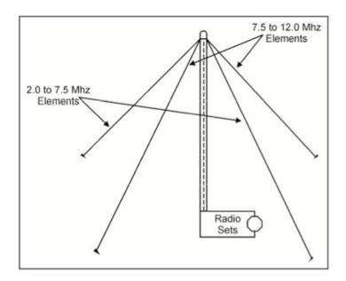
Note that I did <u>not</u> set the radio at the bottom of the mast. Instead we used 50 feet of low loss coax to feed the signal into the house. I could see no point in sitting in the RF pattern all day!
