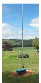
tuner in a weather resistant storage bin. In the bin are two heavy rocks under the tuner to prevent the wind from blowing it away.
