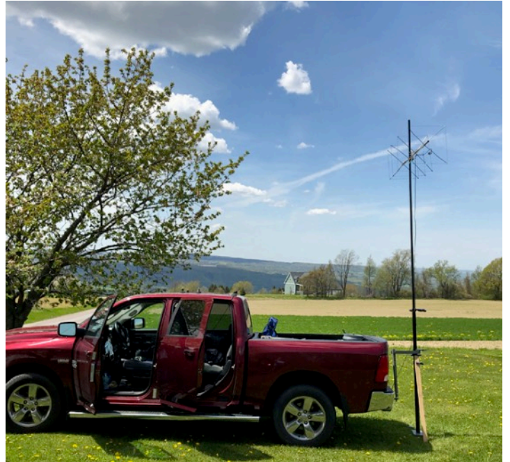
Gary KC2YTD used a 4 element quad antenna as part of his rover station.
