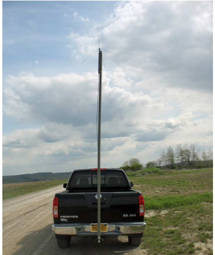
Harold N2FMS using a hitch mounted home-brew ground-plane antenna.
