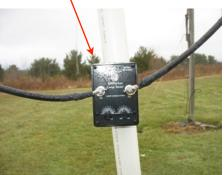
conductors soldered together at each end and soldered to ring terminals. It's a great antenna for hams with limited space or for portable operation. Even though it's close to the ground it has a low takeoff angle not like a dipole at the same height. It's also very easy to rotate, no rotor needed!
