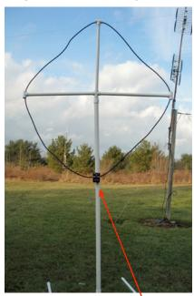
Patterson. The length of the loop must be more than 1/4 wavelength of the desired frequency or less than 1/8. If you use a 1/4 wavelength it will self resonate and cause many problems. The loop uses the magnetic portion of a radio wave. The loop is a very low noise antenna and has very deep nulls to null out interfering
