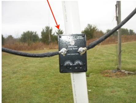
conductors soldered together at each end and soldered to ring terminals. It's a great antenna for hams with limited space or for portable operation. Even though it's close to the ground it has a low takeoff angle not like a dipole at the same height. It's also very easy to rotate, no rotor needed!
